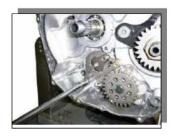
• Fit Oil Pump Gear and adopt snap ring into the groove on Oil Pump Shaft end.
