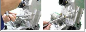
Adjust valve clearance with thickness gauge adopted at TDC position in the following procedures;
