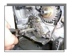
• Insert Shift Shaft CP with Special Tool; Oil Seal Guide adopted.
