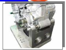
• Apply TB #1344 to Reverse Arm Lever threads (M6), and install along with Reverse Arm Spring.
