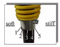
● Turn the adjusting sleeve on front shock absorber to the desired position with the wrench.
