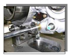
• Apply TB #1316 to Stopper Pin threads, and tighten to the specified tightening torque.
