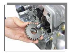
Fit Release Shaft along with Spring (Release) and Plate (Release) in position.
