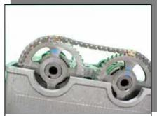
• Apply oil to Camshafts attaching portion, and install Camshaft (IN) and (EX) with Cam Sprocket marking and marking plate of Timing Chain aligned.
