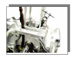
● Inspect the exhaust side and intake side chain guides. Wear/Damage – Replace.
