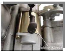
Remove the starter motor wire nut for disconnect the starter motor wire.
