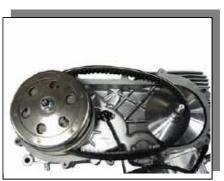
Reverse the Removal procedure to install the drive pulley, wash and nut.
