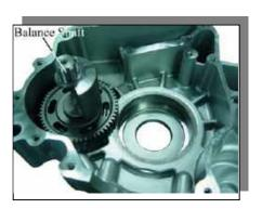
Clean off all gasket material from the crankcase mating surfaces.
