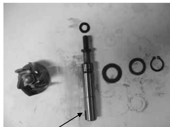
Water pump shaft
