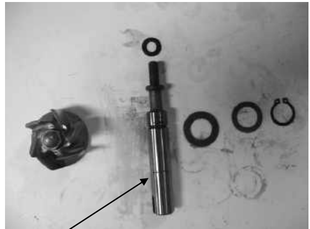
Water pump shaft
