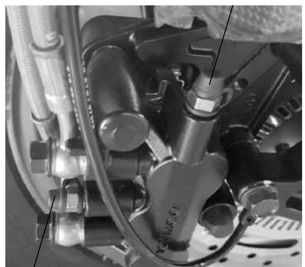
Secondary front brake tube bleed valve
