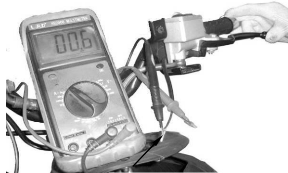
Stop Switch Wire
