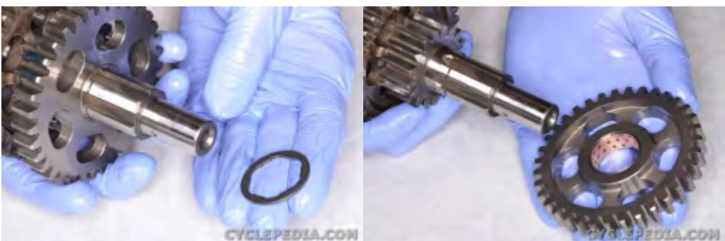
Remove the washer and low drive gear.
