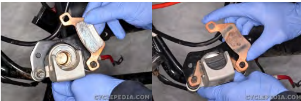
Install the brake pads.
