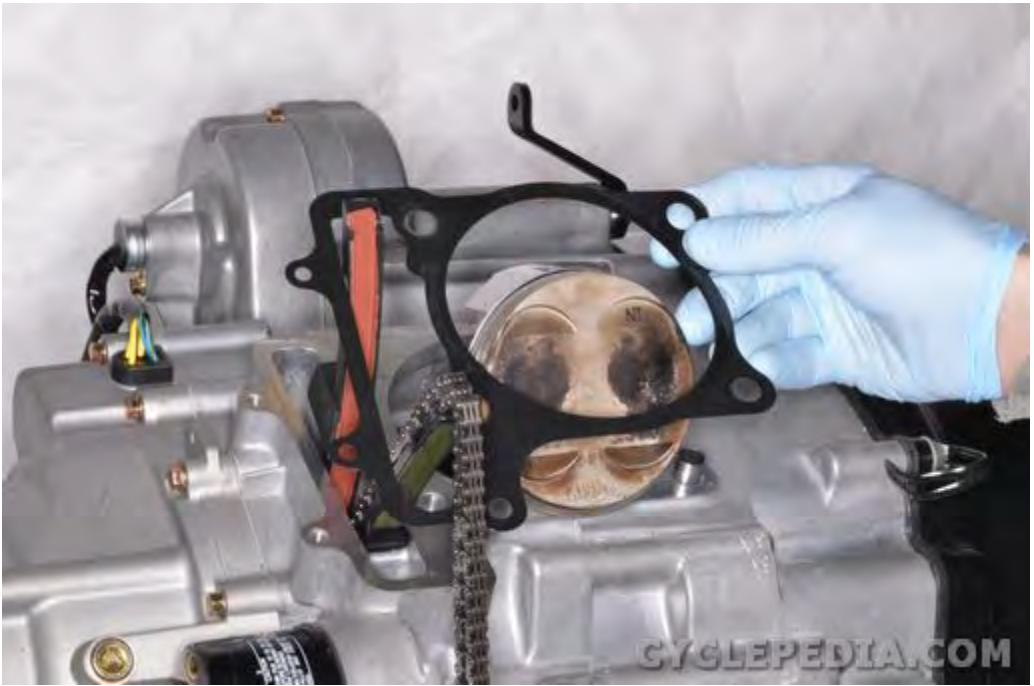
Lift off the base gasket.
