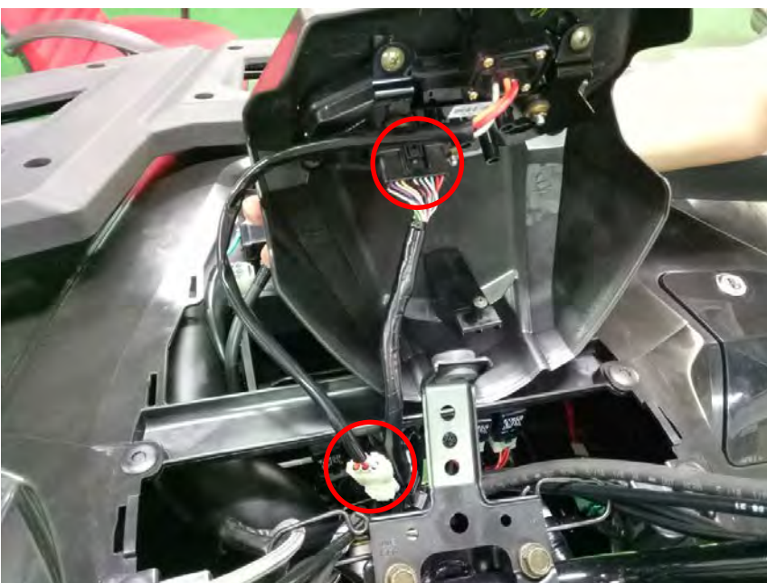
Plug the connector into the back of the instrument display.
