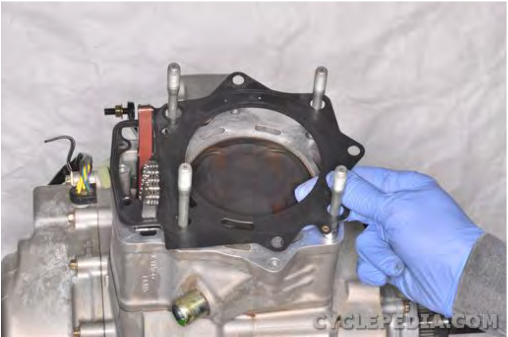
Remove the cylinder head gasket.
