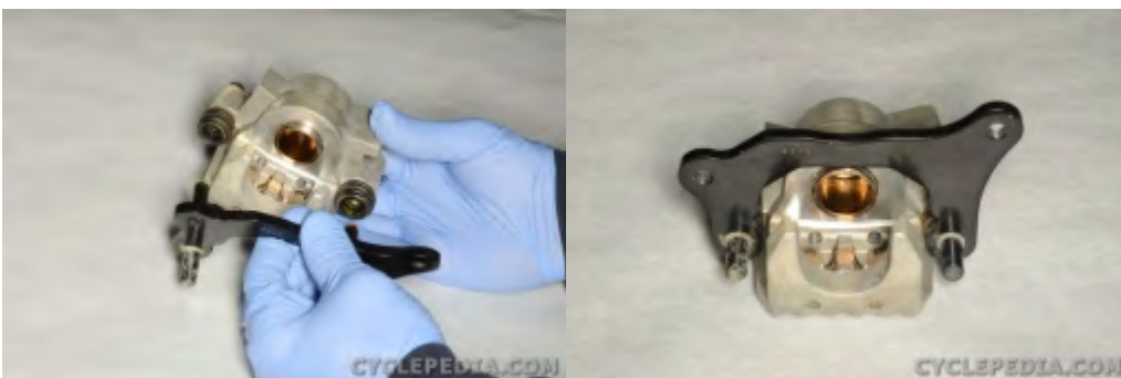
Apply silicone grease to the caliper bracket pins. Install the caliper bracket.
