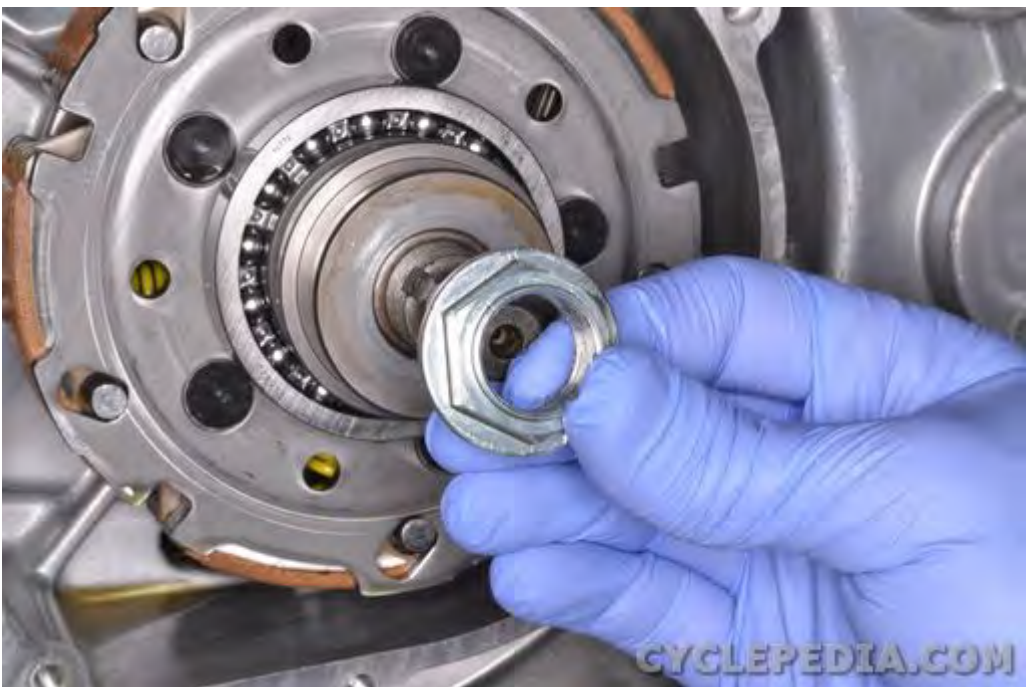
Thread on a new clutch lock nut.
