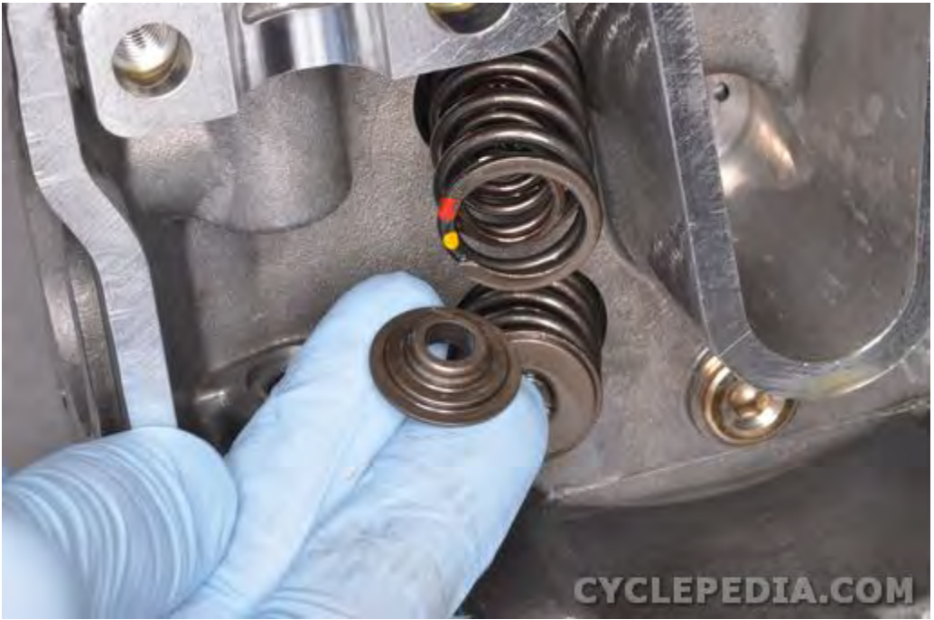
Remove the spring retainers.
