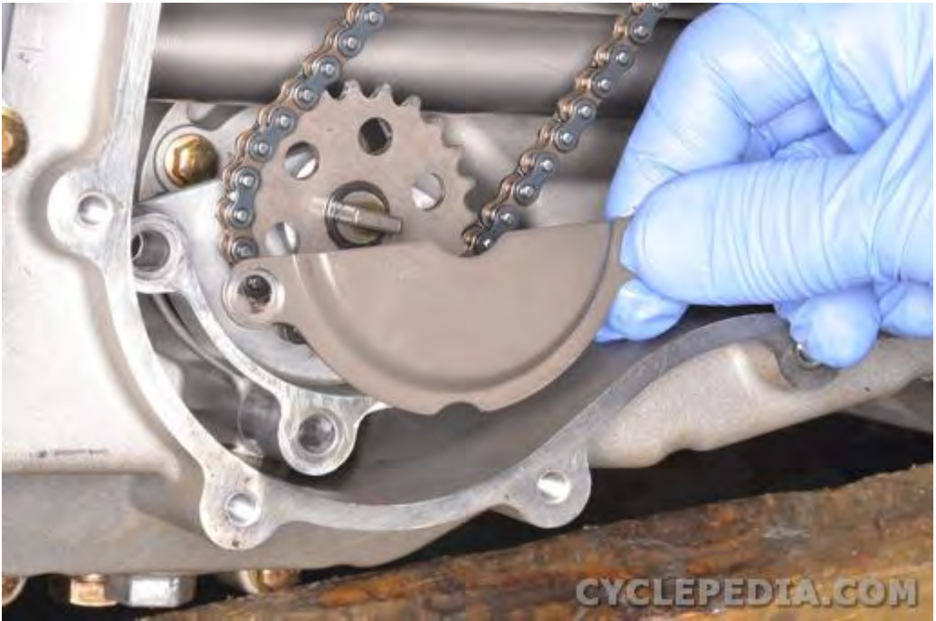
Remove the oil pump cover.
