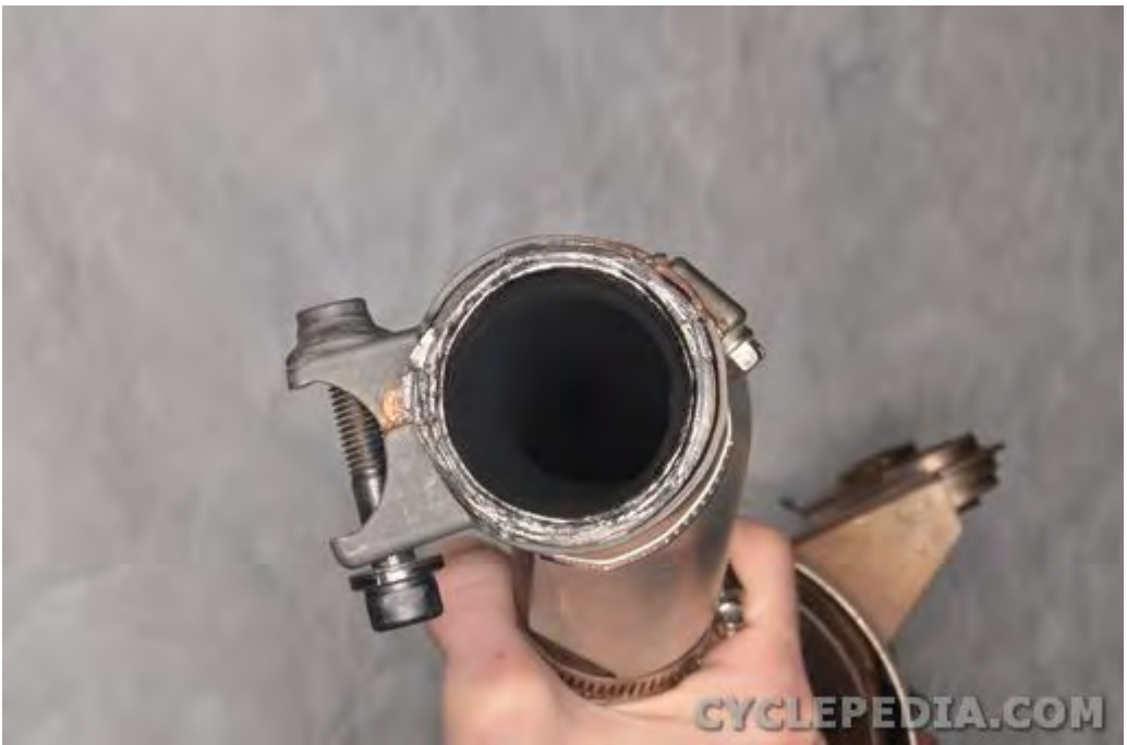
Remove the exhaust pipe gasket and discard it.
