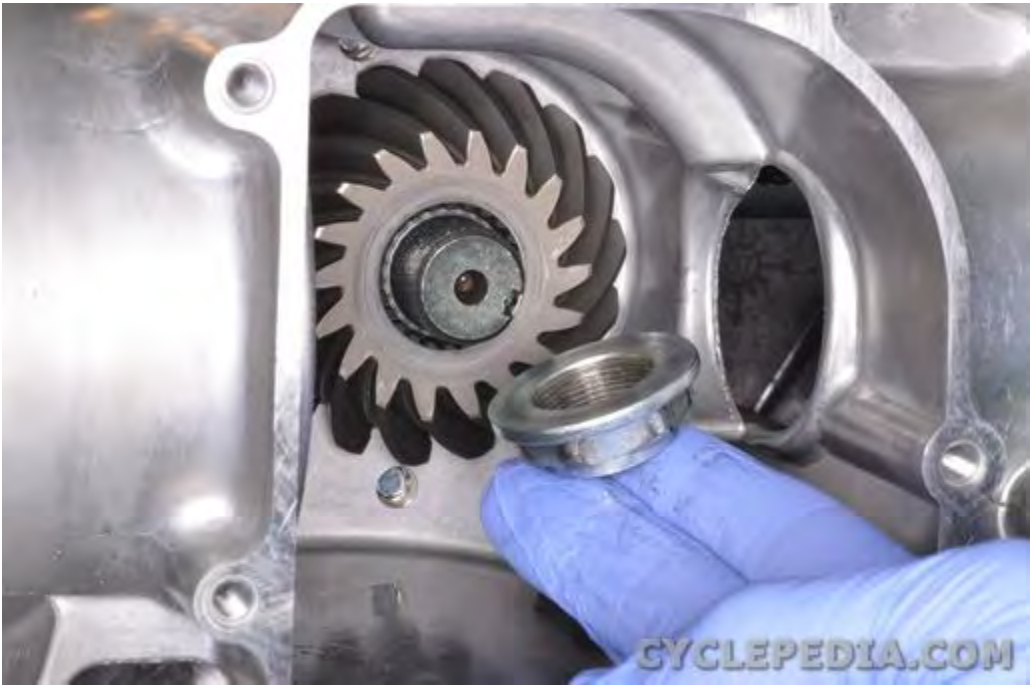
Remove the drive bevel gear nut.
