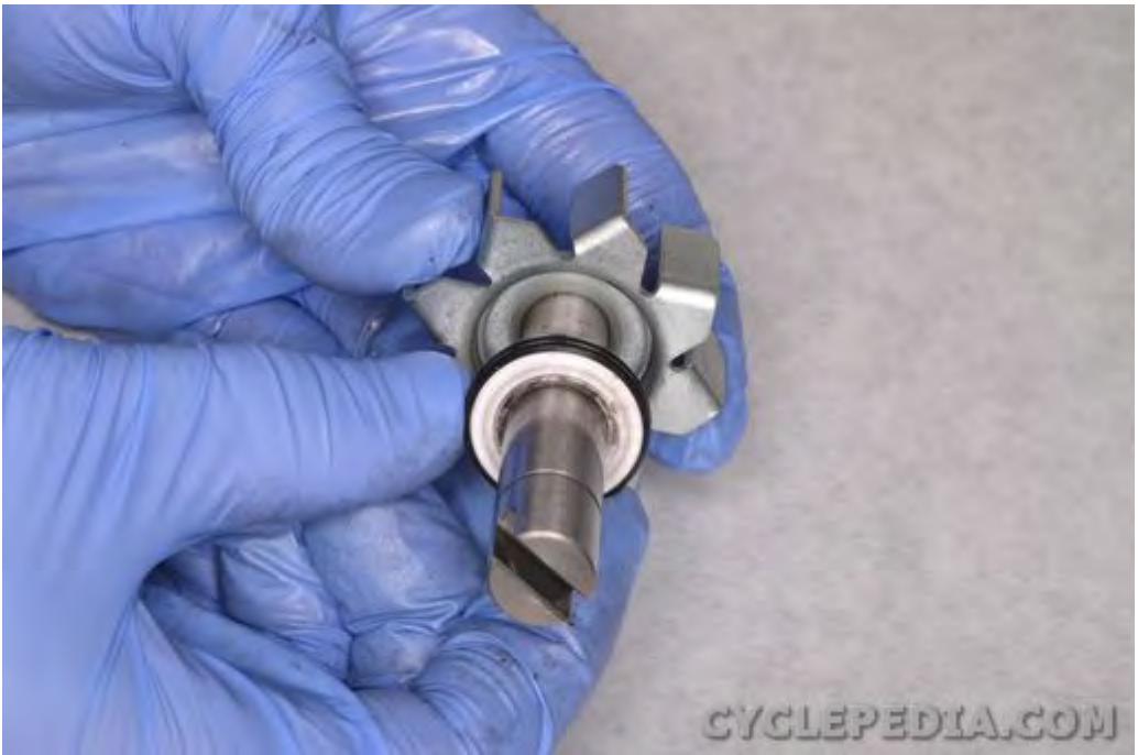
Remove the outer part of the mechanical seal.
