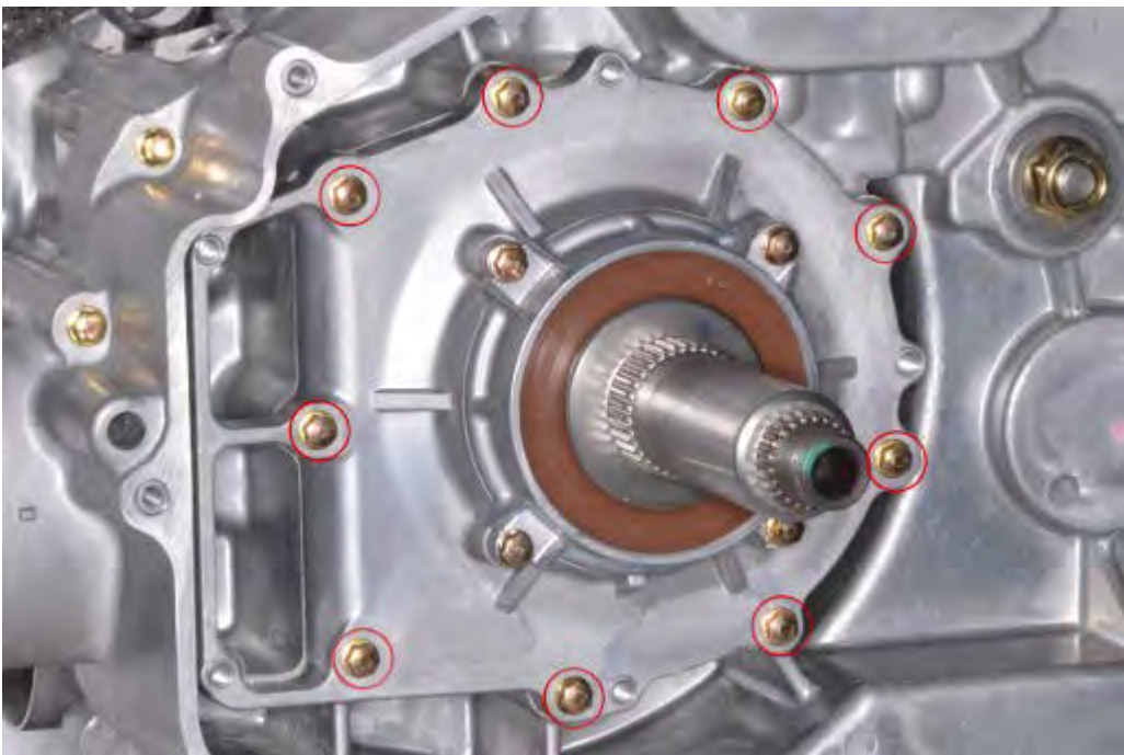
Loosen the 9 clutch cover bolts a little bit at a time and in a crisscross pattern.
