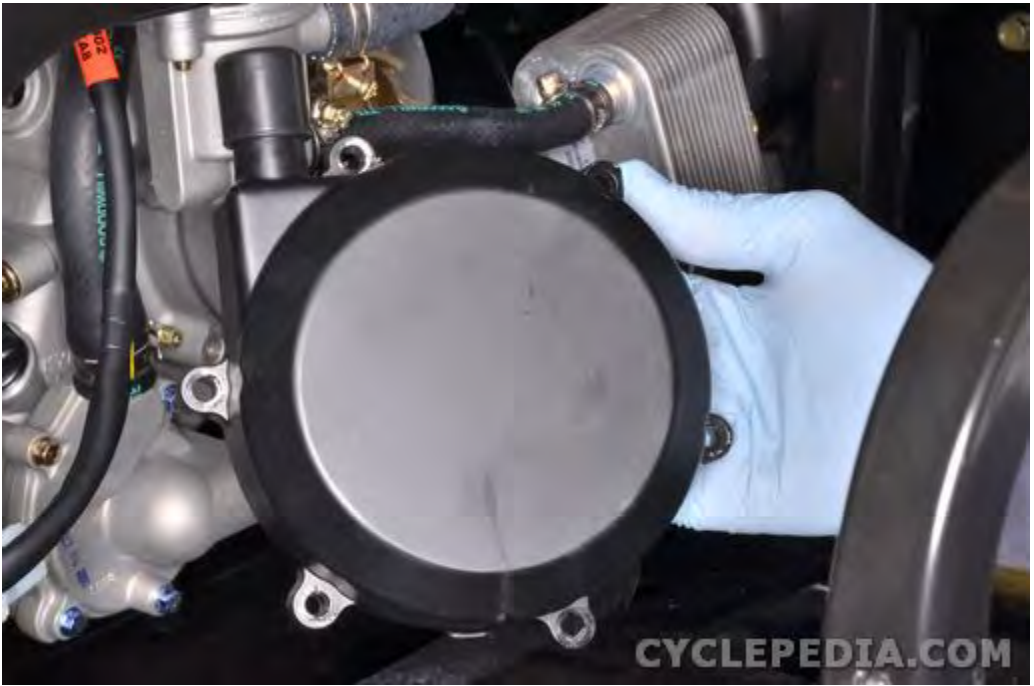
Remove the recoil starter cover.
