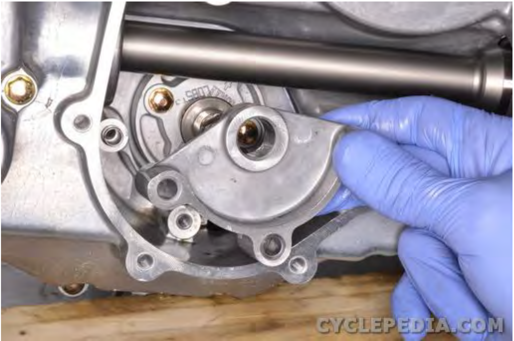
Fit the oil pump shaft holder into place.
