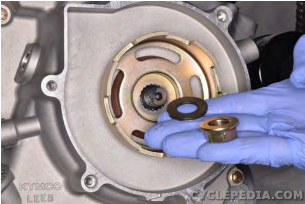
Remove the recoil starter nut and washer.
