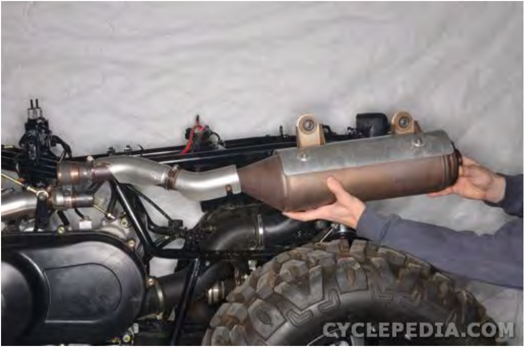
Slide the muffler back and free it from the header pipe.
