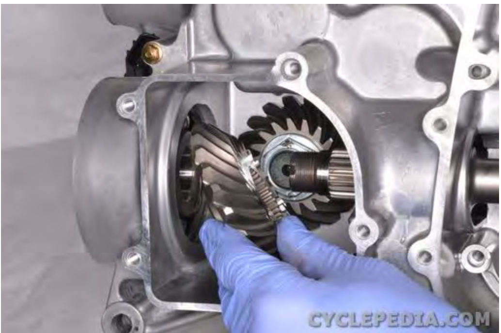
Guide the output shaft through the driven bevel gear and shim.
