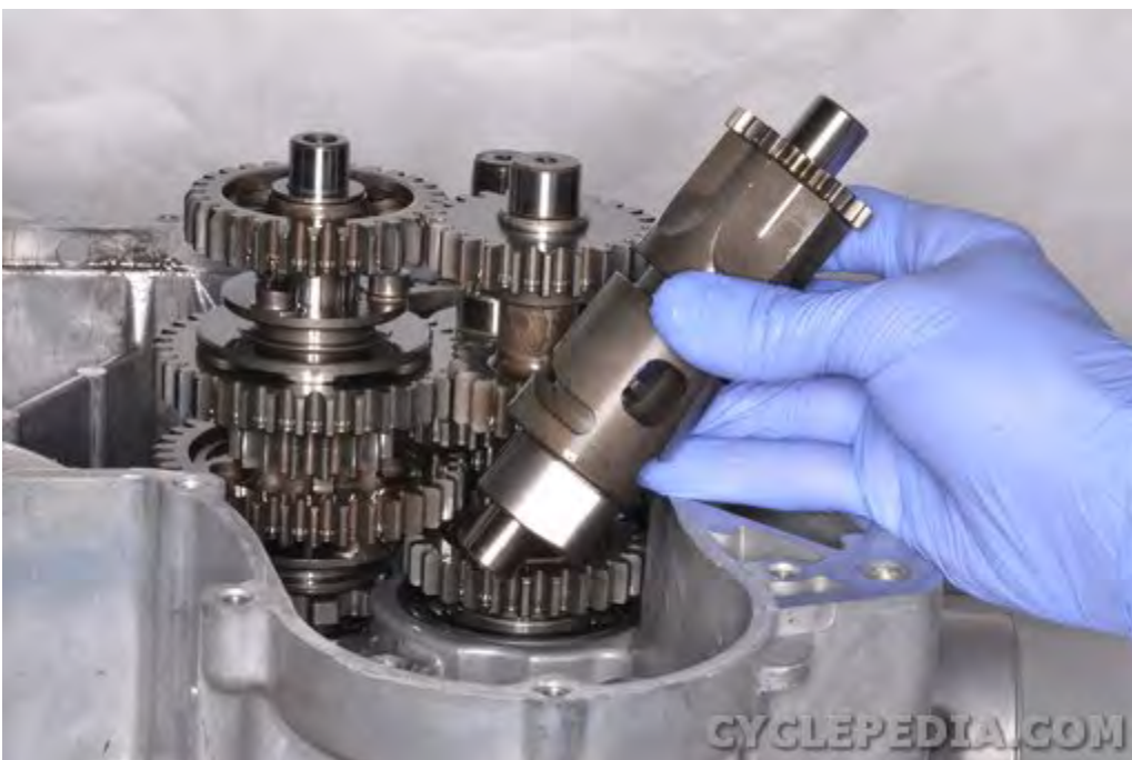
Apply clean engine oil to the shift cam and install it.
