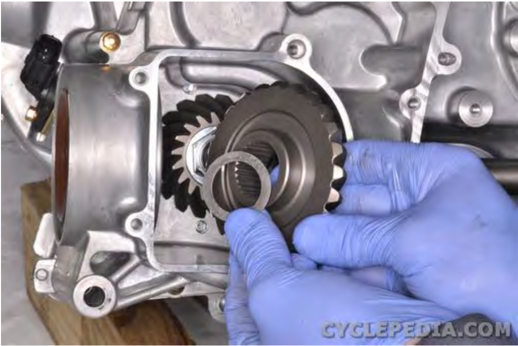
Remove the driven bevel gear and shim.
