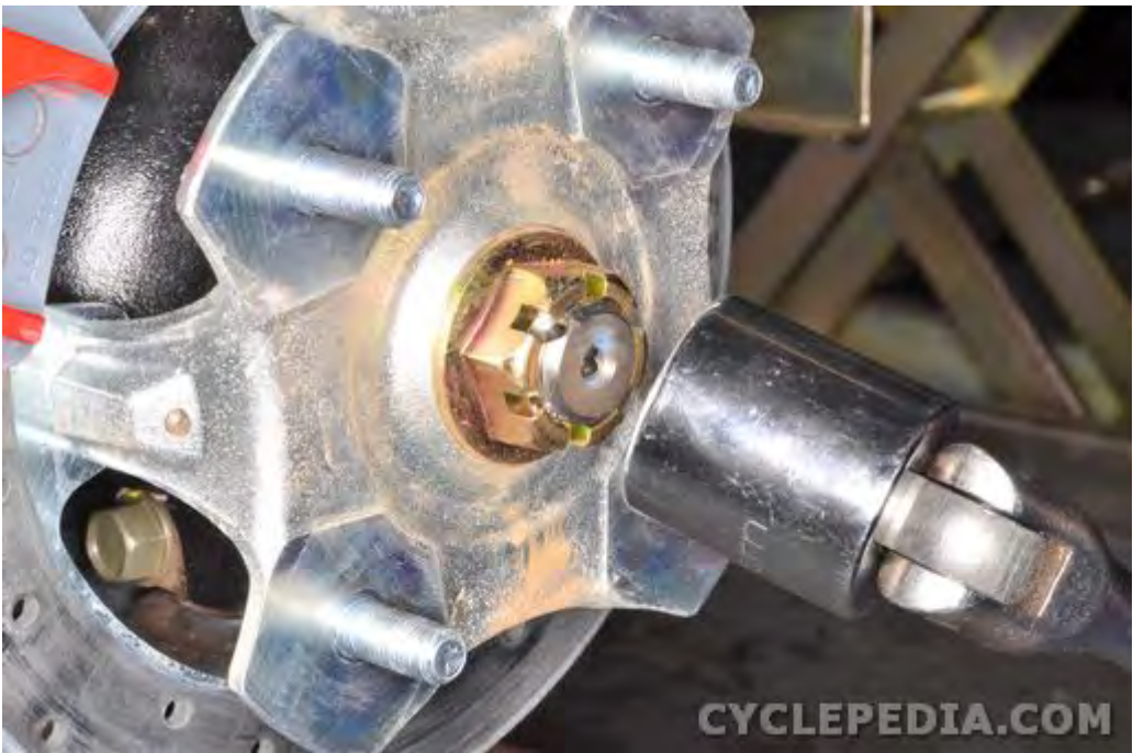
Apply the front brakes and tighten the axle nut to specification with a 30 mm socket.
