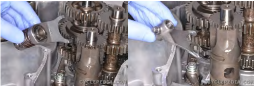
Remove the upper and lower shift forks.
