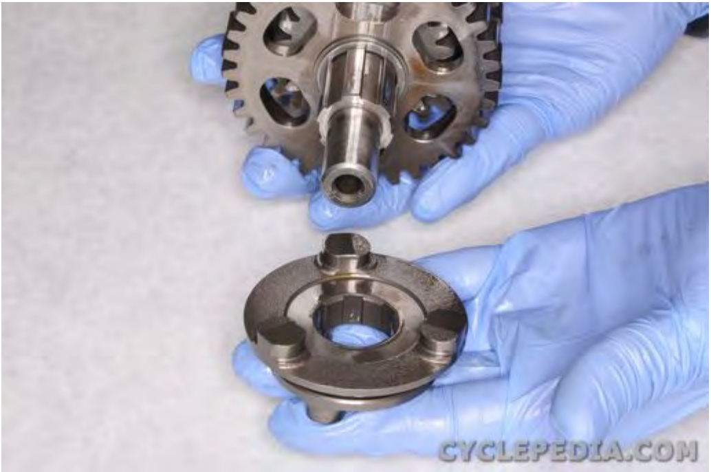
Remove the high/low gear shifter.
