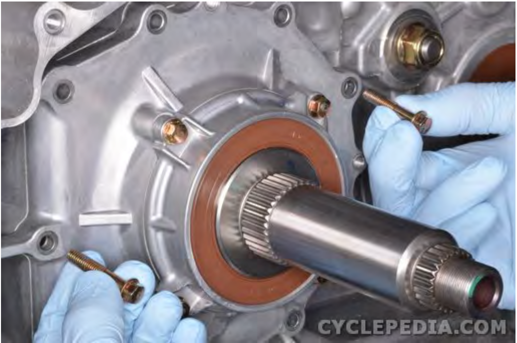
Remove the clutch cover bolts.
