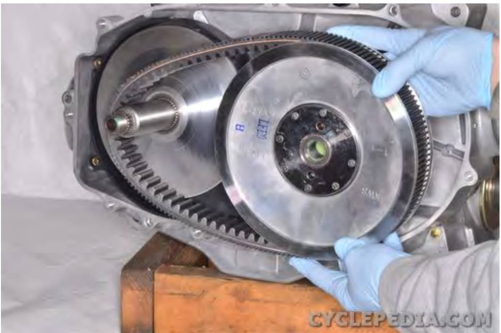
Remove the driven pulley and CVT belt.
