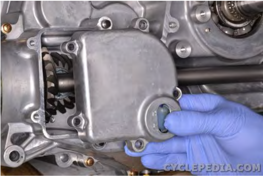
Remove the bevel gear cover.
