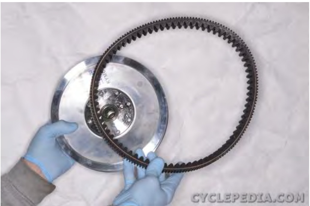
Remove the drive belt from the driven pulley.
