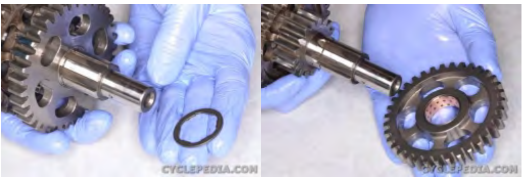
Remove the washer and low drive gear.
