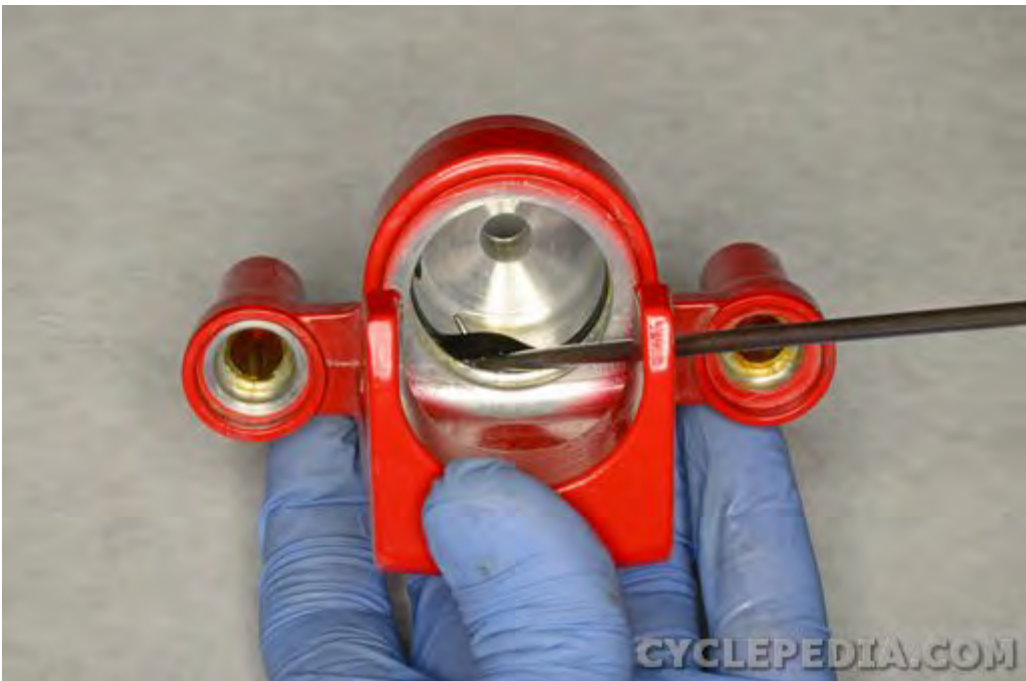
Use a mechanics pick to remove the piston fluid seal from the caliper bore and discard.
