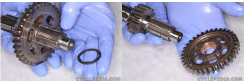
Remove the washer and reverse drive gear.
