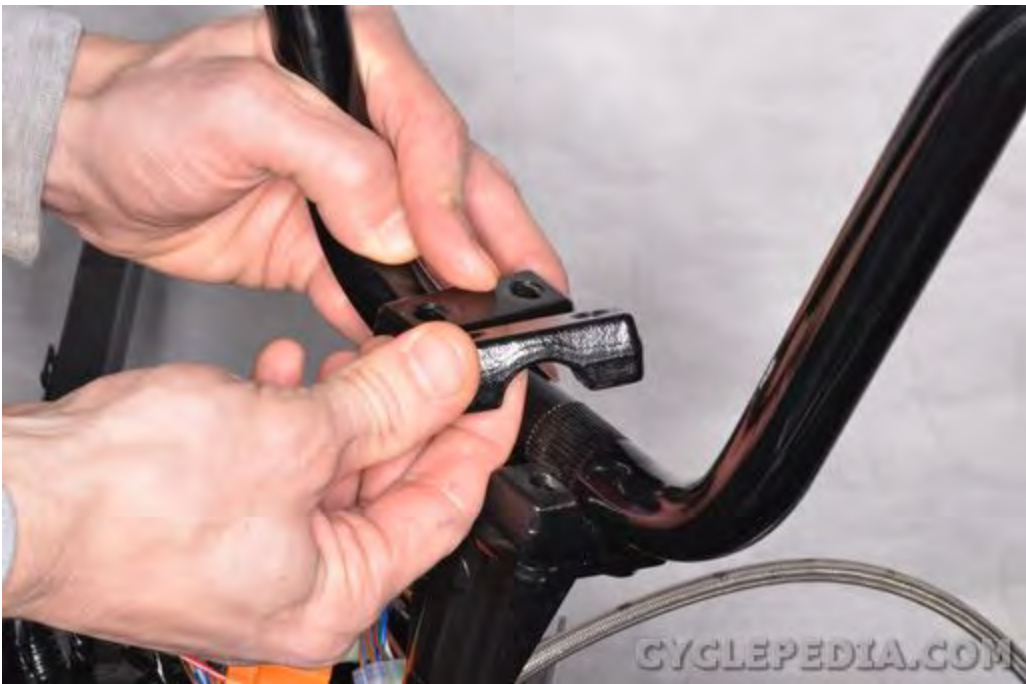
Lift off the handlebar clamps.
