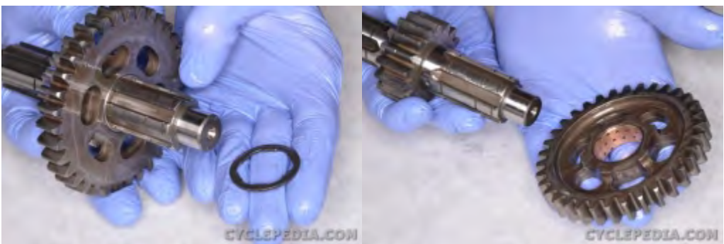
Remove the washer and reverse drive gear.
