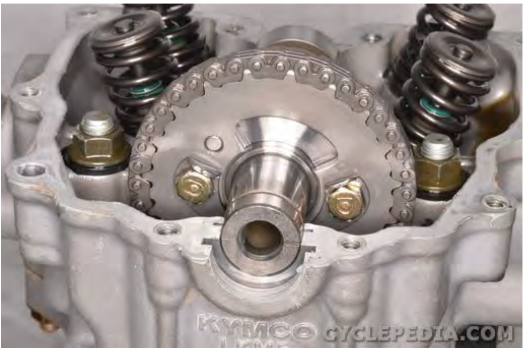
Remove the cam chain tensioner and gasket.
