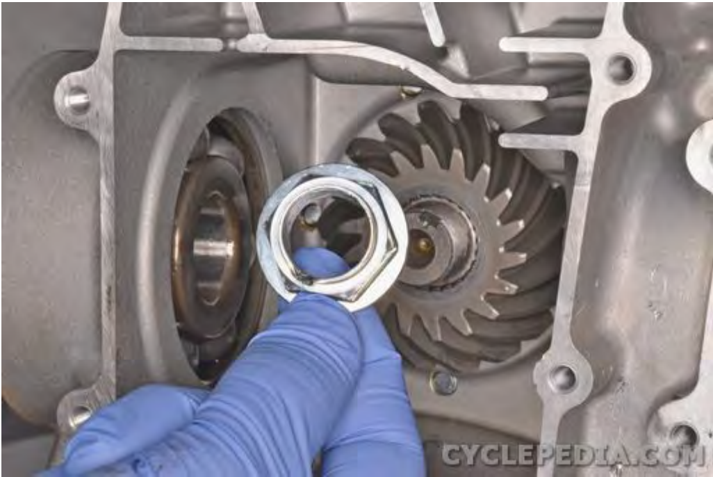
Remove the drive bevel gear nut.
