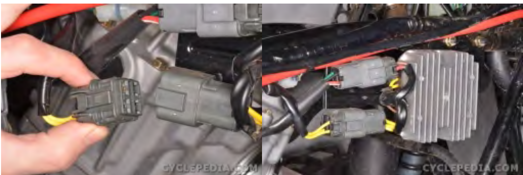
Plug in the 4-pin stator connector.
