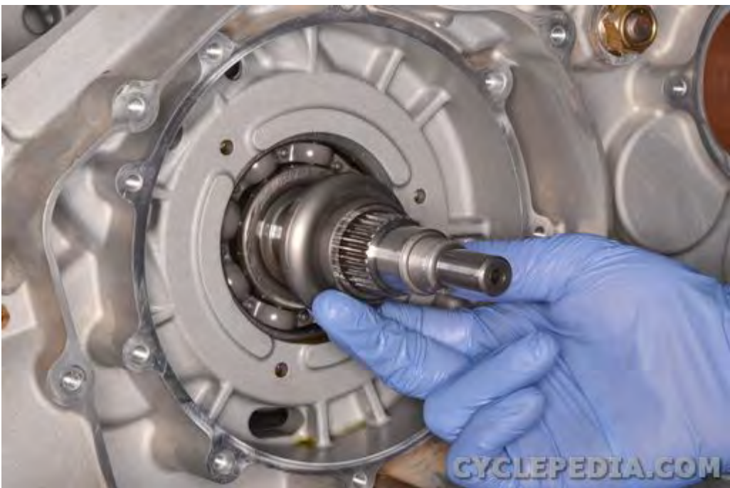
Slide off the inner clutch collar.
