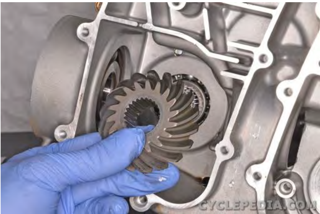
Slide off the drive bevel gear.
