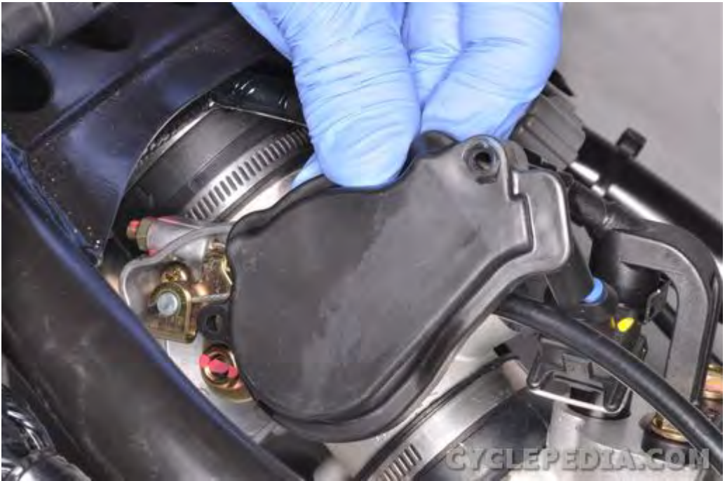
Remove the throttle drum cover.
