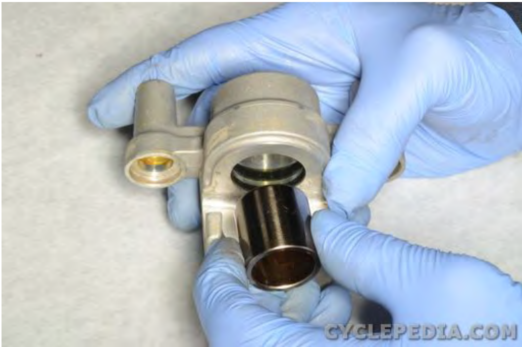
Remove the caliper piston by hand.
