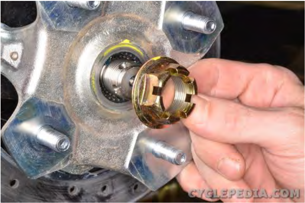
Thread on the wheel hub nut.
