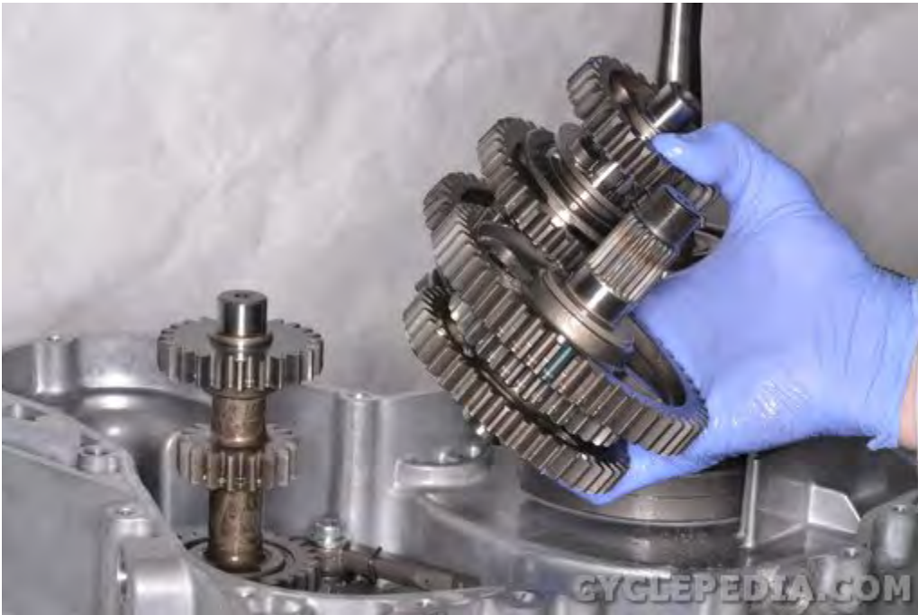
Install the transmission shafts together into the crankcase.
