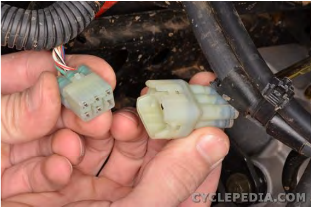
Plug in the gear position switch connector.
