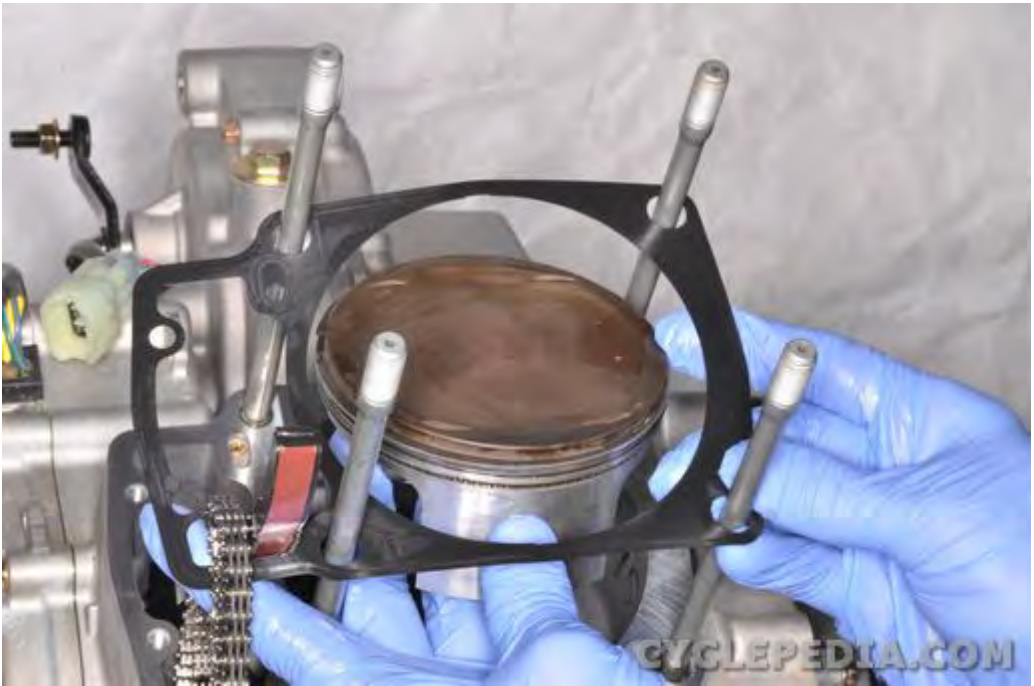
Lift off the base gasket.
