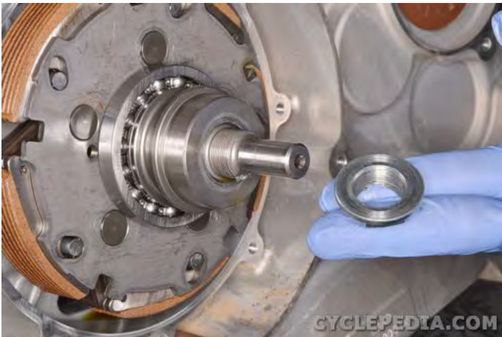
Thread on a new clutch lock nut.
