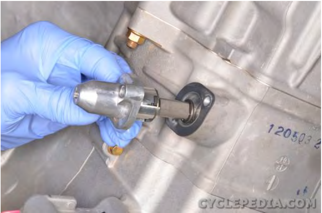
Remove the cam chain tensioner and gasket.
