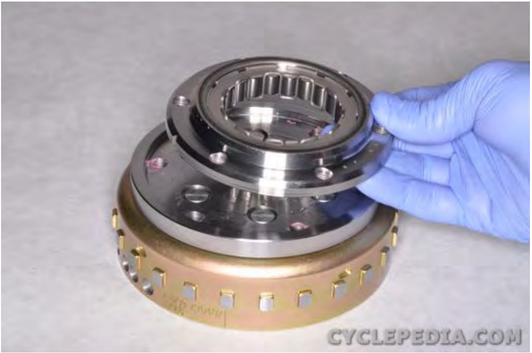
Remove the starter clutch and mounting plate from the back of the flywheel.
