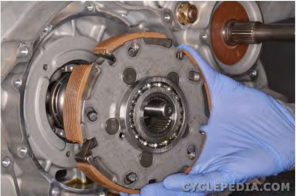
Slide the clutch onto the crankshaft. Be sure to align the splines.
