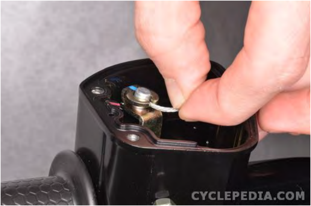
Free the end of throttle cable from the throttle lever.
