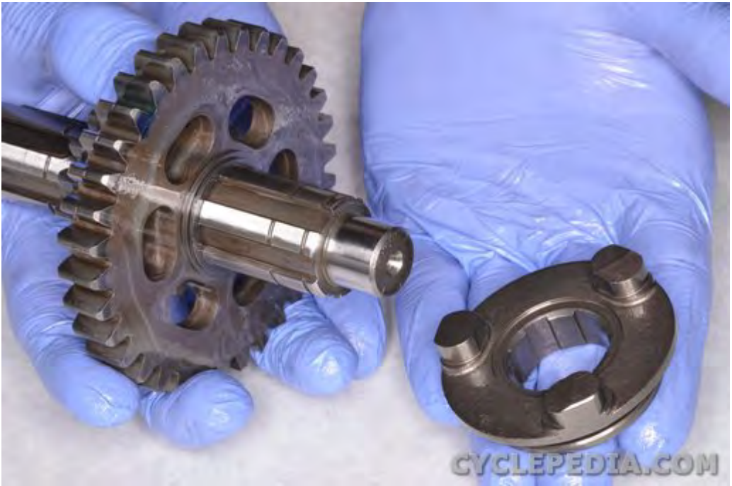
Remove the reverse gear shifter.
