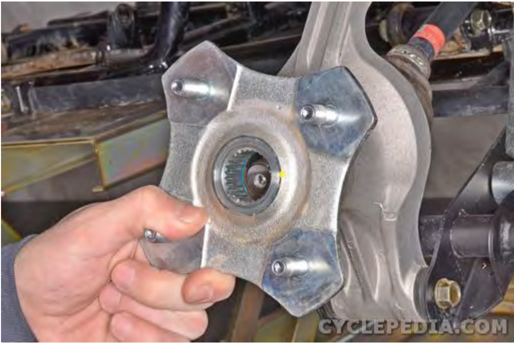
Slide on the wheel hub assembly.
