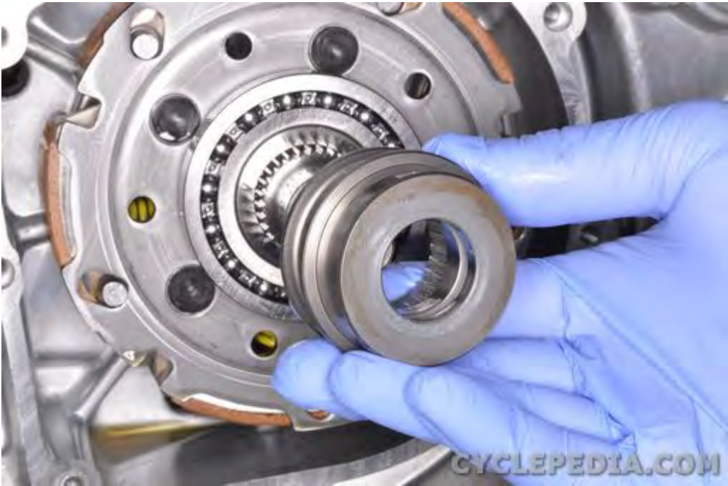
Slide off the outer clutch collar.
