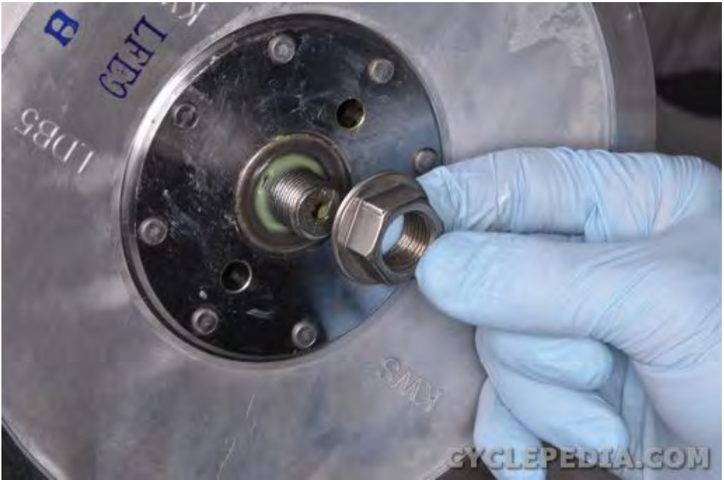
Remove the driven pulley nut.
