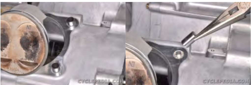
Remove the two dowel pins.
