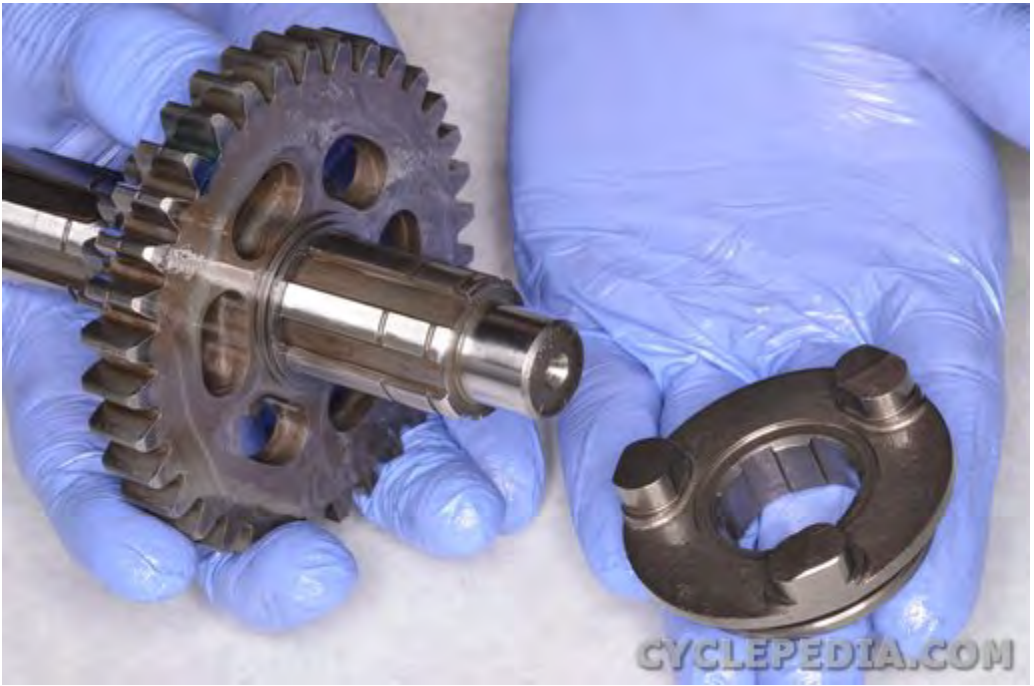
Remove the reverse gear shifter.
