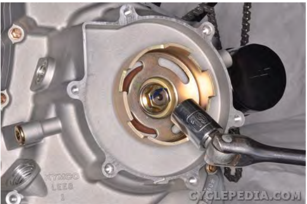
Turn the crankshaft clockwise with a socket.
