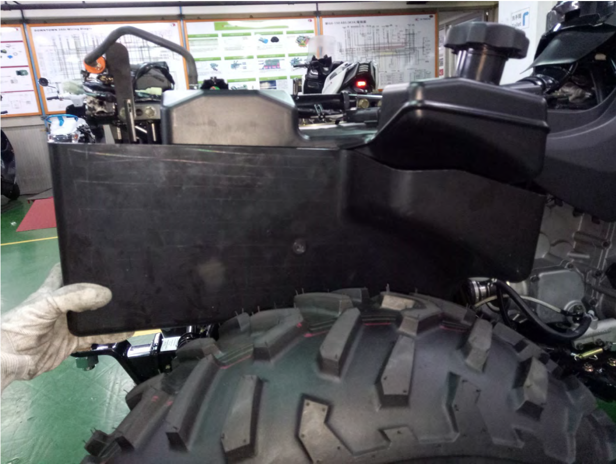
Remove the fuel tank protector cover.
