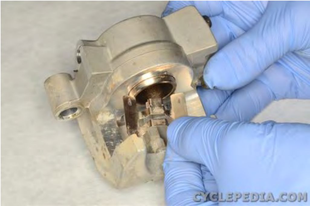
Install the brake pad spring.
