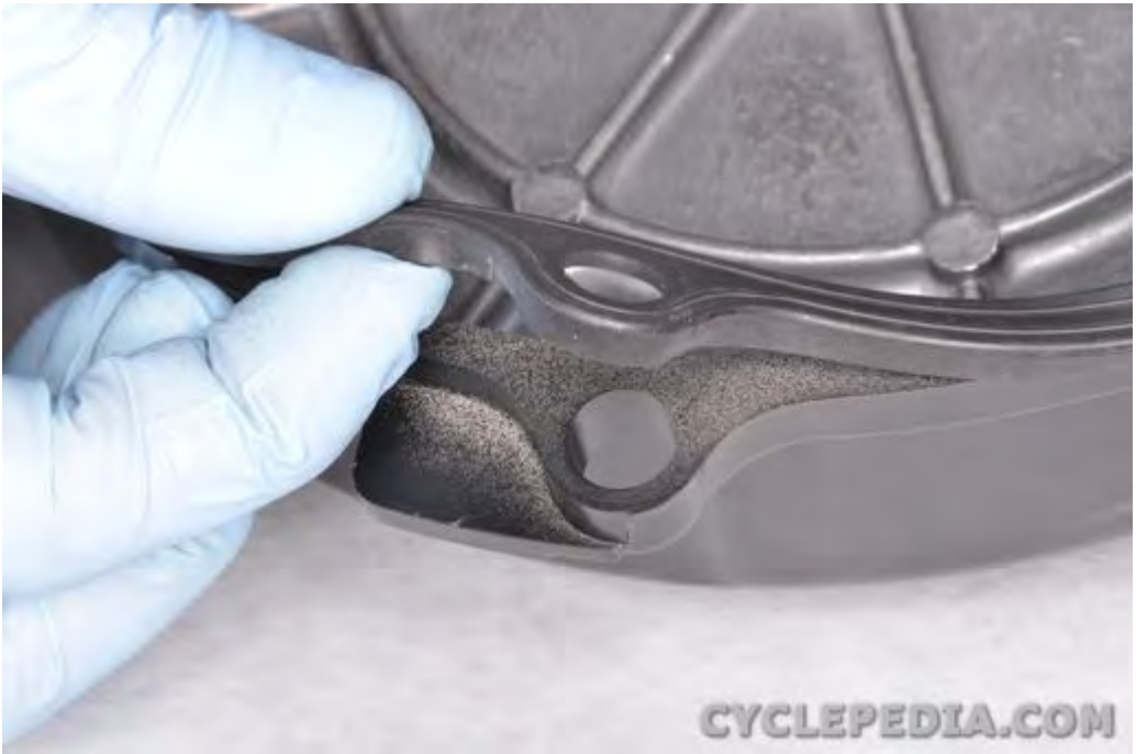
Remove the belt case cover rubber gasket.
