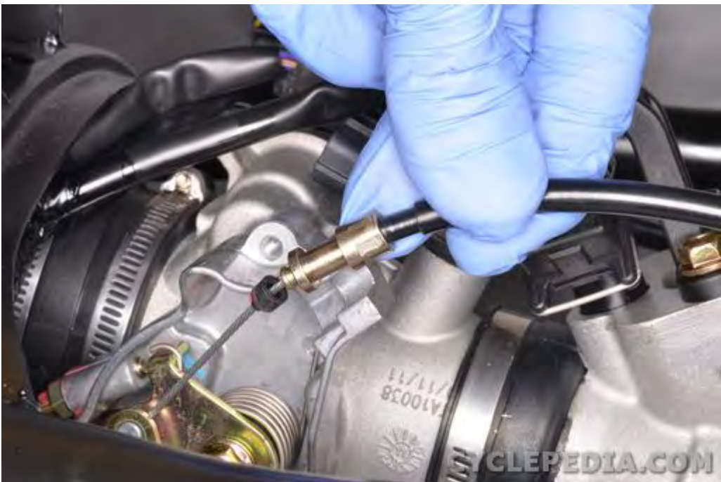
Fit the throttle cable into the throttle body as shown.
