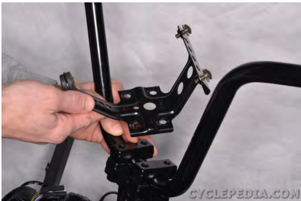
Set the instrument bracket into place.
