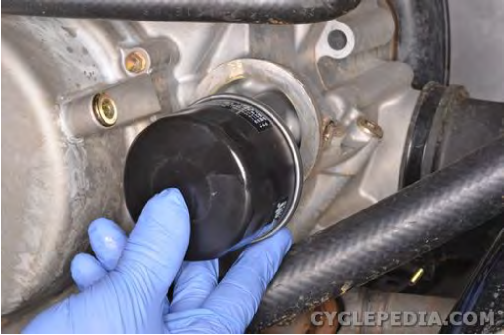
Remove the oil filter cartridge.
