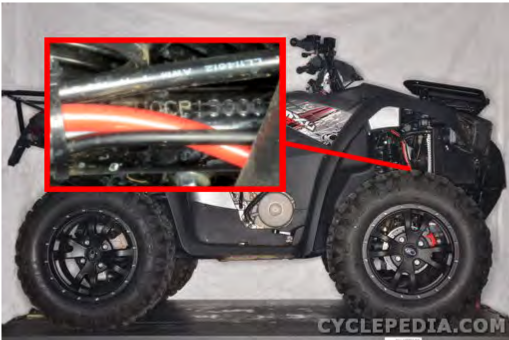
The VIN stamped into the front of the frame just in front of the front differential.
