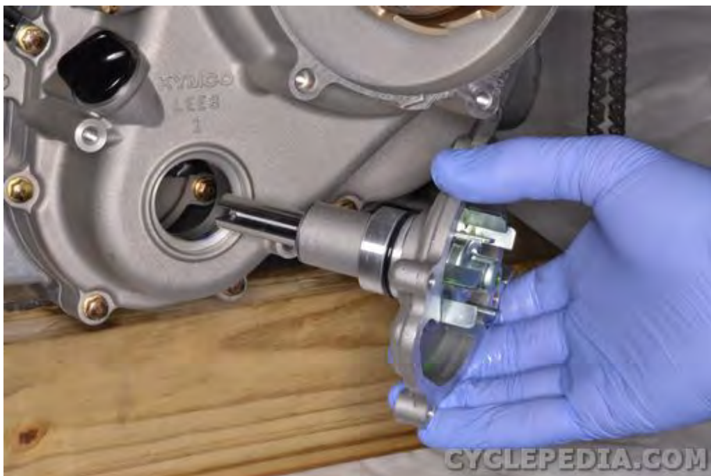
Fit the water pump body into place.
