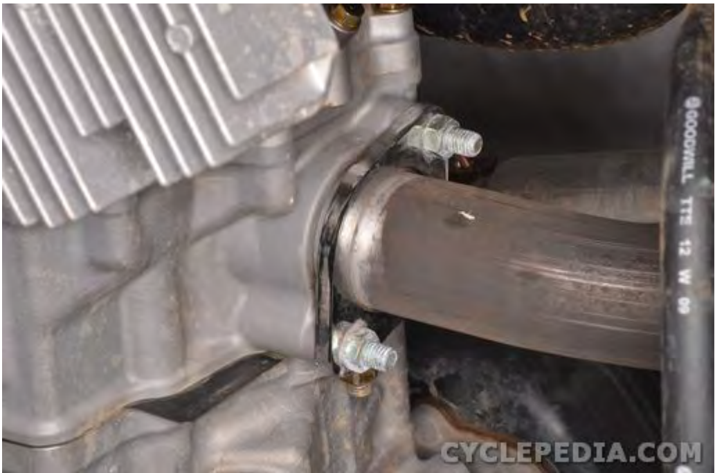
Thread on the exhaust pipe joint nuts. Tighten them securely with a 12 mm socket.
