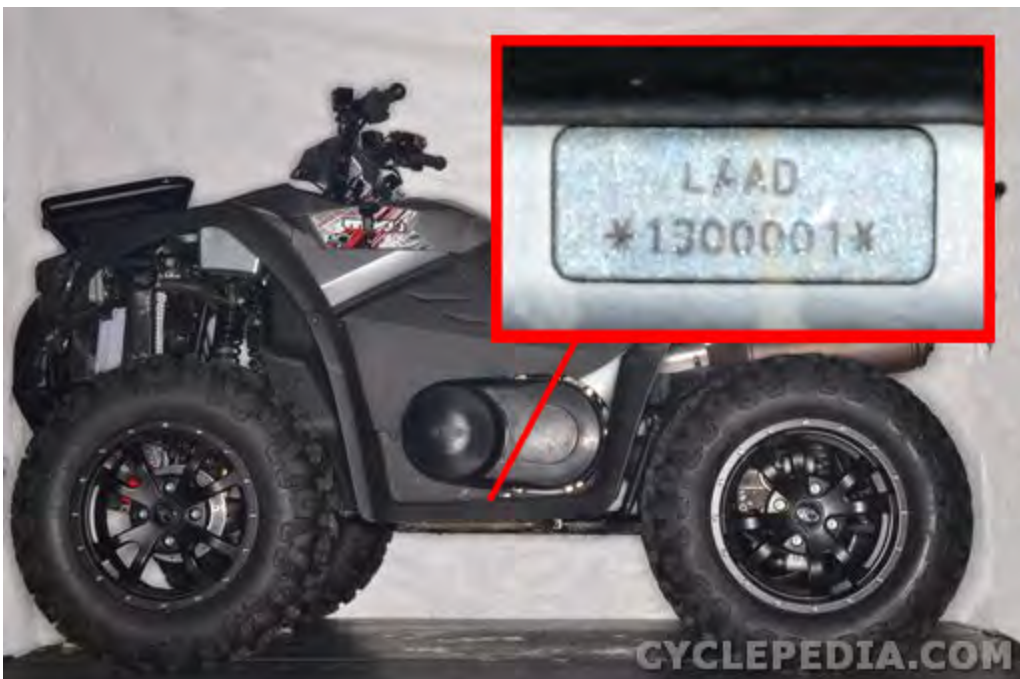
The engine number is located near the bottom of the left crankcase half.
