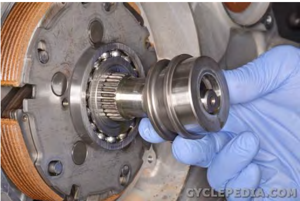
Slide off the outer clutch collar.
