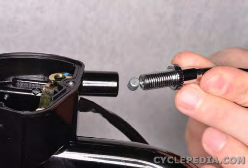
Thread the throttle cable into the throttle housing.
