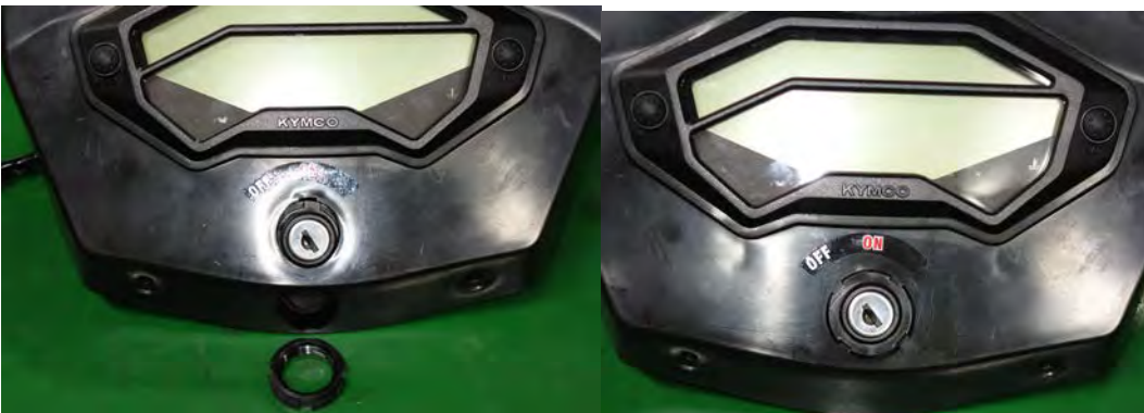
Install and tighten the ring to secure the main switch.
