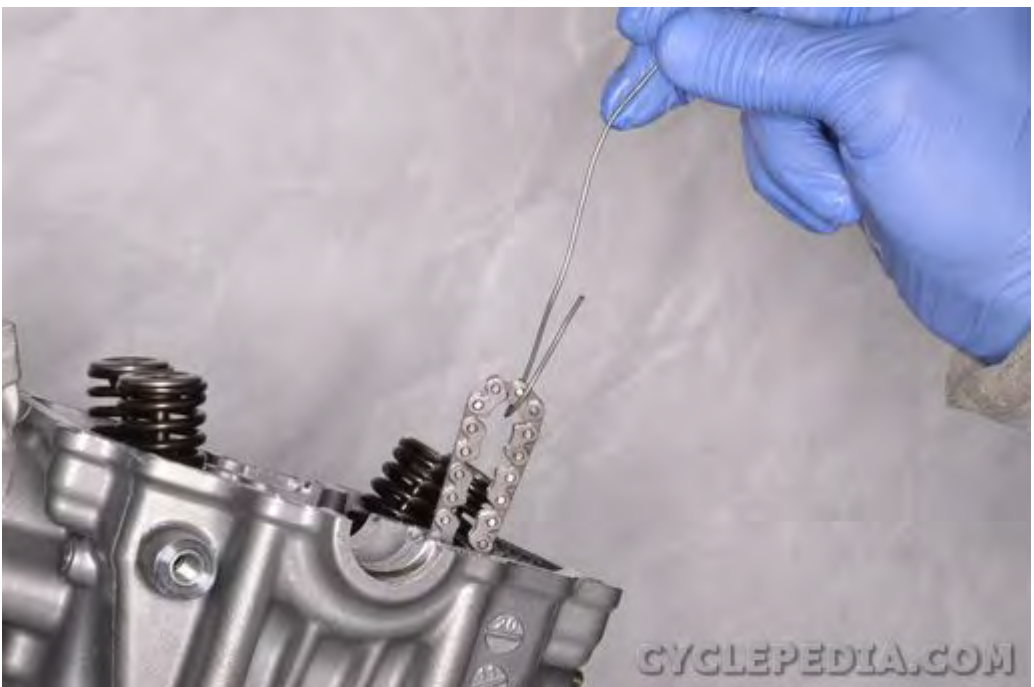
Secure the cam chain with a piece of wire to keep it from falling into the bottom end of the engine.
