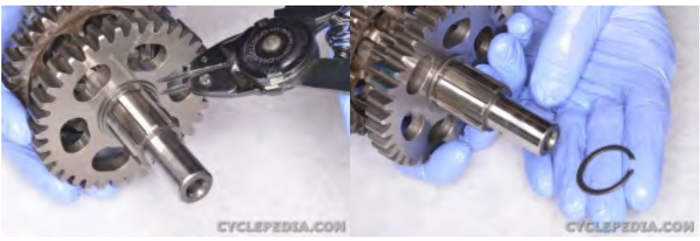
Remove the snap ring with snap ring pliers.
