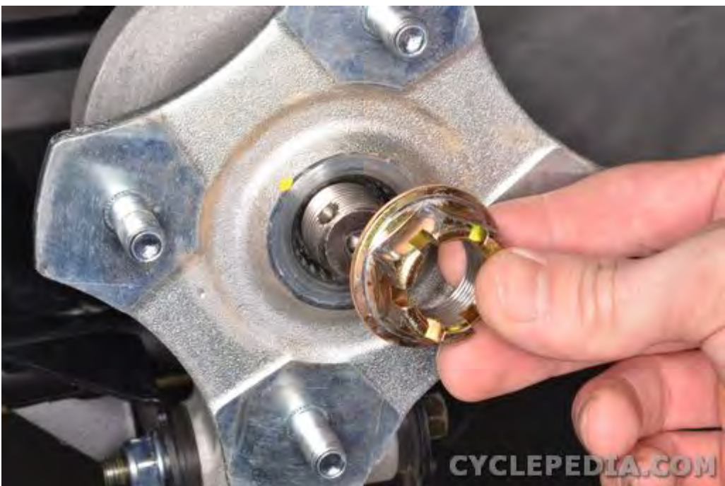
Thread on the wheel hub nut.
