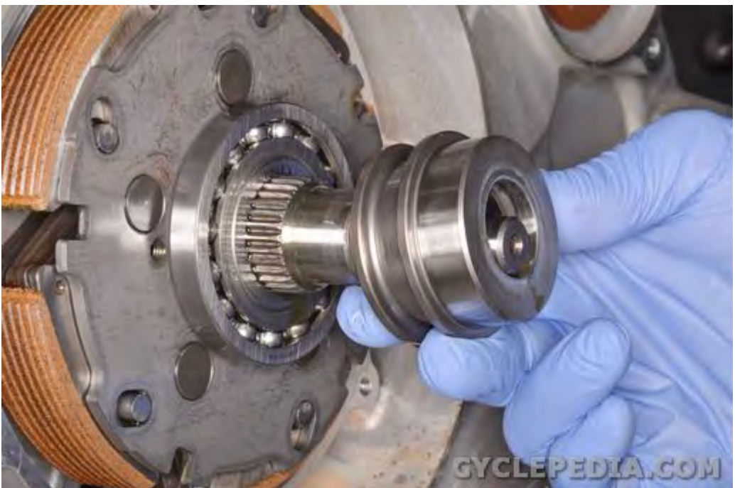
Slide the outer clutch collar onto the crankshaft.
