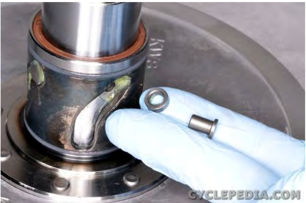
Remove the four guide rollers with guide roller pins.
