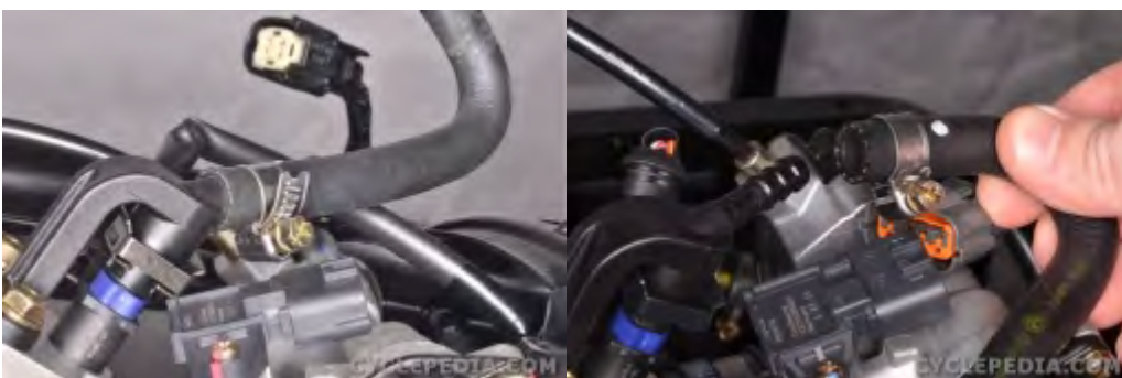
Loosen the fuel injector hose clamp with a #2 Phillips screwdriver. Disconnect the fuel hose from the fuel injector.
