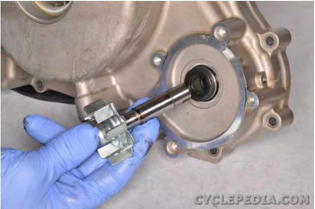
Remove the water pump impeller from the generator cover.
