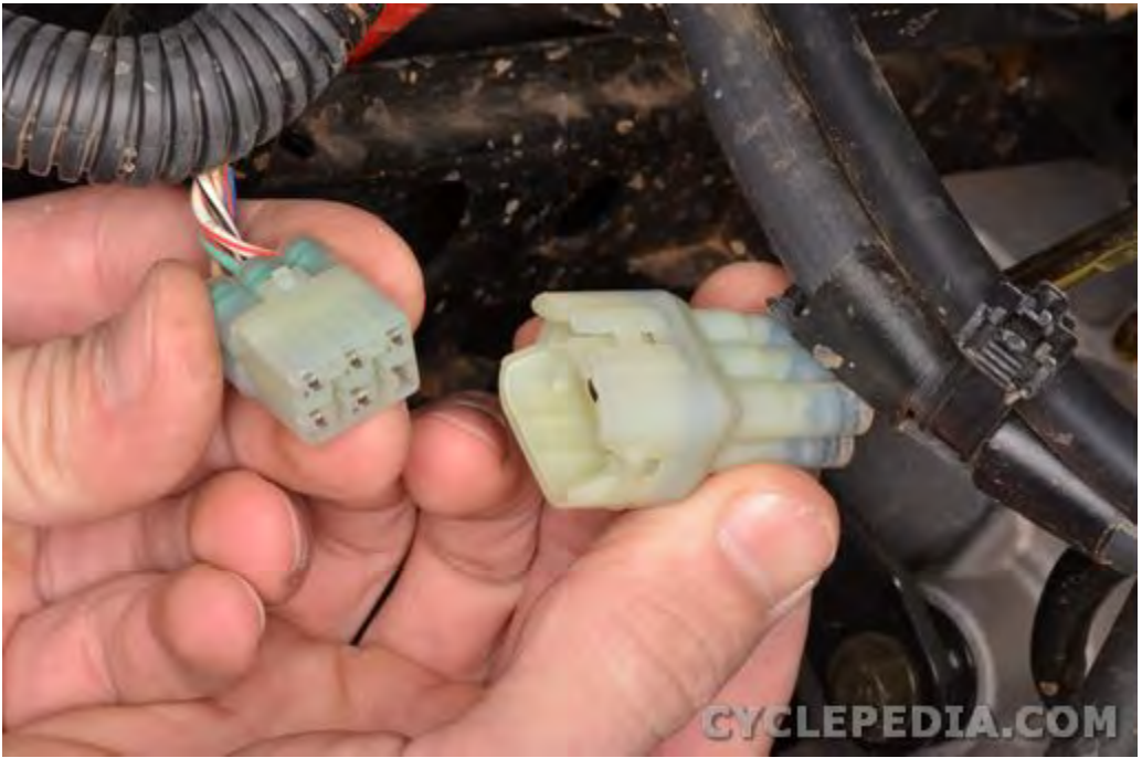
Plug in the gear position switch connector.
