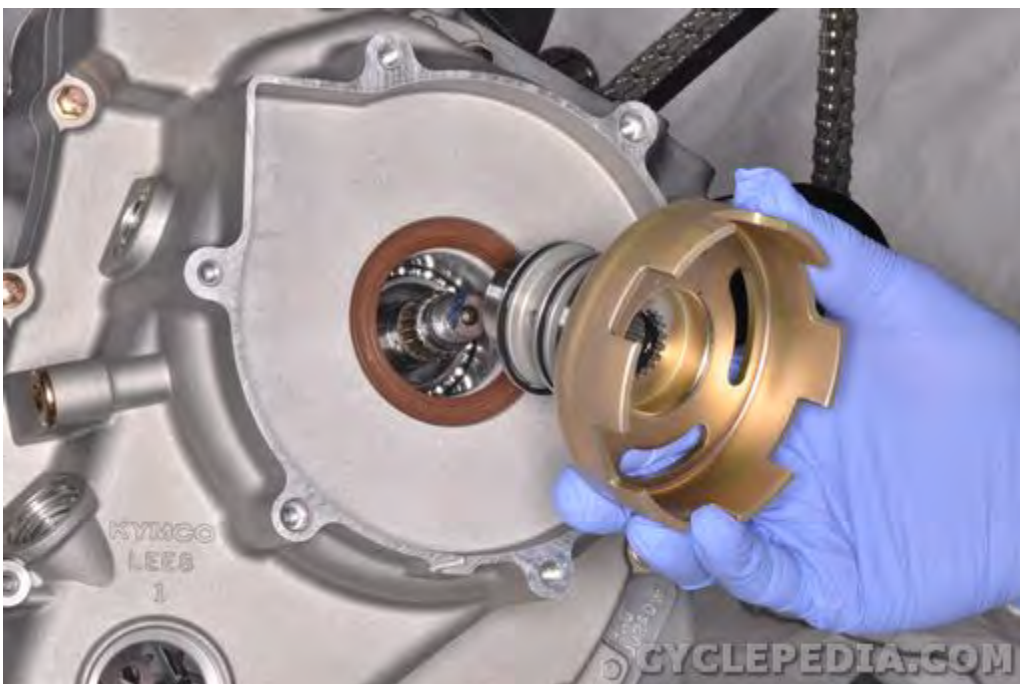
Slide out the recoil starter drum. Be careful to not damage the oil control rings.
