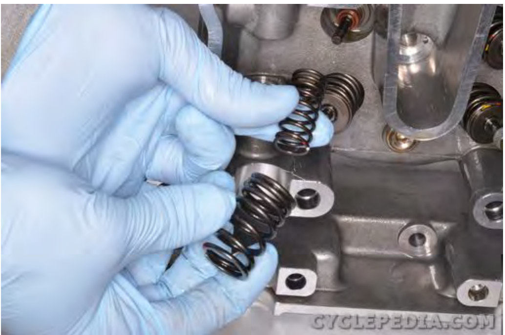
Lift out the valve springs.
