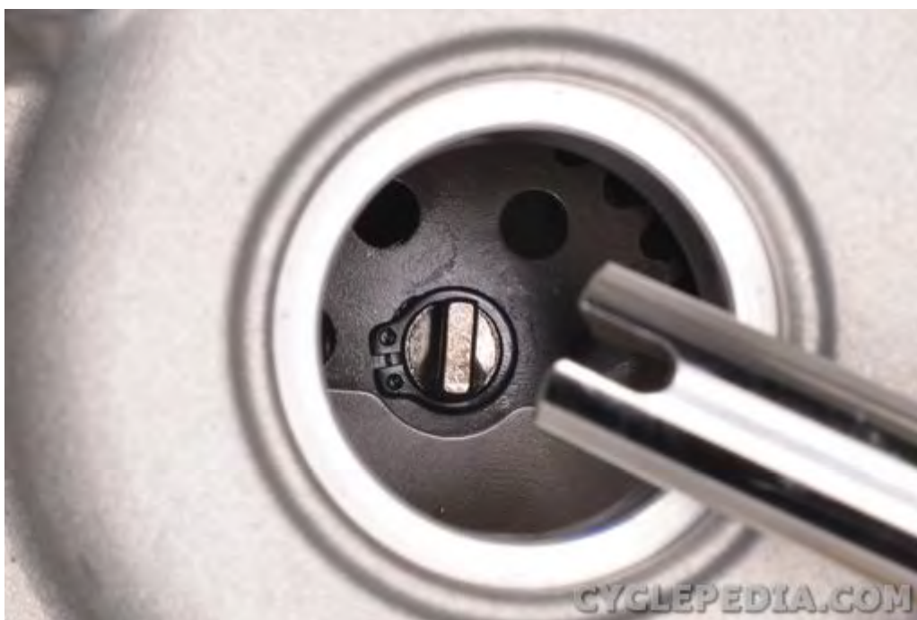
Guide the water pump shaft groove onto the end of the oil pump shaft.
