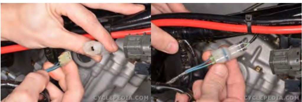
Plug in the 2-pin ignition pulse generator / crank position sensor connector.
