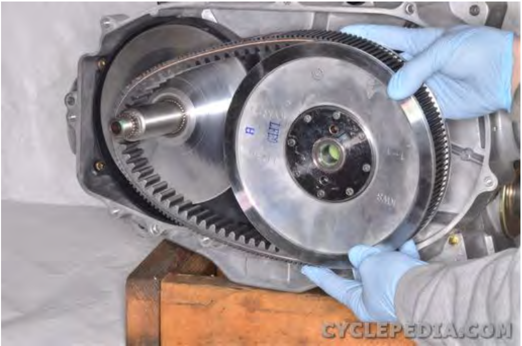
Install the driven pulley onto the driven pulley shaft.
