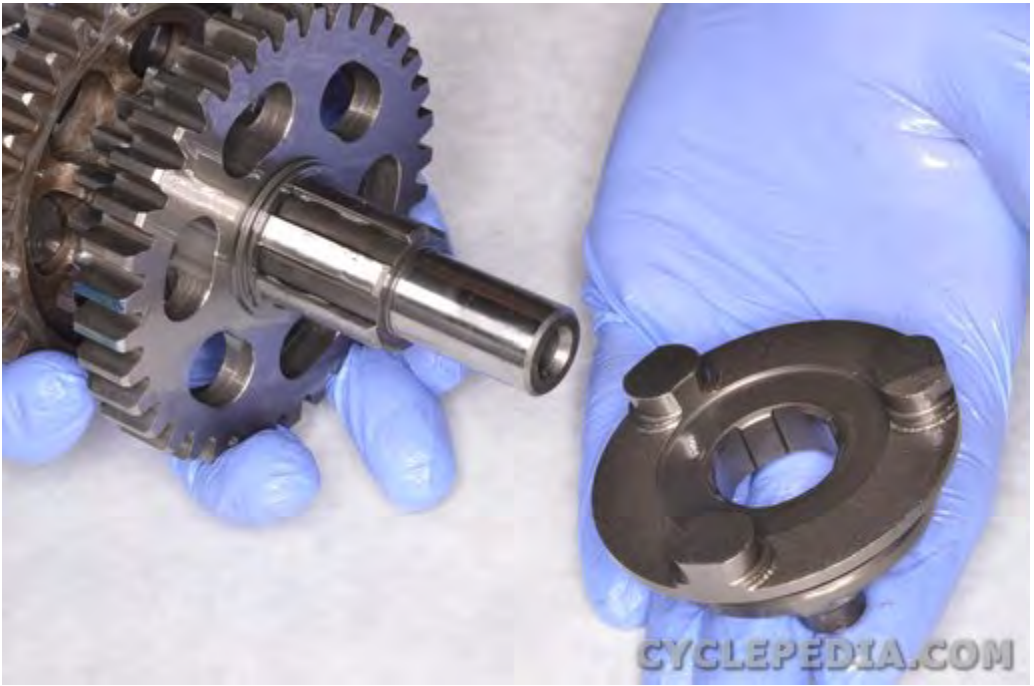
Remove the high/low gear shifter.
