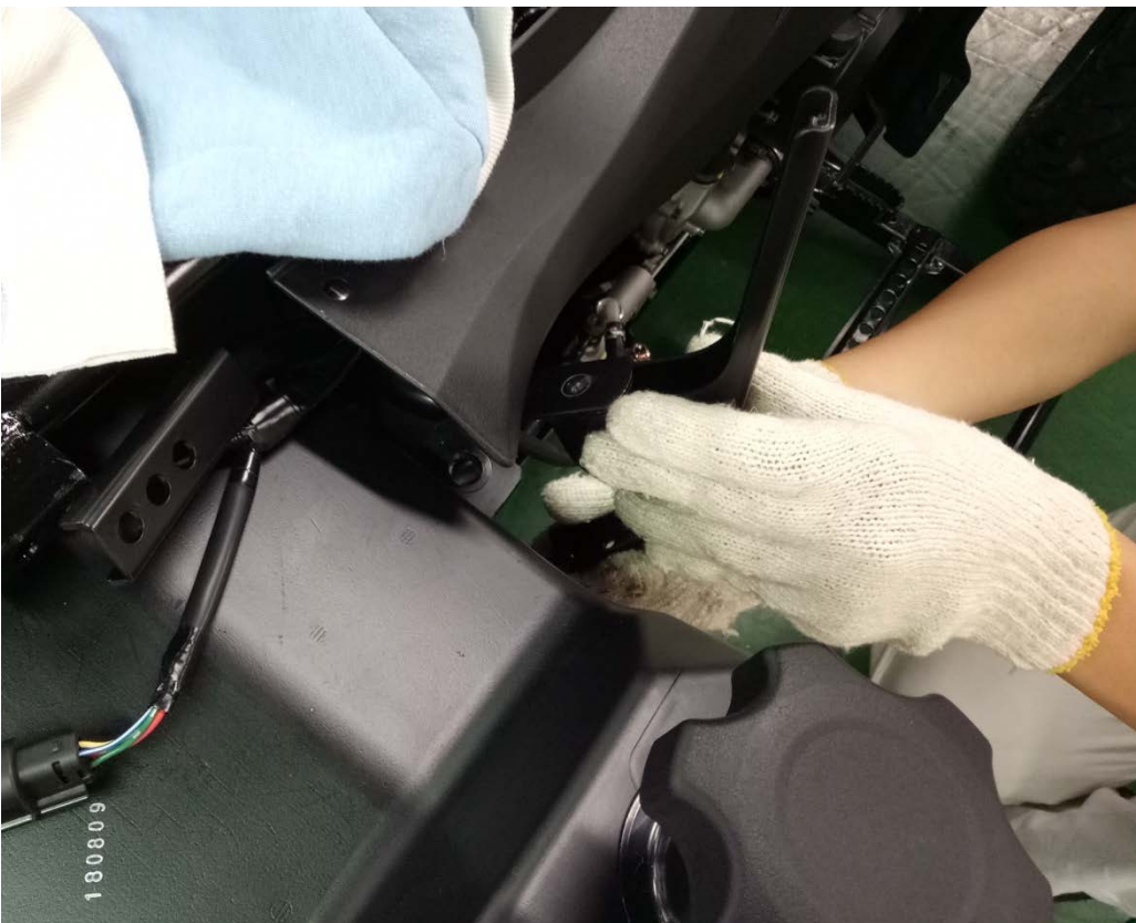
Remove the fuel tank front pipe.
