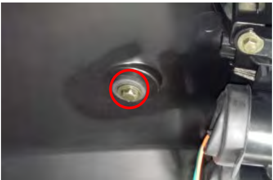
Remove the two rear bolts with a 10 mm socket.
