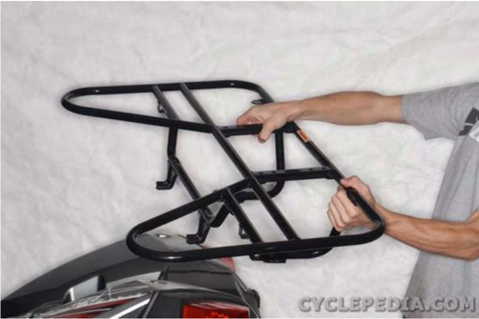
Lift off the rear rack carrier.
