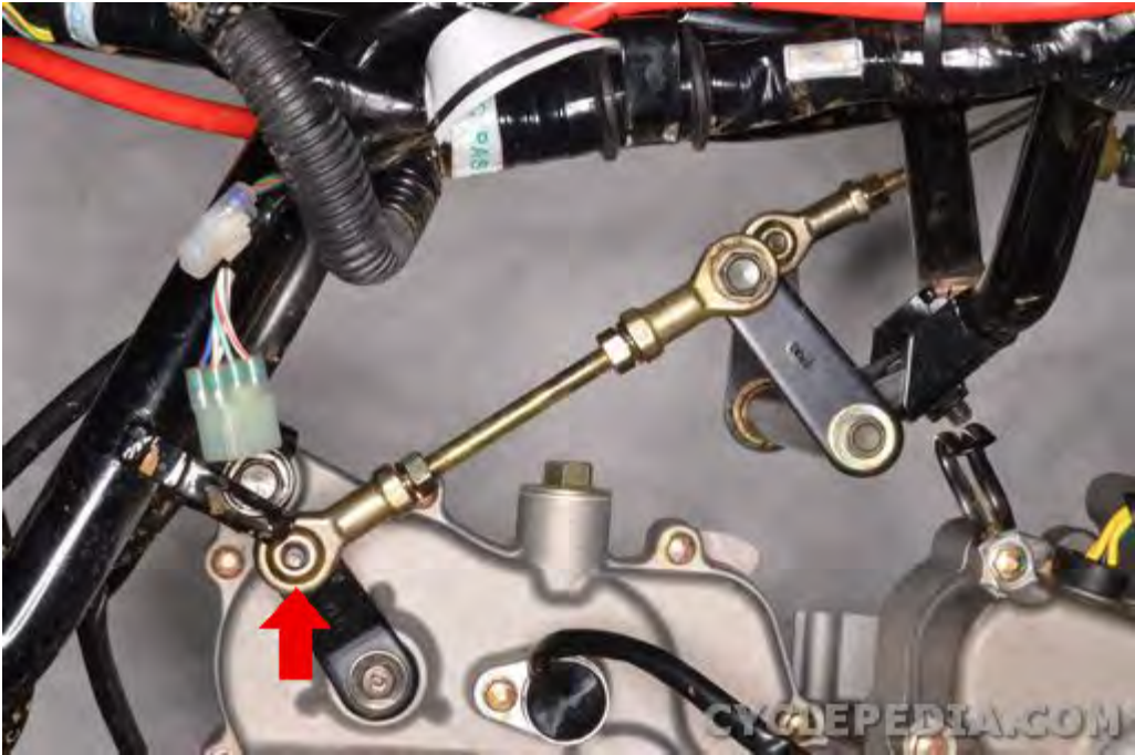
Remove the nut from the engine side of the linkage.
