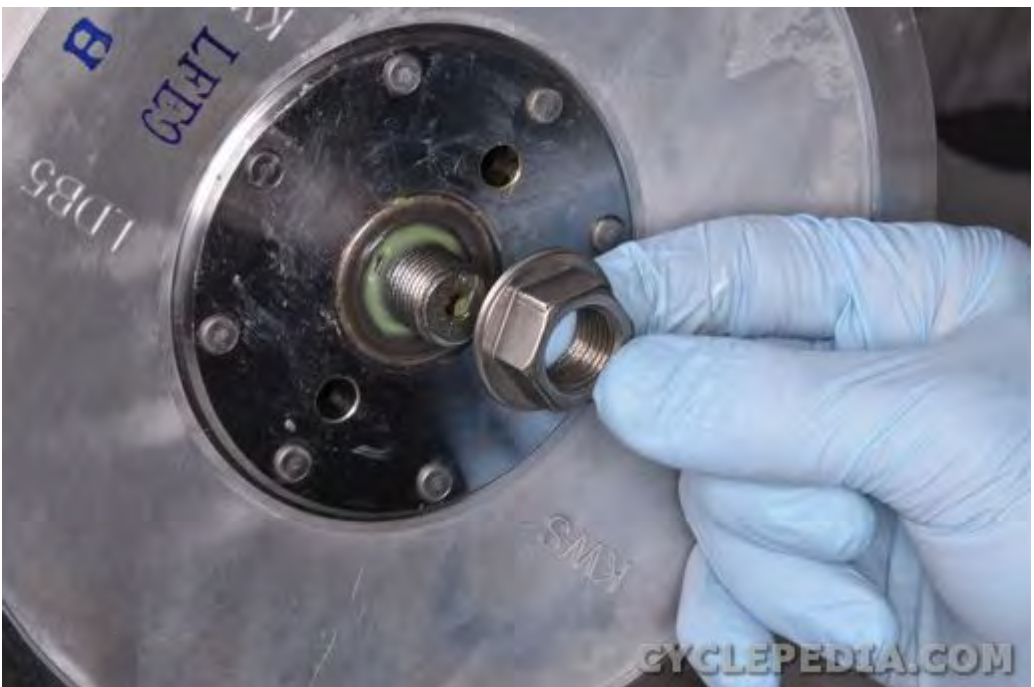
Lubricate the threads of the driven pulley nut with oil. Thread on the driven pulley nut.
