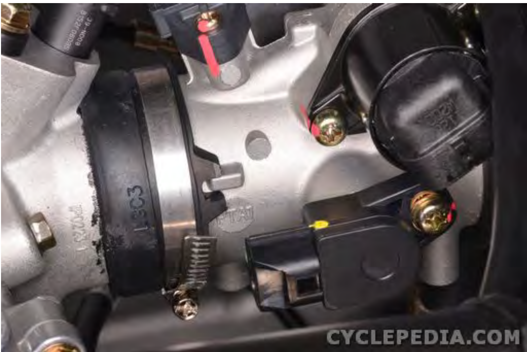
The throttle body is held to the intake pipe with a clamp.
