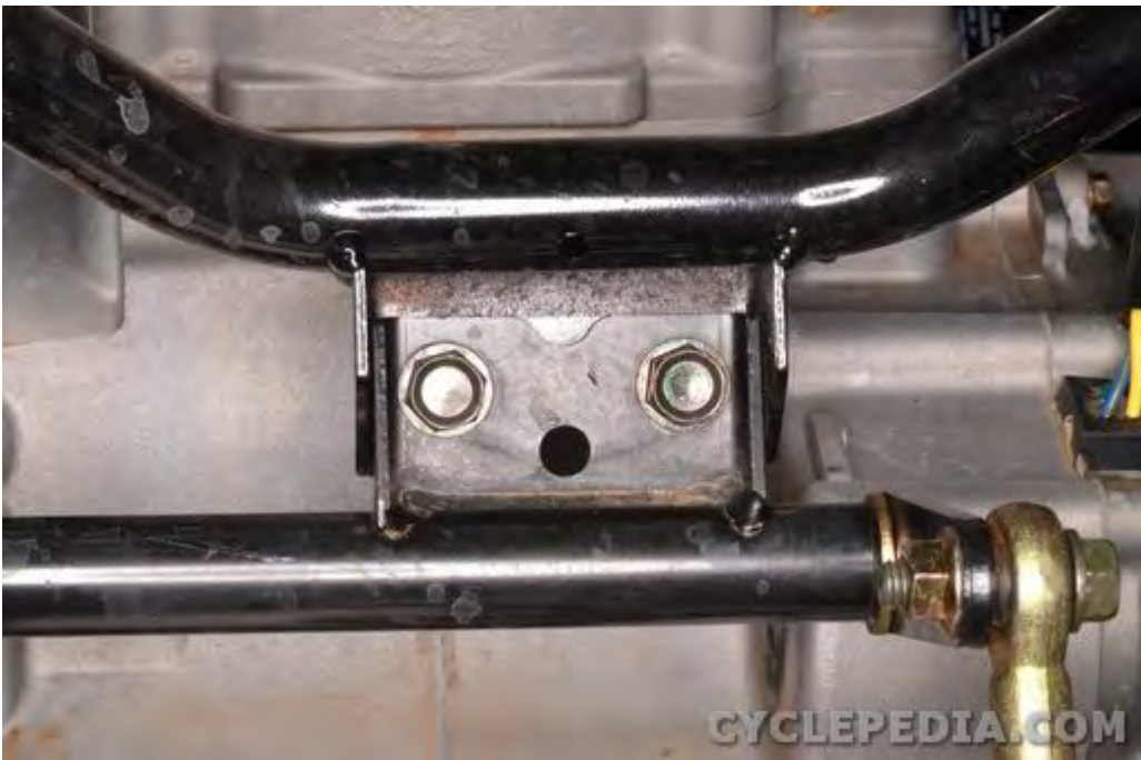
Remove the two linkage pivot mounting bolts.
