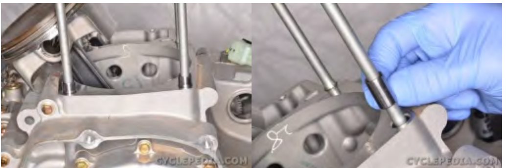
Remove the two dowel pins.
