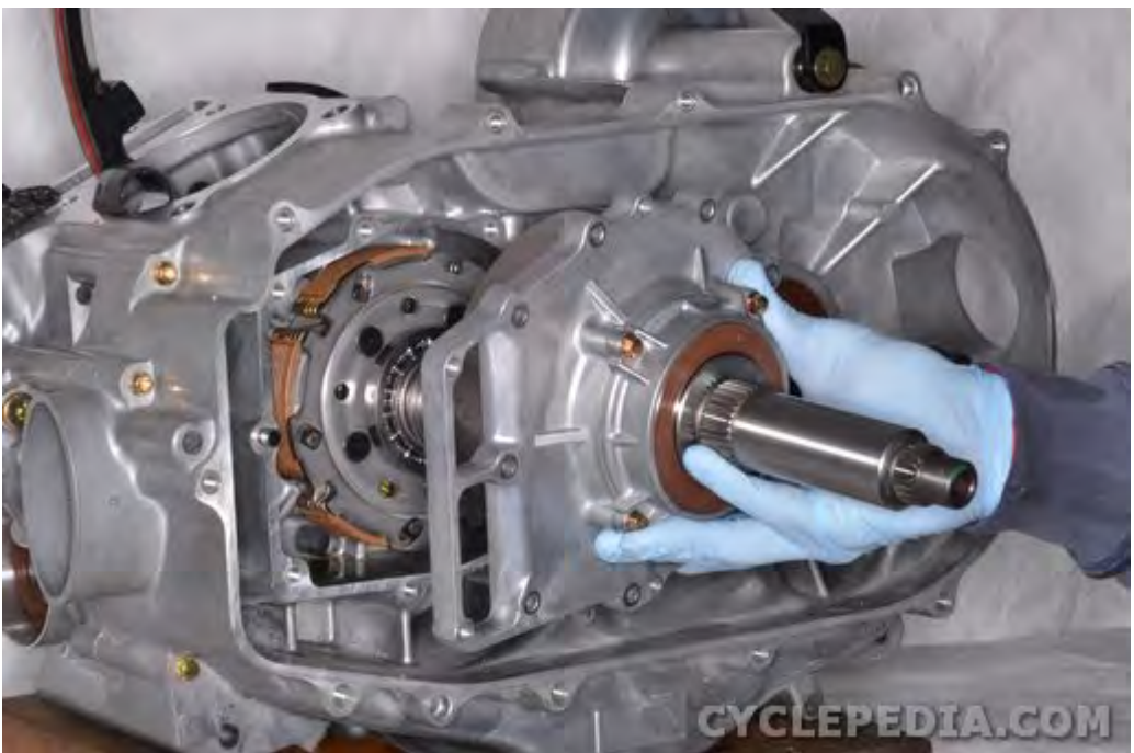
Remove the clutch cover assembly evenly.
