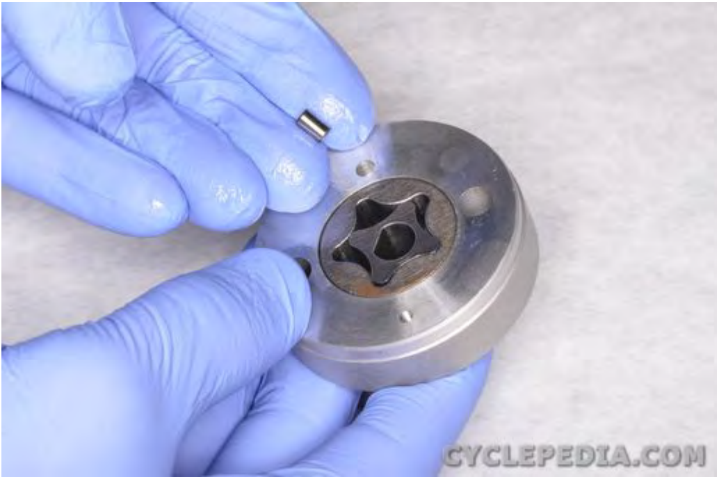
Remove the oil pump dowel pin.
