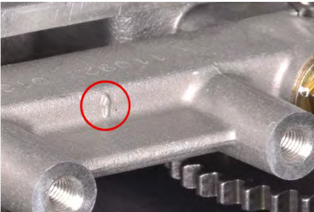
The arrow on the camshaft holder must face out.
