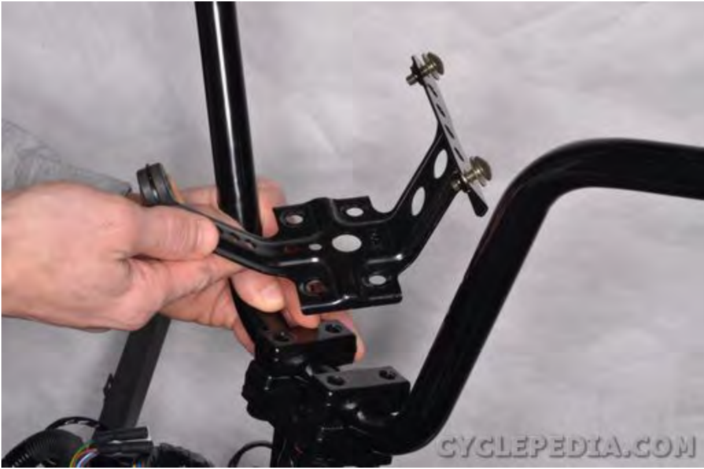
Lift off the instrument bracket.
