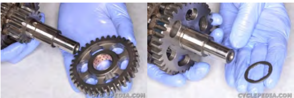
On the other side of the countershaft; Install the low drive gear and washer.
