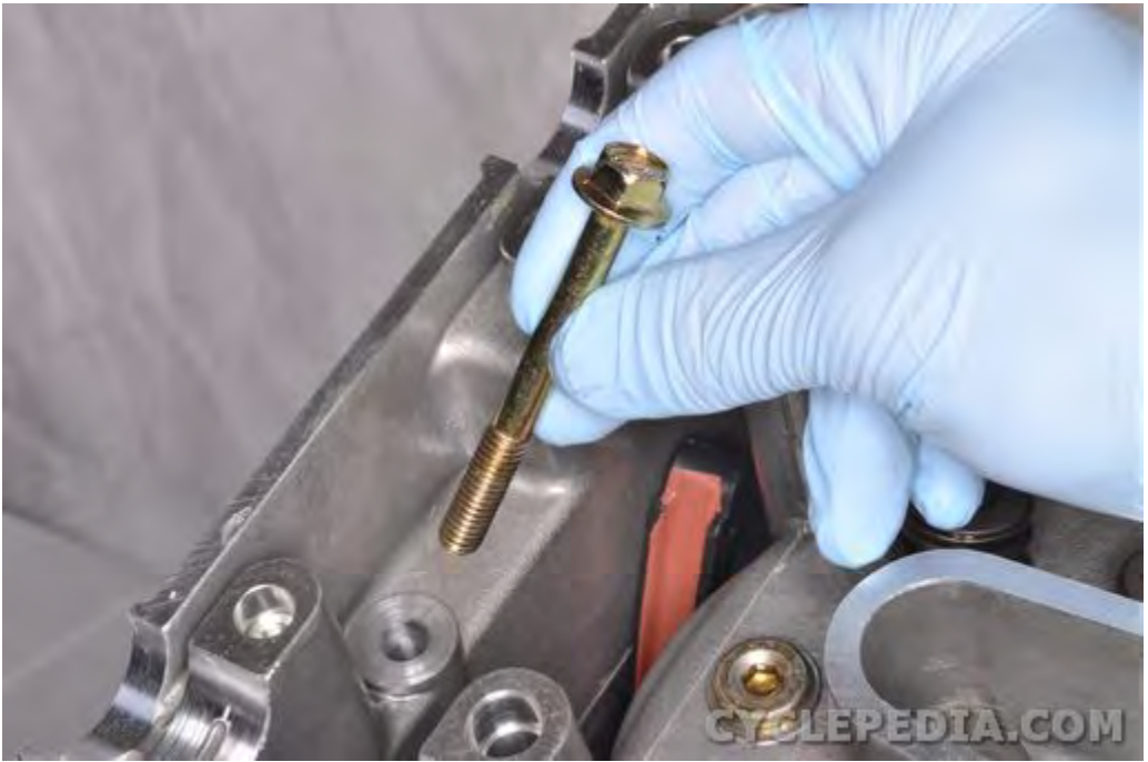
Remove the cylinder head bolt.
