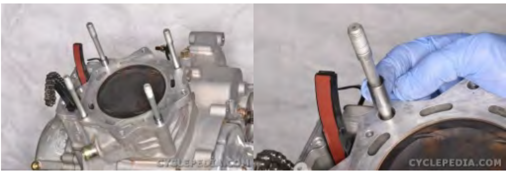
Remove the two cylinder head dowel pins.
