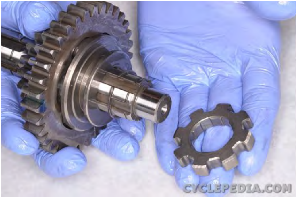
Install the stopper wheel.
