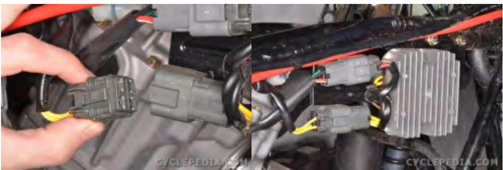
Plug in the 4-pin stator connector.
