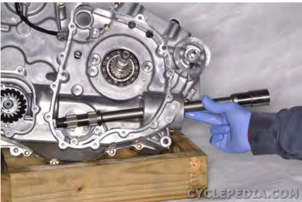
Slide the output shaft out of the engine.
