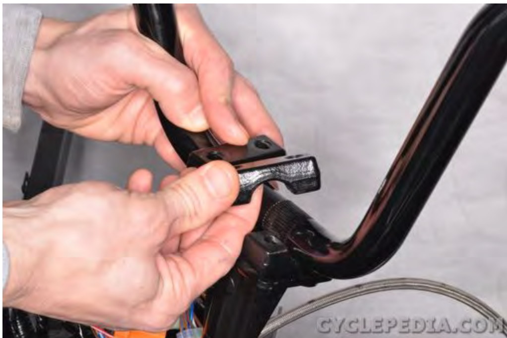
Set the handlebar clamps into place.
