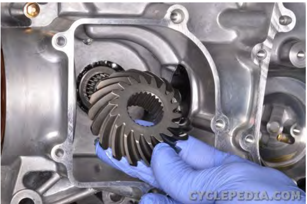
Slide off the drive bevel gear.
