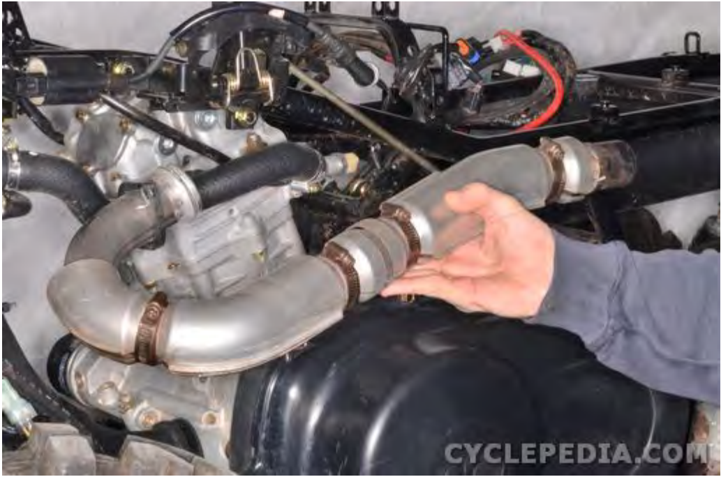
Fit the exhaust pipe into place.
