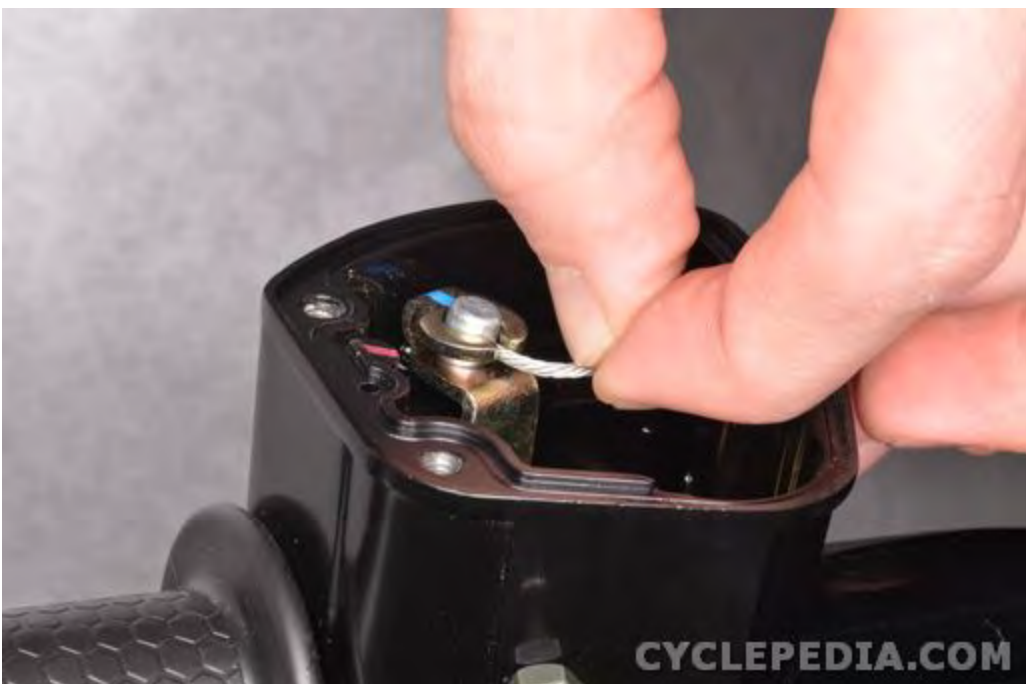
Connect the end of the throttle cable to the throttle lever.
