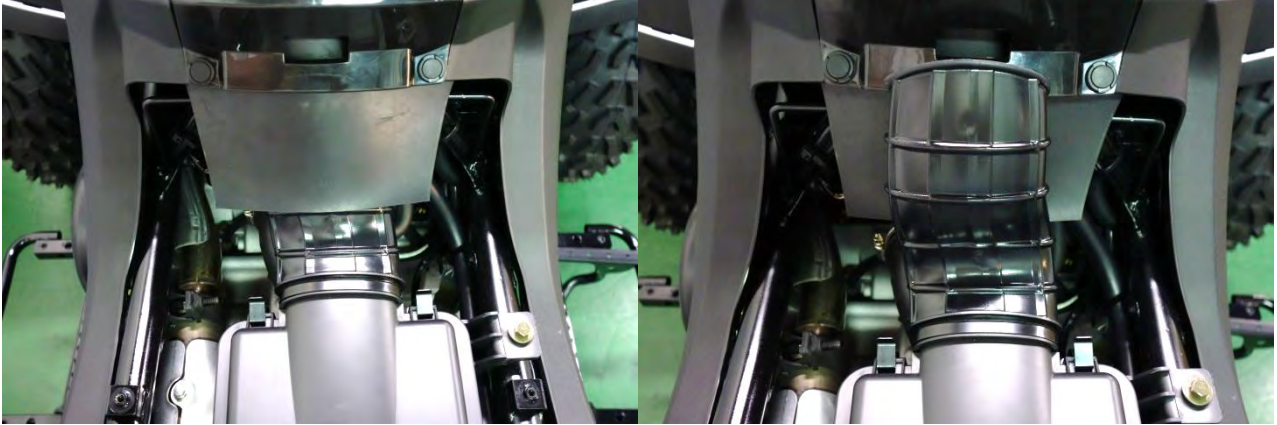
Pull out the air/c chamber duct.
