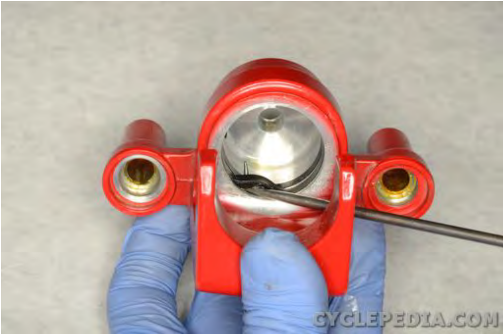
Remove the dust seal from the caliper bore and discard.
