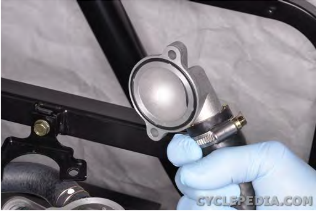
Remove the O-ring from the housing cover.
