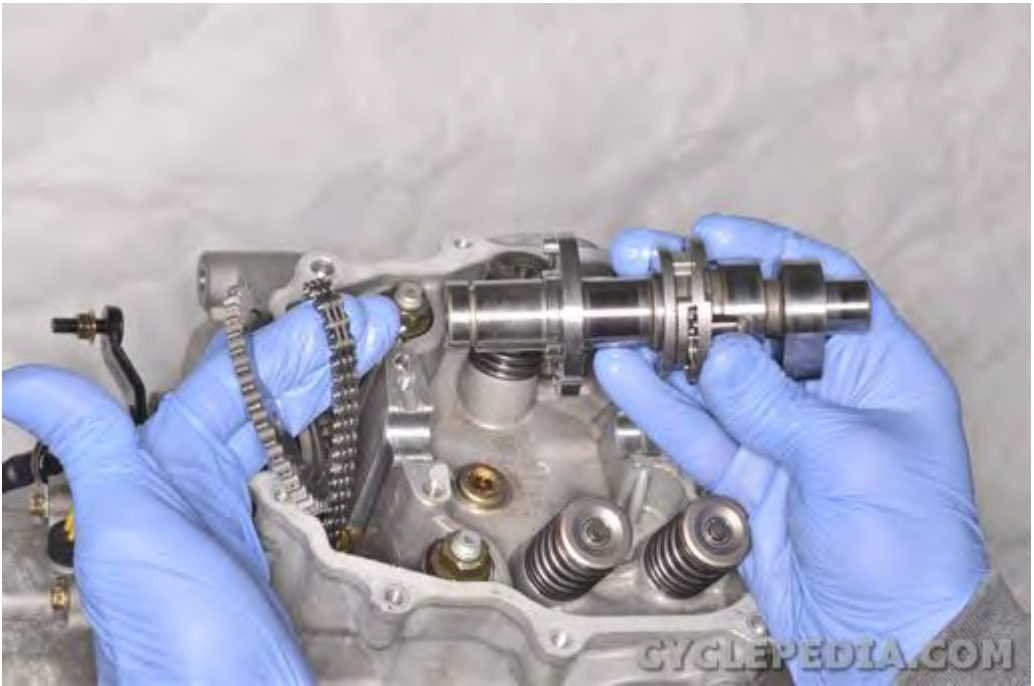
Remove the camshaft and sprocket.
