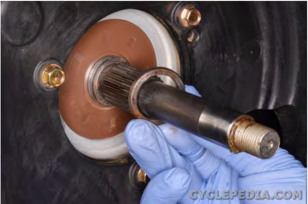
Remove the washer from the driven pulley shaft.
