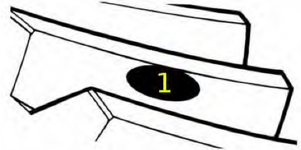
1 - Incorrect (contact at tooth top)
