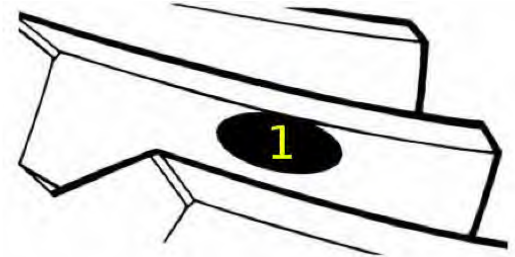
1 - Incorrect (contact at tooth top)
