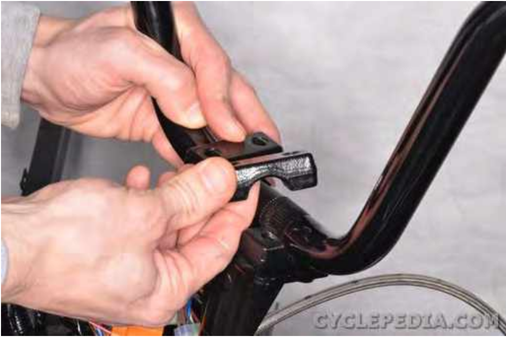
Set the handlebar clamps into place.
