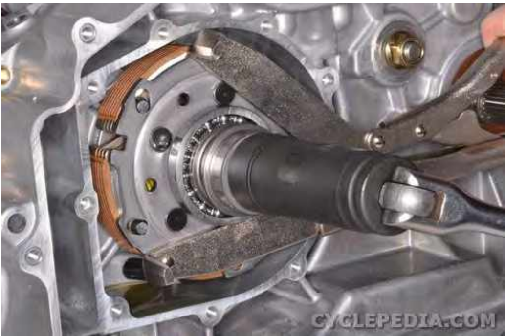
Hold the clutch with the Y-type holder and torque the clutch nut to specification with a deep well commercially available 26 mm socket.
