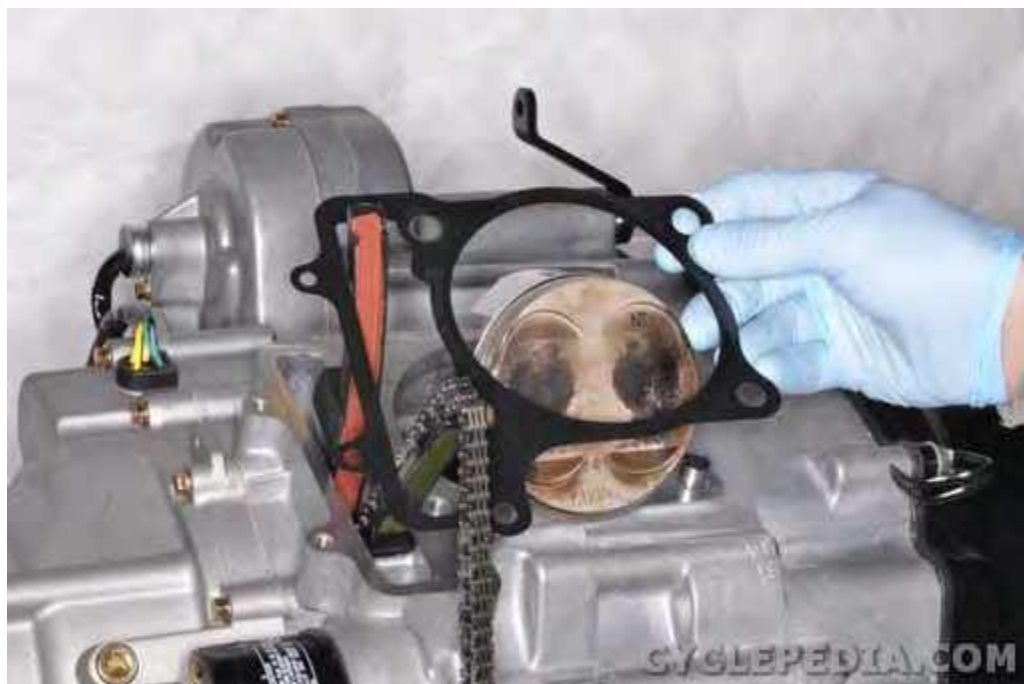
Lift off the base gasket.
