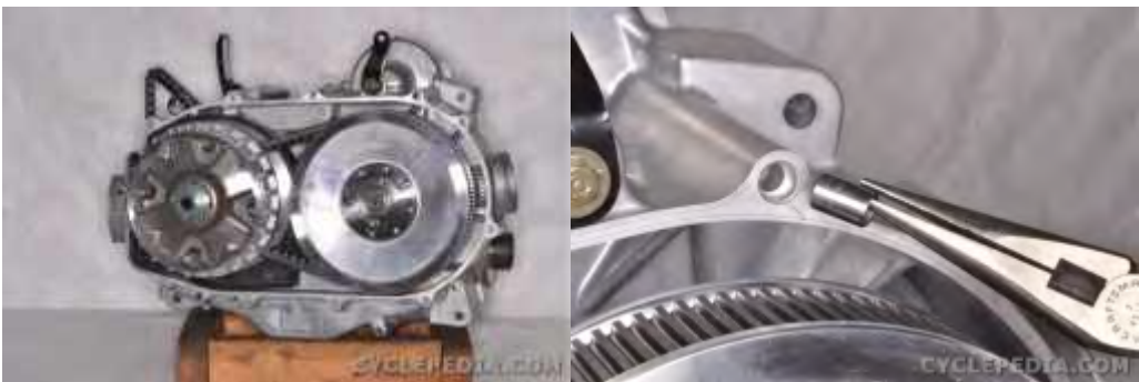
Remove the two belt case cover dowel pins.
