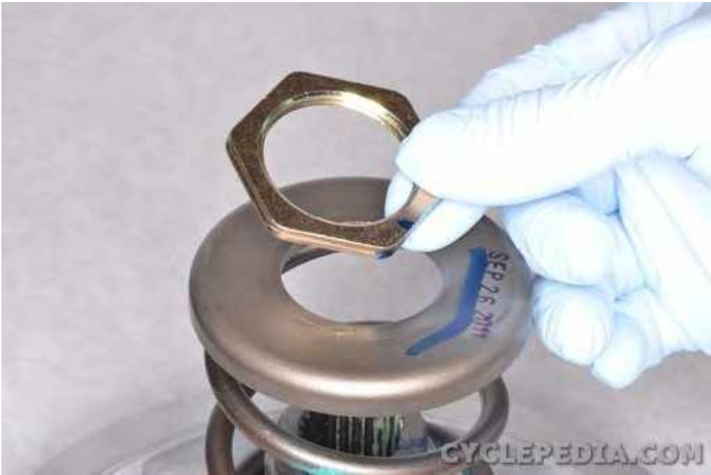
Remove the special tool components and the nut.
