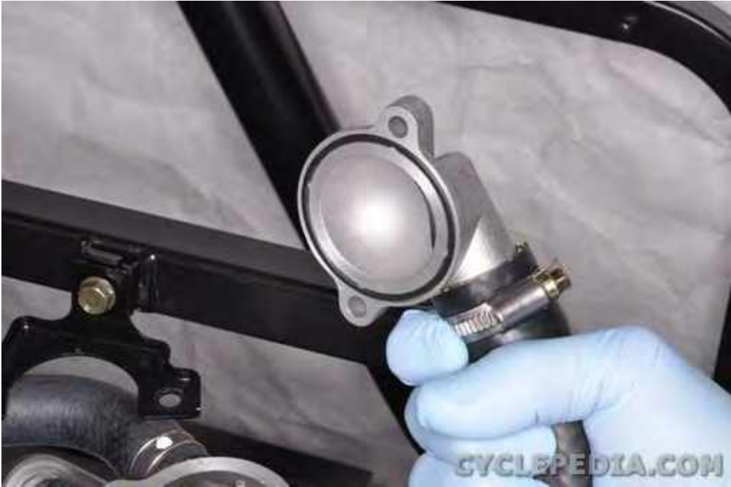
Remove the O-ring from the housing cover.
