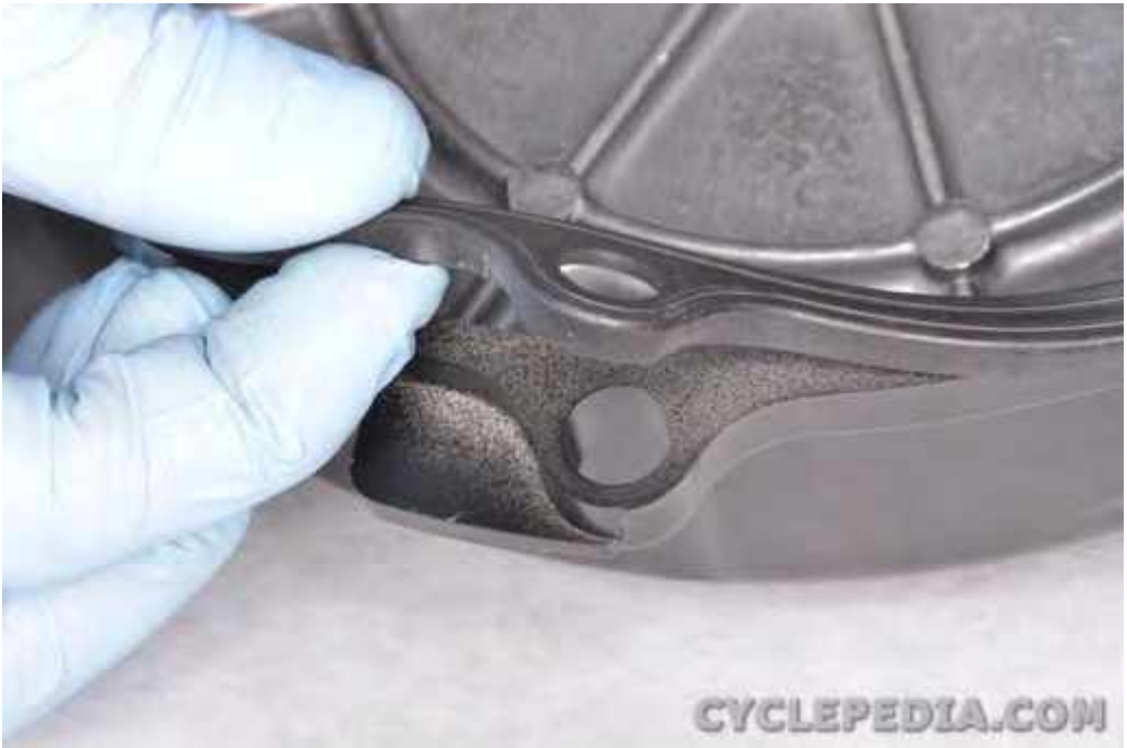
Remove the belt case cover rubber gasket.
