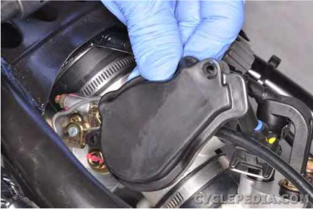
Remove the throttle drum cover.
