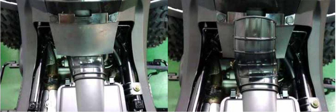
Pull out the air/c chamber duct.
