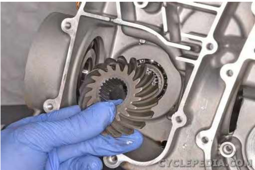
Slide off the drive bevel gear.
