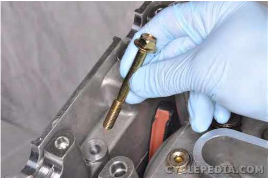
Remove the cylinder head bolt.
