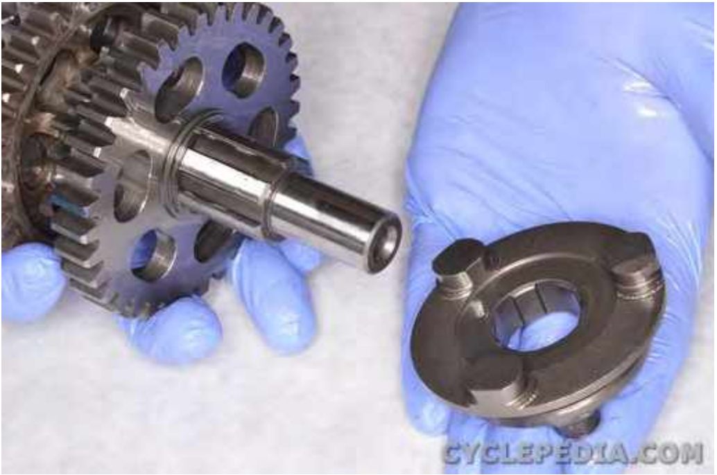
Remove the high/low gear shifter.
