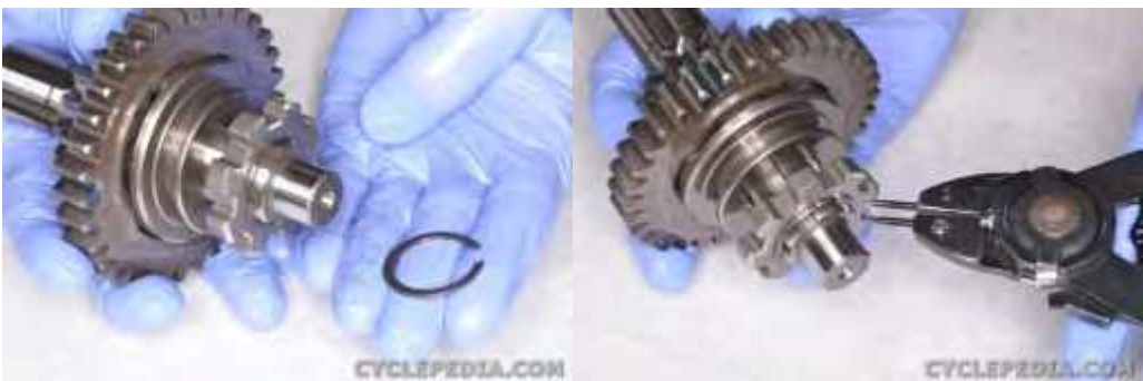
Install the snap ring with snap ring pliers.
