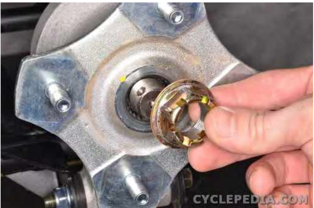
Thread on the wheel hub nut.
