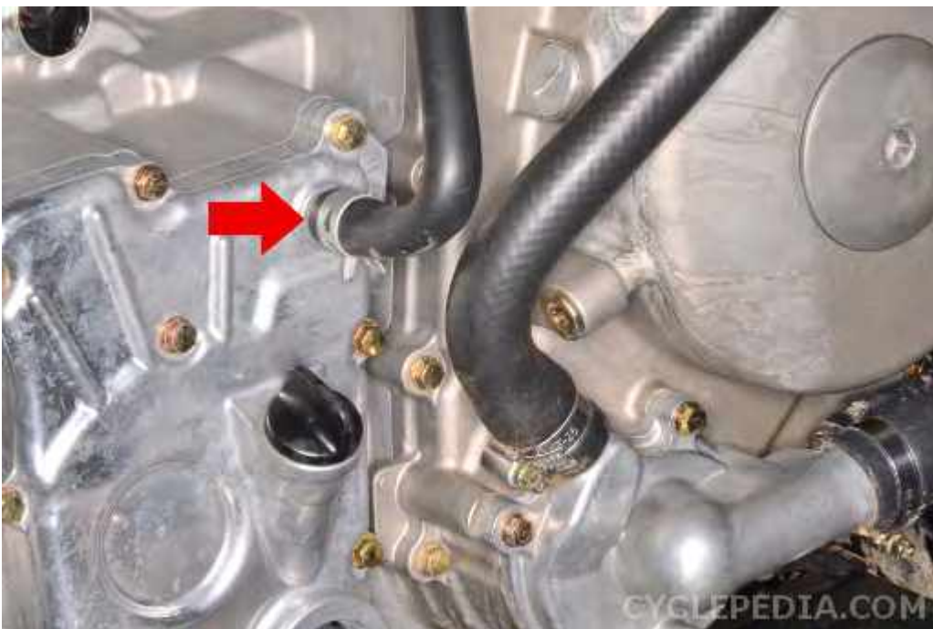
Free the breather hose from the bevel gear cover on the MXU 700i models.
