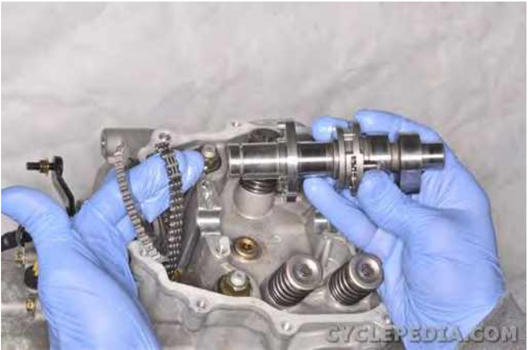
Remove the camshaft and sprocket.
