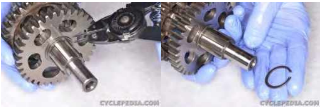
Remove the snap ring with snap ring pliers.
