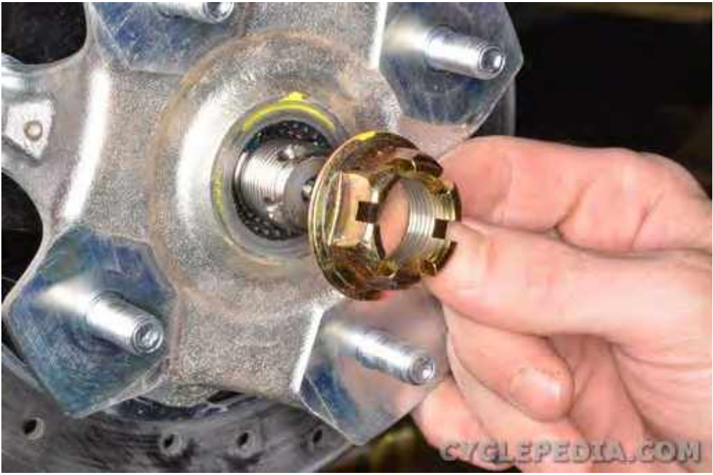
Thread on the wheel hub nut.
