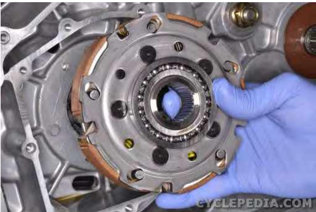
Slide the clutch assembly off of the crankshaft.
