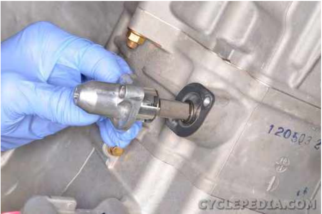
Remove the cam chain tensioner and gasket.
