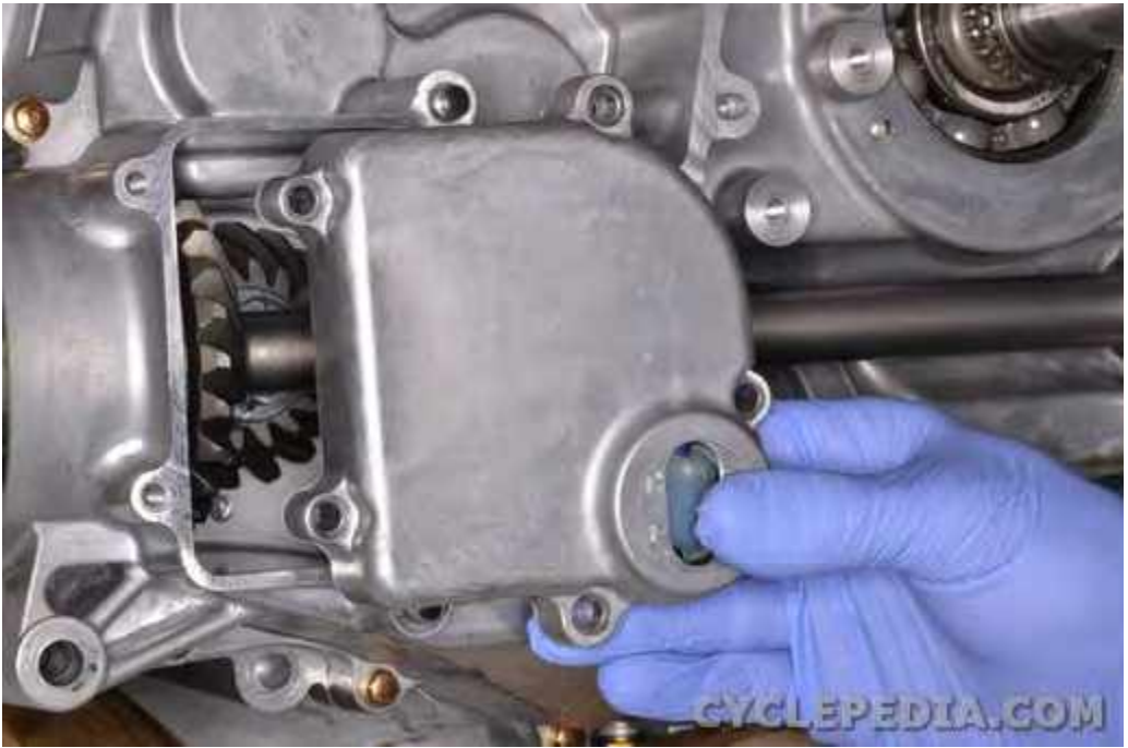
Remove the bevel gear cover.
