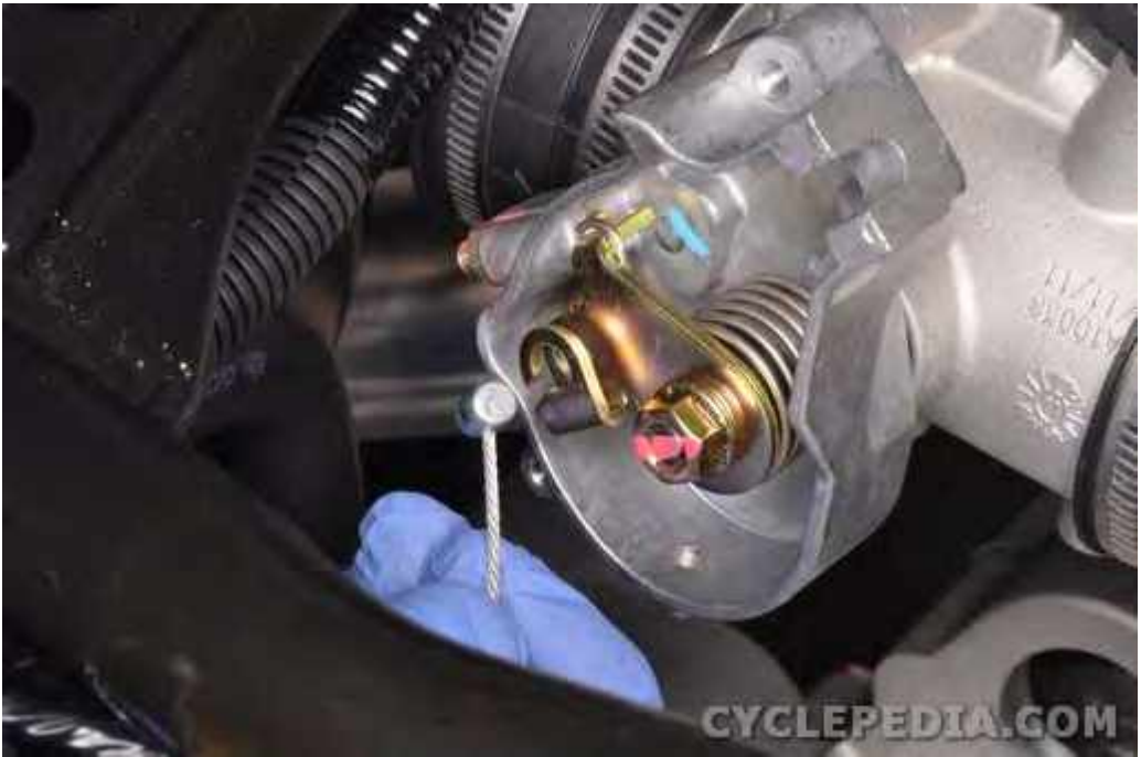
Fit the end of the throttle cable into the throttle drum.
