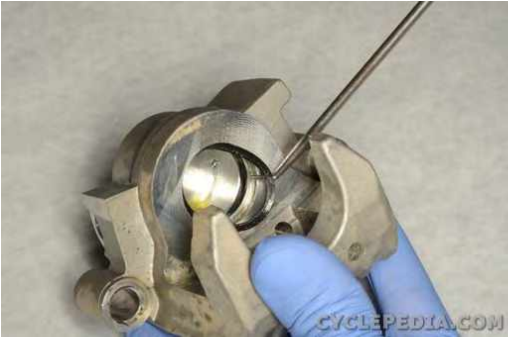
Remove the dust seal from the outer caliper bore and discard.
