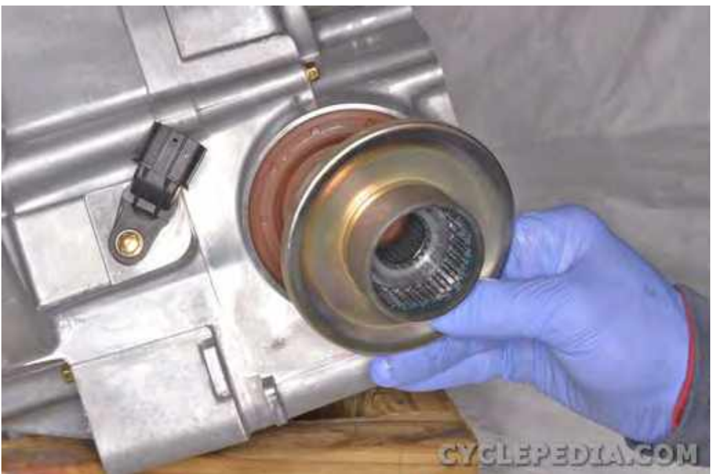
Remove the rear propeller shaft coupler from the engine.
