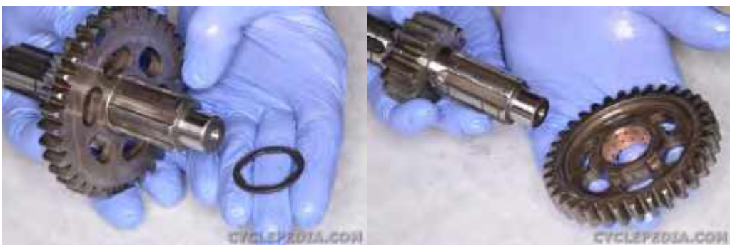
Remove the washer and reverse drive gear.
