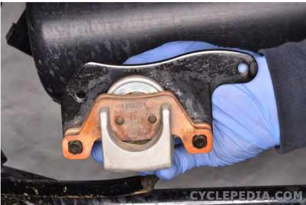
Apply silicone grease to the caliper bracket pins. Install the caliper bracket.
