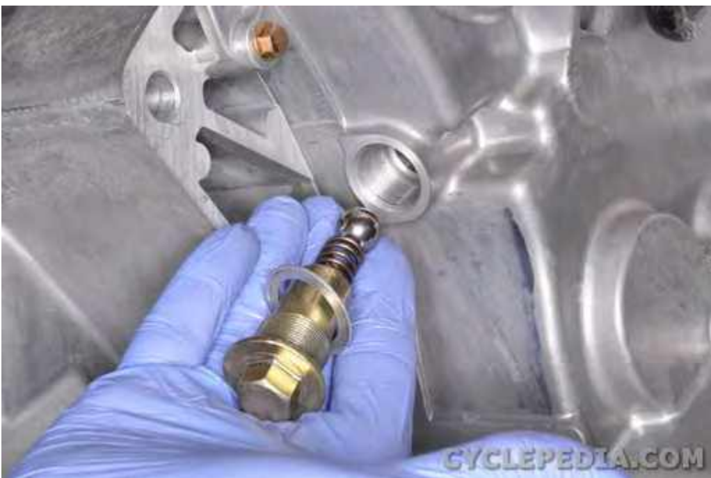
Remove the stopper plug, washer, spring, and stopper ball.
