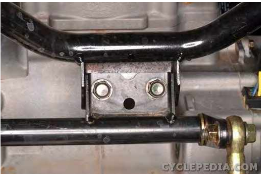
Remove the two linkage pivot mounting bolts.
