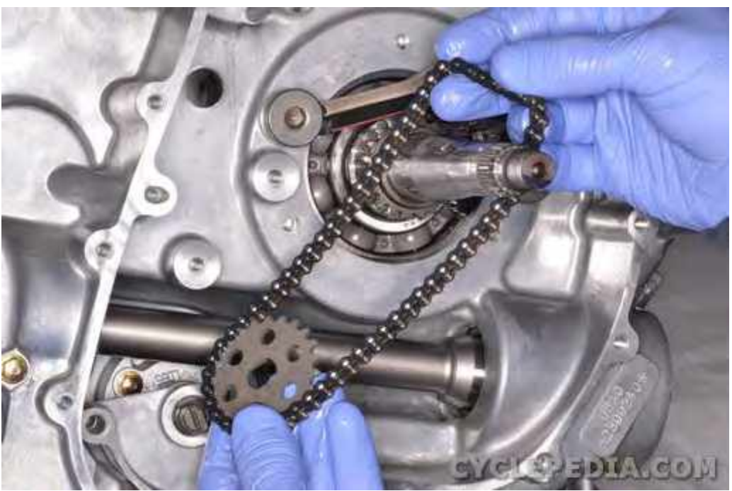
Install the oil pump shaft holder bolt. Do not tighten, yet.
