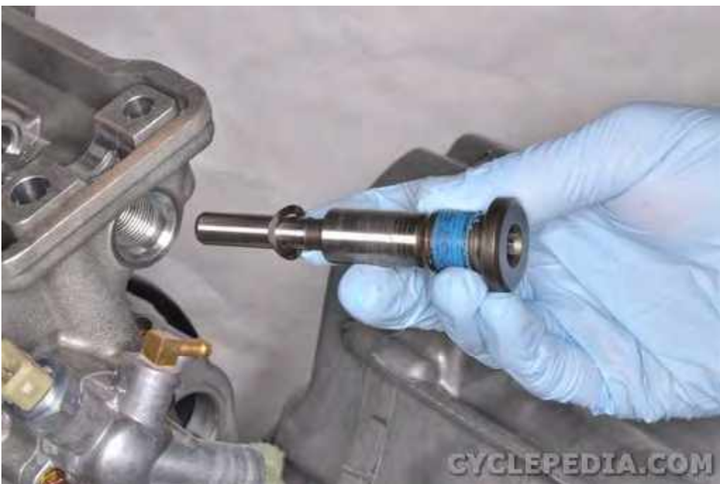
Remove the rocker arm shafts and washers from the cylinder head.
