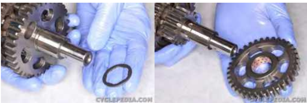
Remove the washer and low drive gear.
