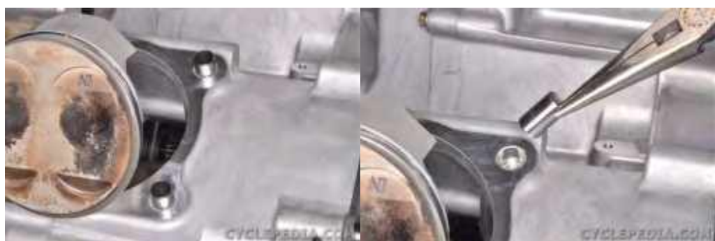
Remove the two dowel pins.
