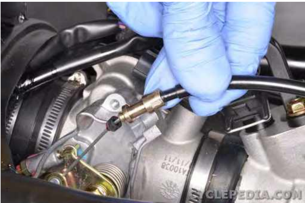
Slide the throttle cable housing out of the throttle body.
