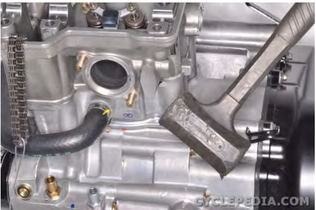
Tap the reinforced areas of the cylinder head with a rubber mallet to free the dowel pins.
