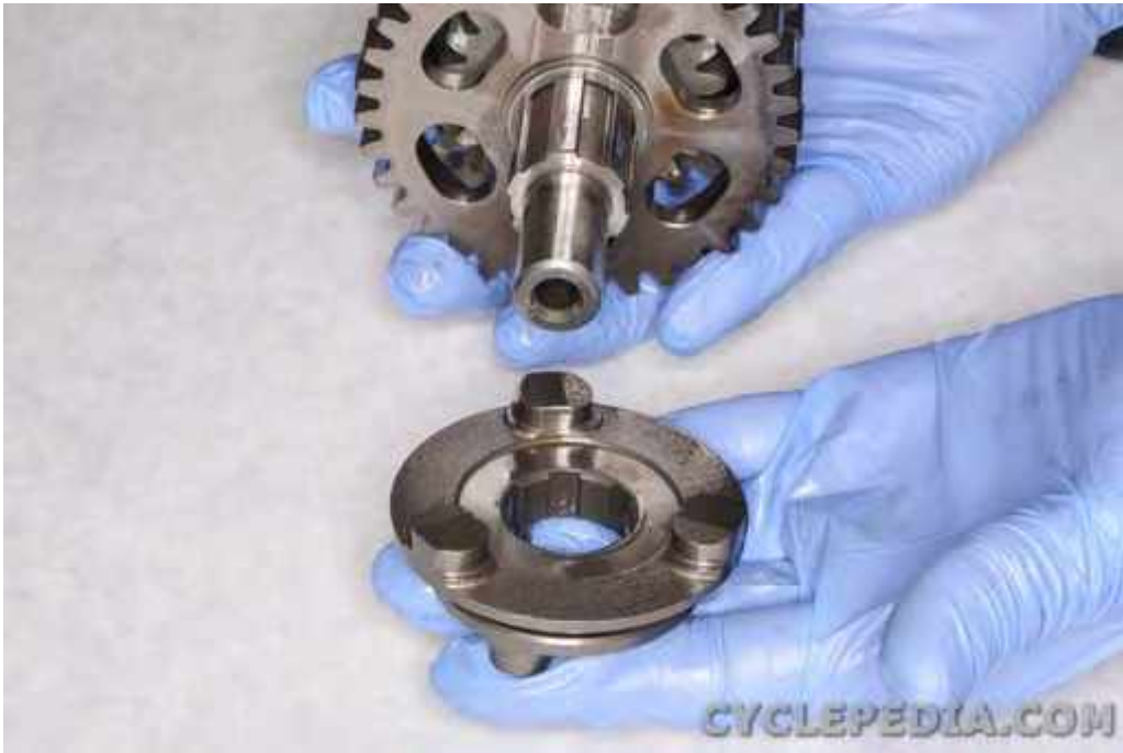
Remove the high/low gear shifter.
