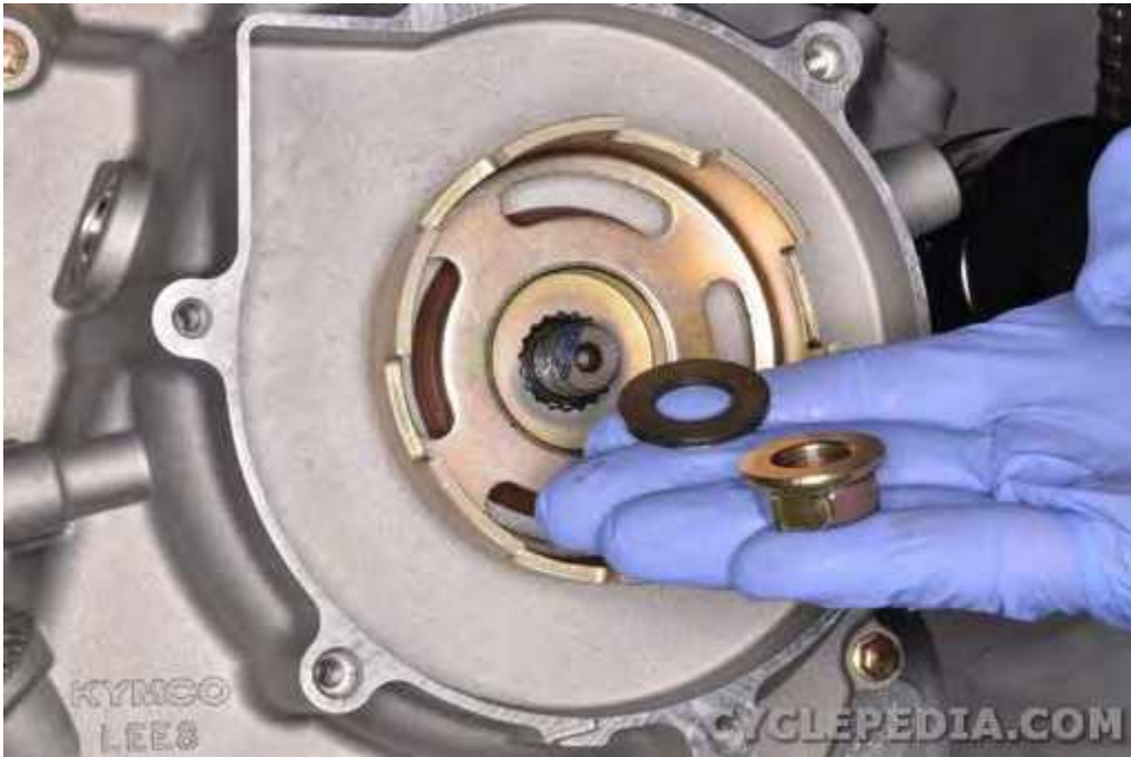
Remove the recoil starter nut and washer.
