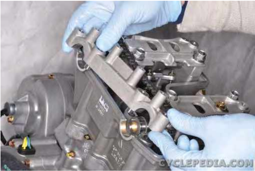
Fit the cam chain side camshaft holder into place.
