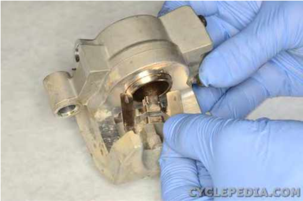
Install the brake pad spring.
