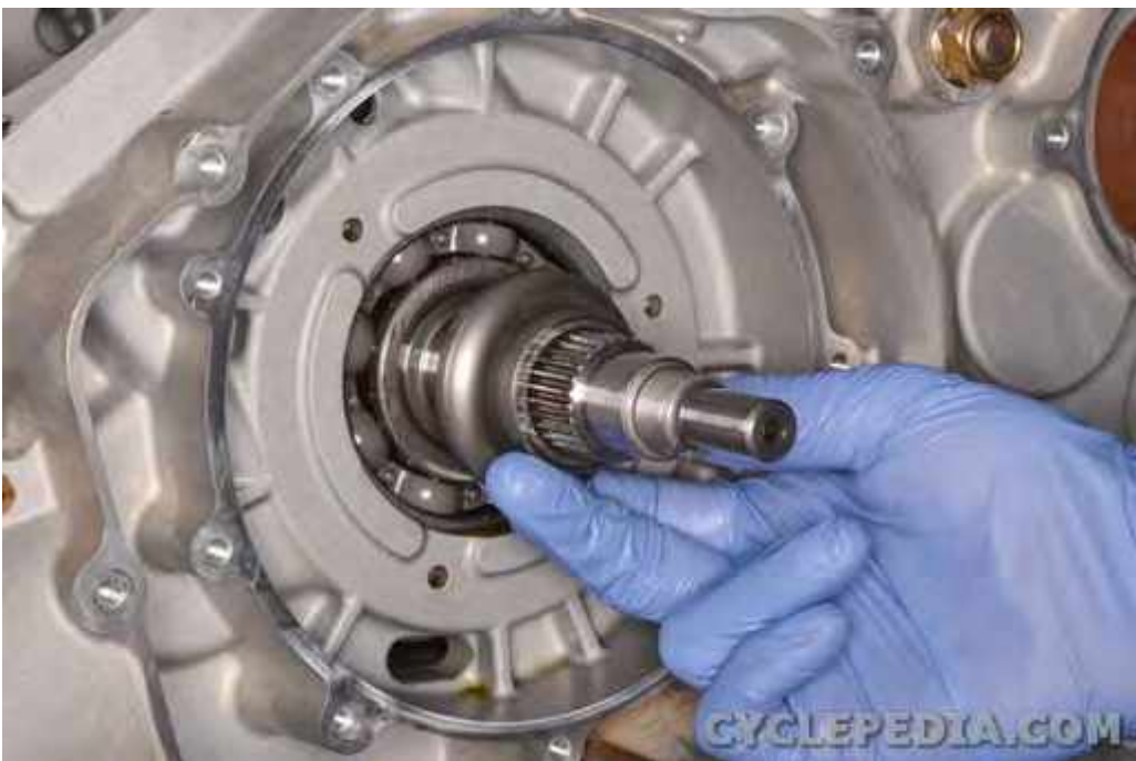
Slide off the inner clutch collar.
