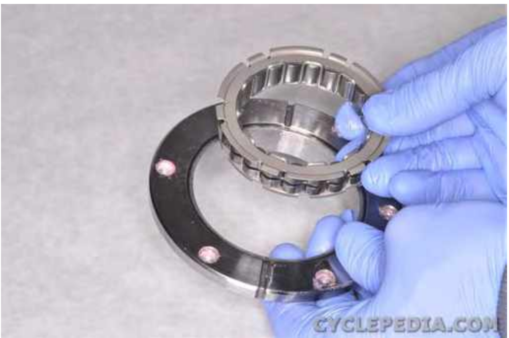
Remove the starter clutch from the mounting plate.
