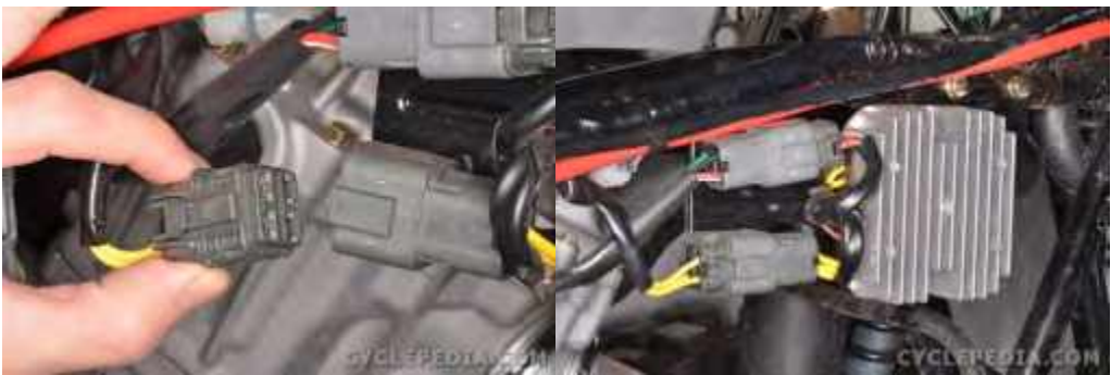
Plug in the 4-pin stator connector.
