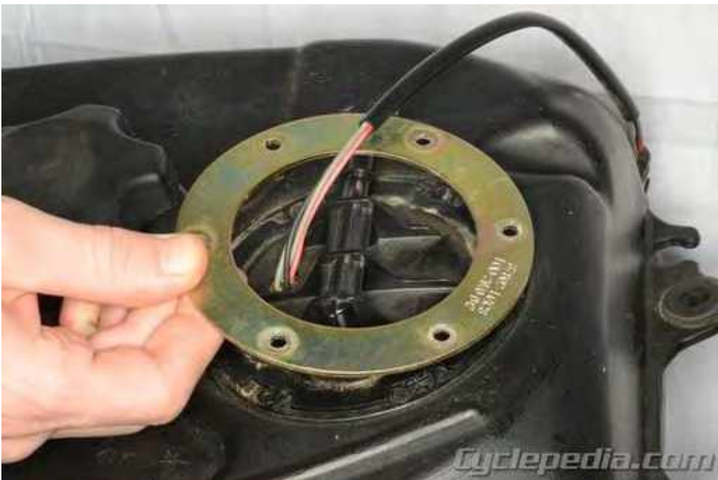
Install the fuel pump mounting ring.
