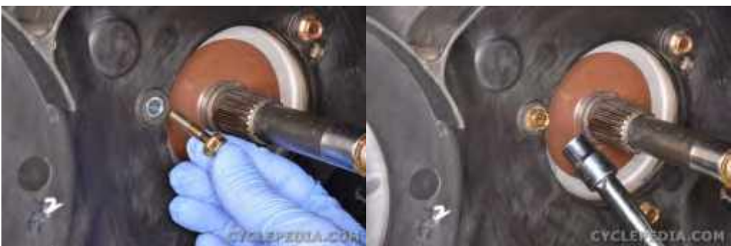
Install the inner belt case bolts and tighten them securely with a 10 mm socket.
