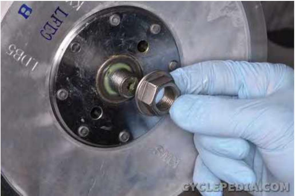
Remove the driven pulley nut.
