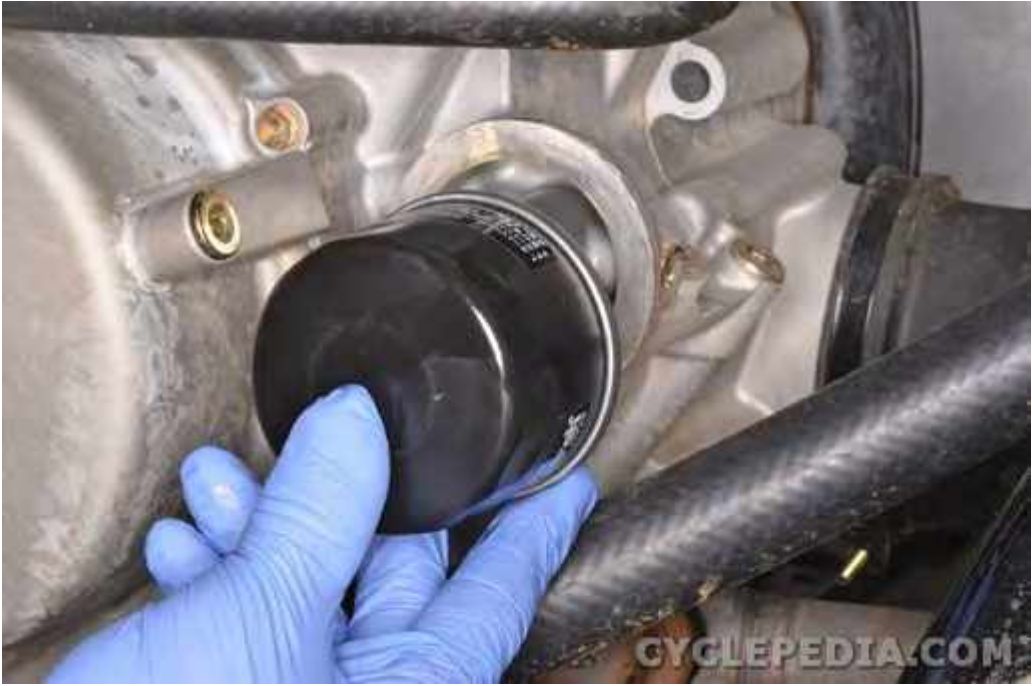
Remove the oil filter cartridge.
