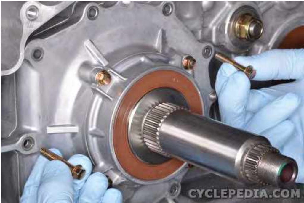
Remove the clutch cover bolts.
