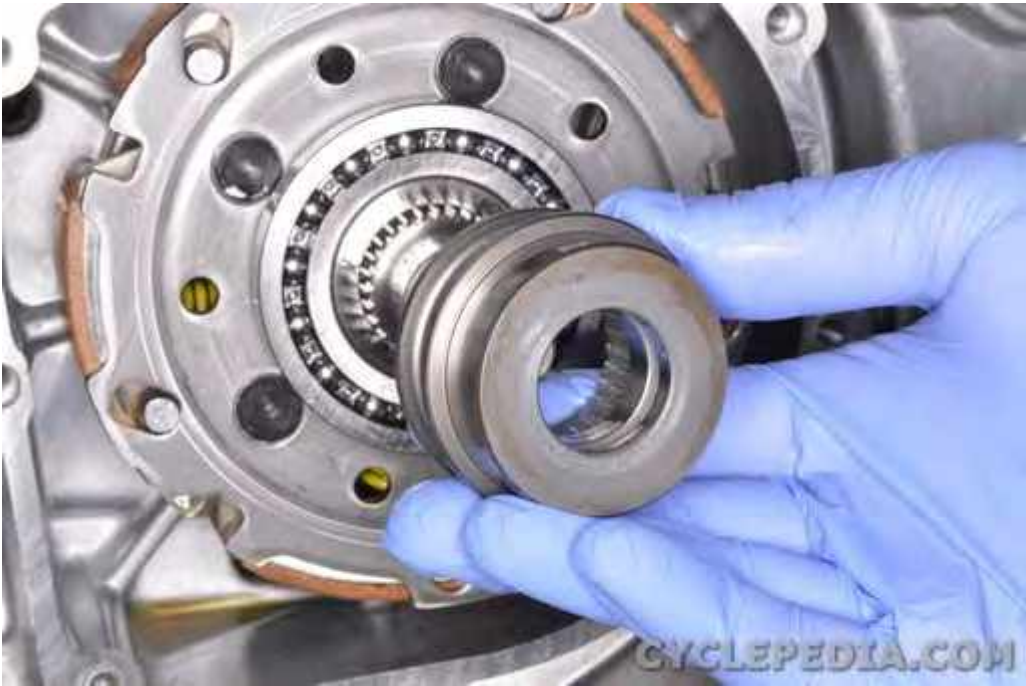
Slide off the outer clutch collar.
