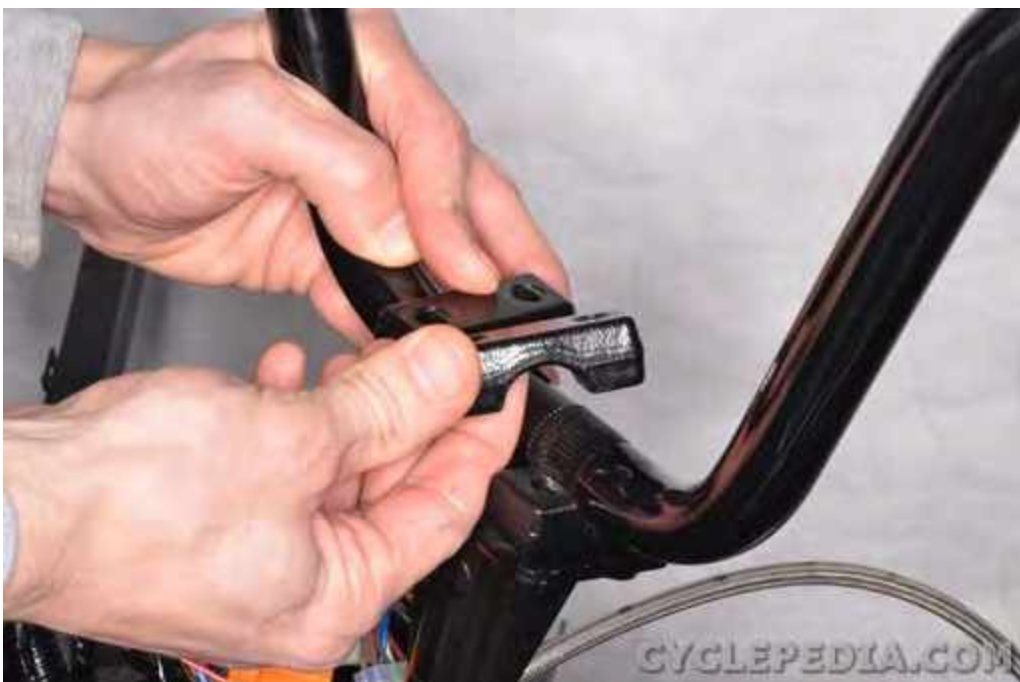
Lift off the handlebar clamps.
