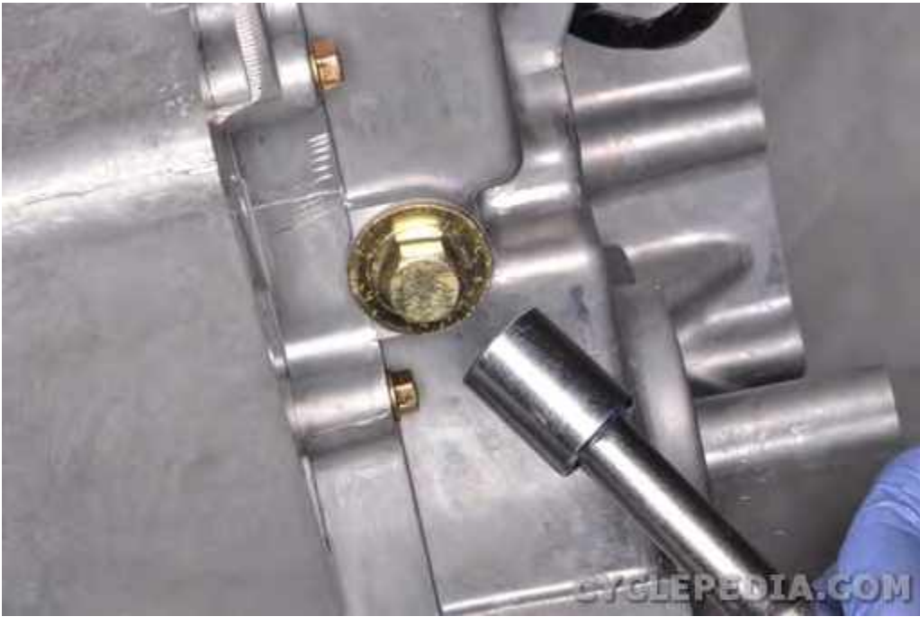
Loosen the shift cam stopper plug with a 14 mm socket.
