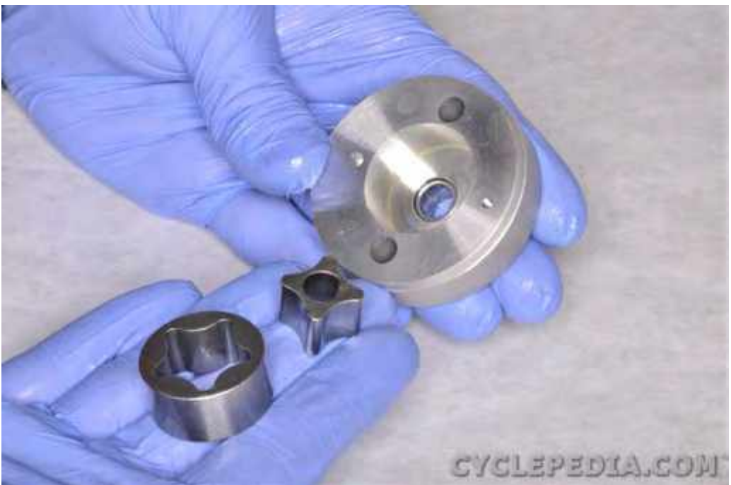
Remove the inner and outer oil pump rotors.
