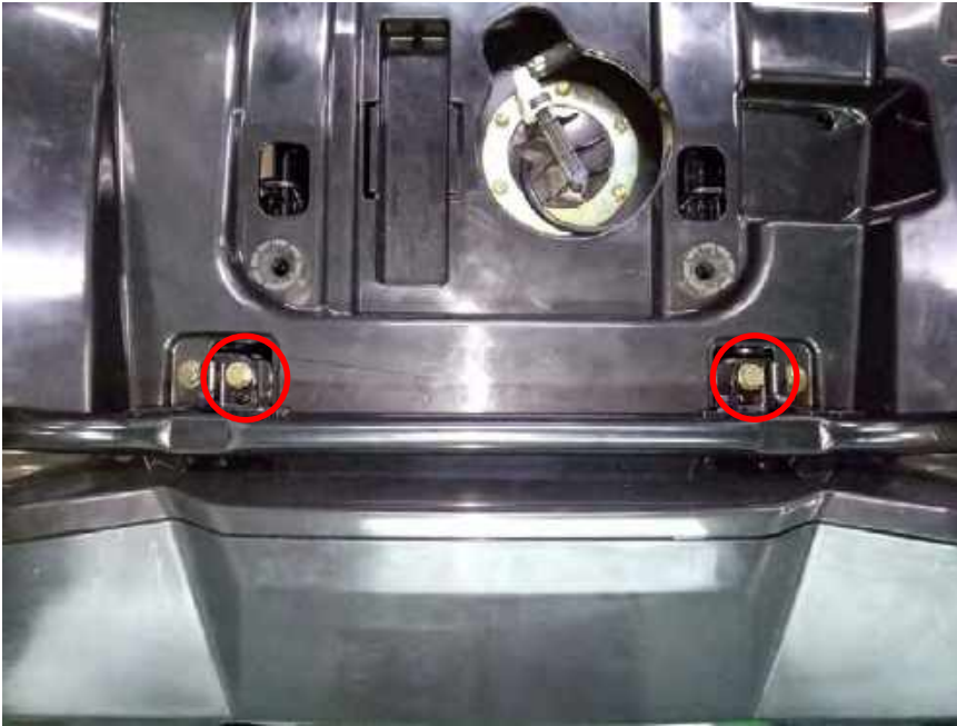
Remove the rear rack support pipe with two bolts
