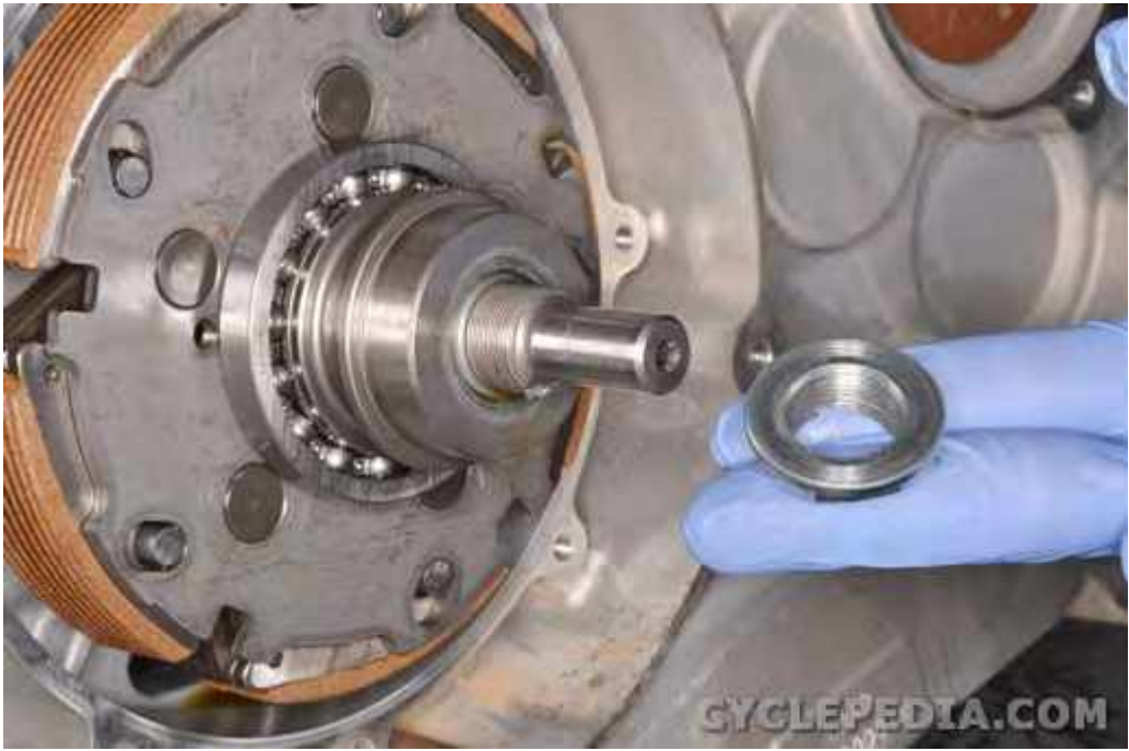
Thread on a new clutch lock nut.
