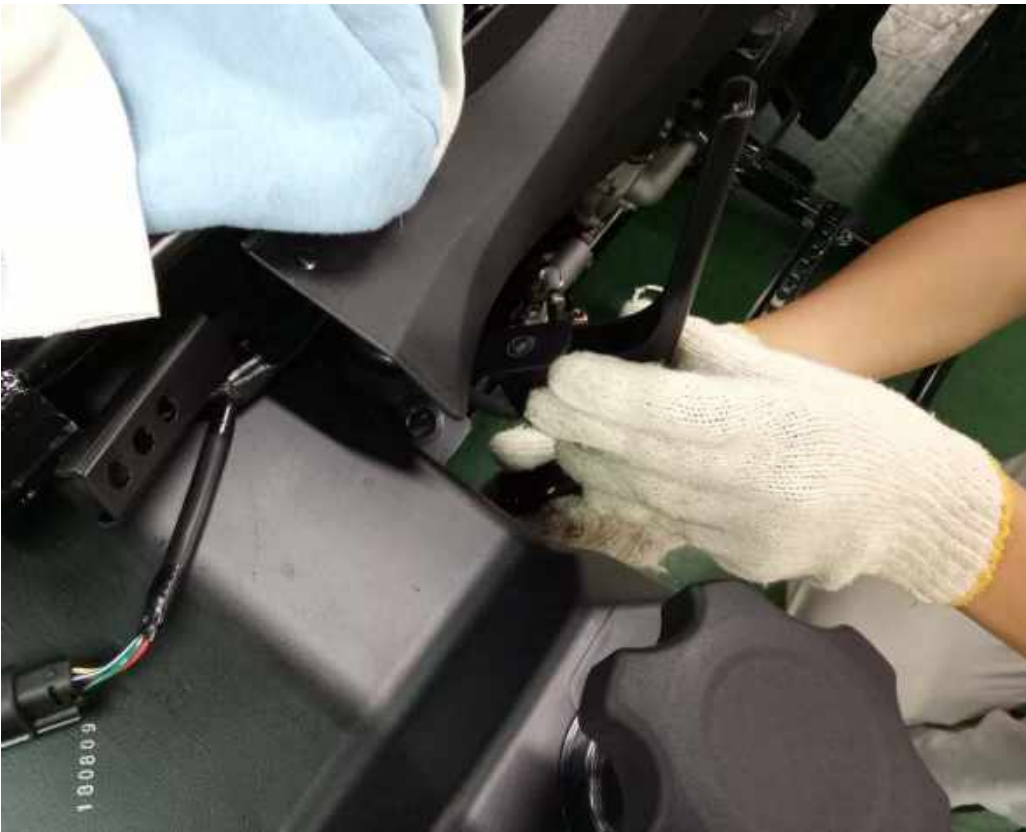
Remove the fuel tank front pipe.
