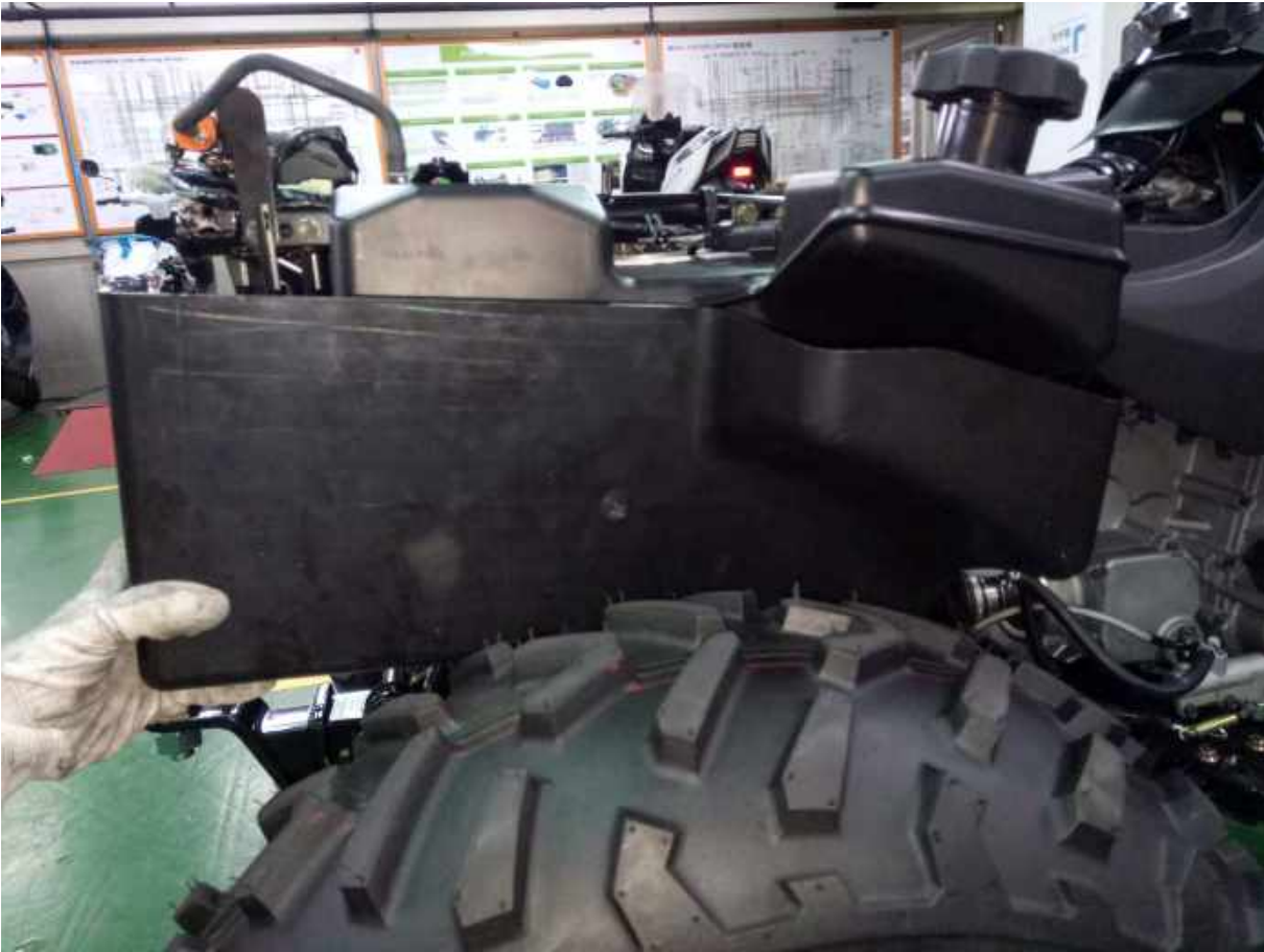
Remove the fuel tank protector cover.
