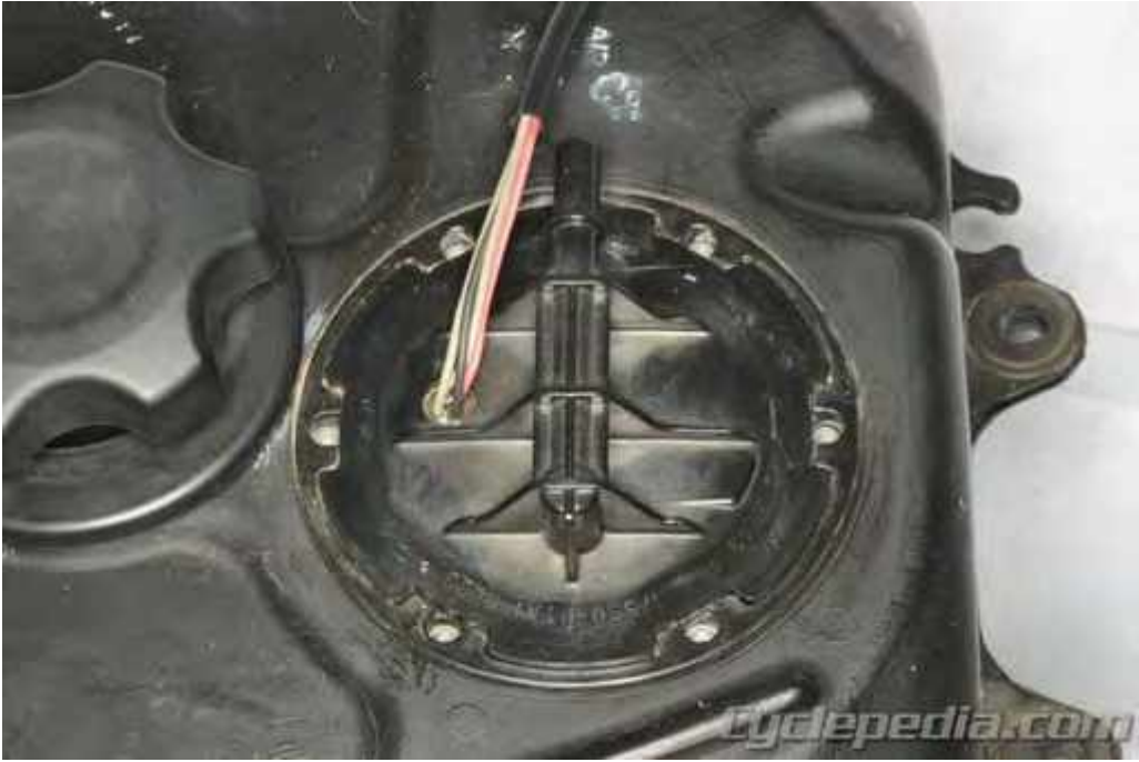
Position the fuel delivery pipe as shown.
