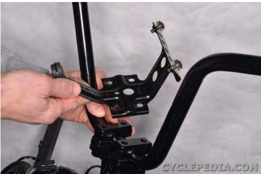
Set the instrument bracket into place.
