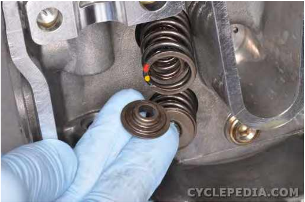
Remove the spring retainers.
