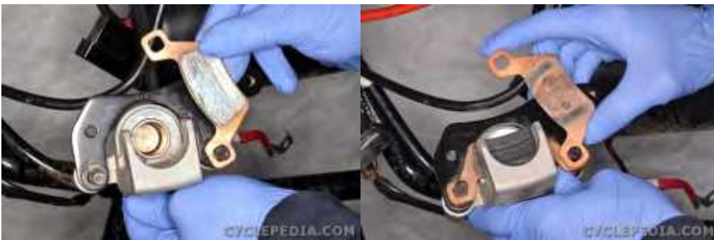
Install the brake pads.
