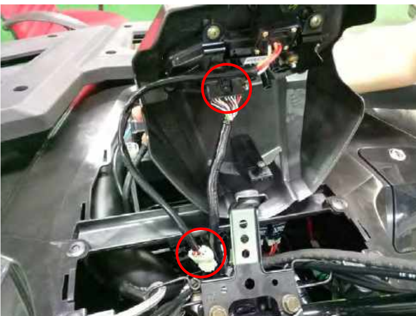
Plug the connector into the back of the instrument display.
