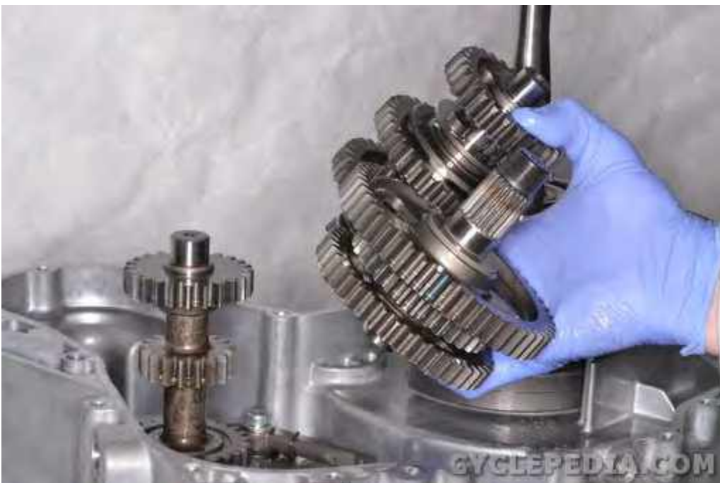
Remove the transmission shafts together from the crankcase.
