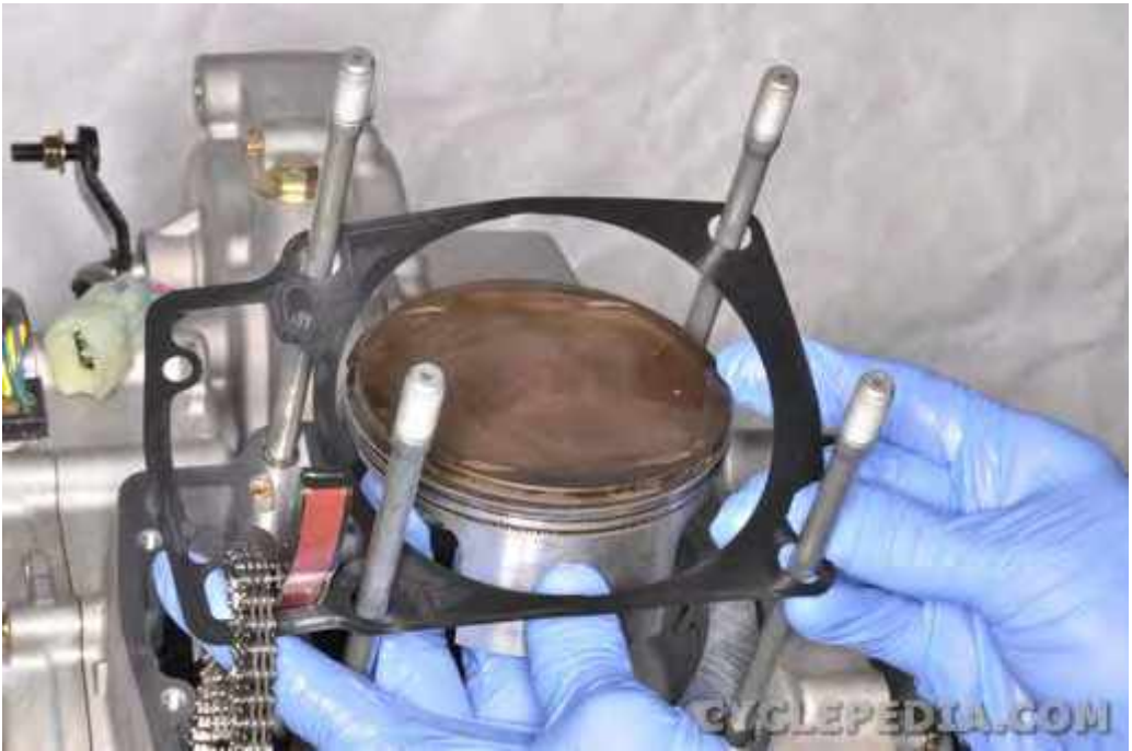
Lift off the base gasket.
