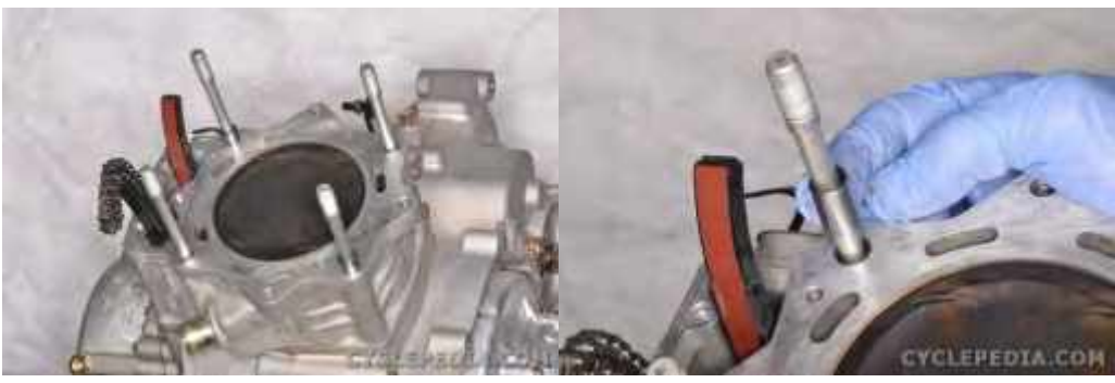
Remove the two cylinder head dowel pins.
