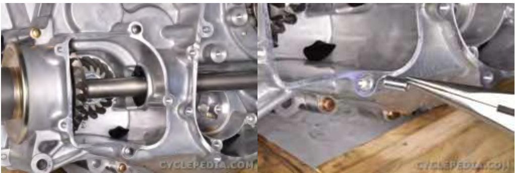
Remove the gasket and the two bevel gear cover dowel pins.
