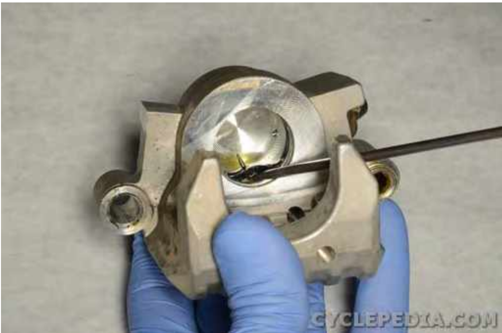
Use a mechanics pick to remove the piston seal from the inner caliper bore and discard.
