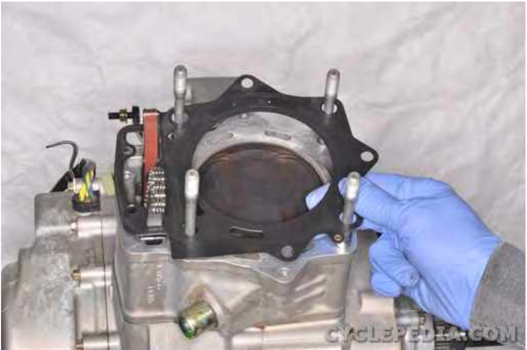
Remove the cylinder head gasket.
