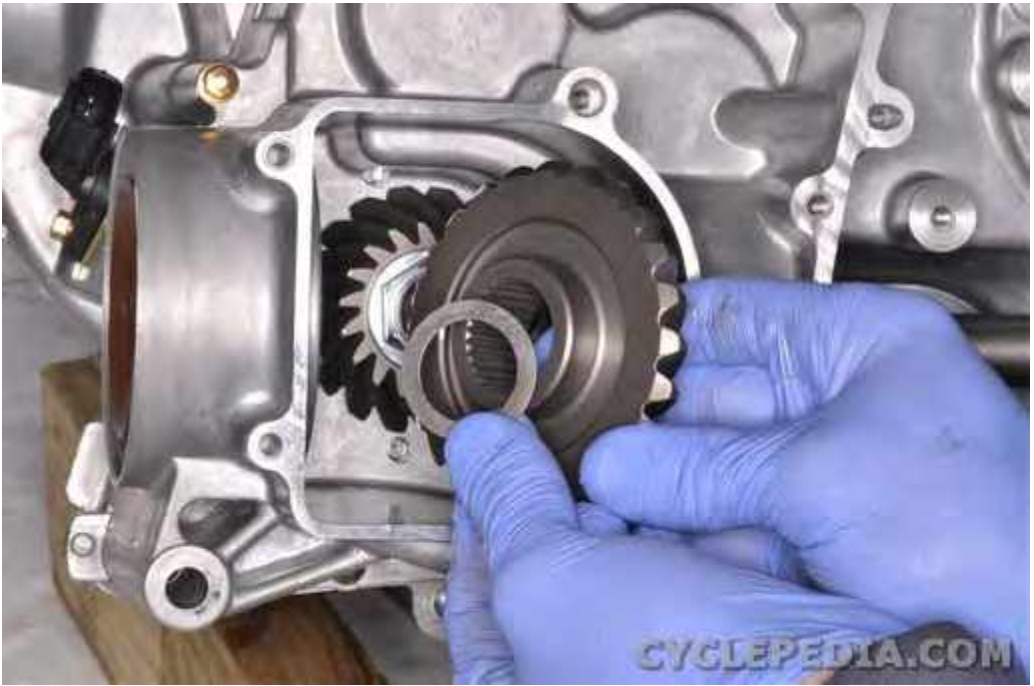
Fit the driven bevel gear and shim into place.
