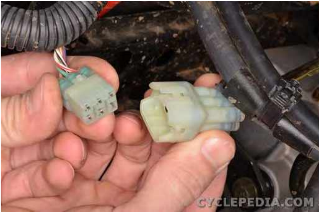
Plug in the gear position switch connector.
