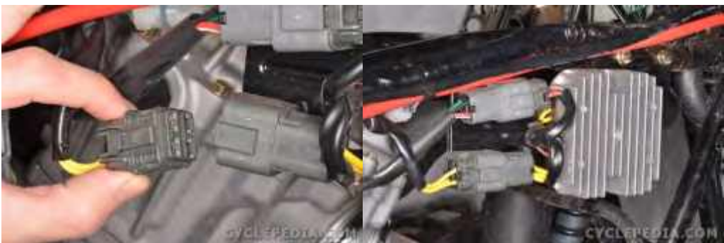
Plug in the 4-pin stator connector.
