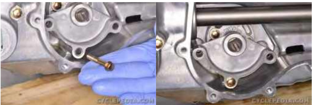
Install the oil pump shaft holder bolt. Do not tighten, yet.
