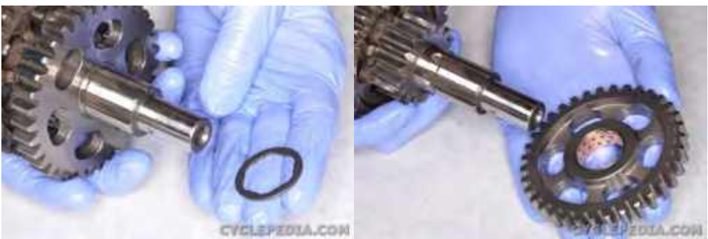
Remove the washer and low drive gear.
