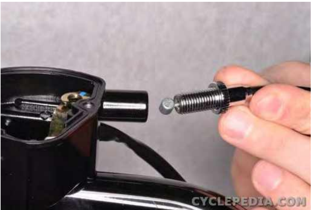
Unscrew the throttle cable from the throttle housing.
