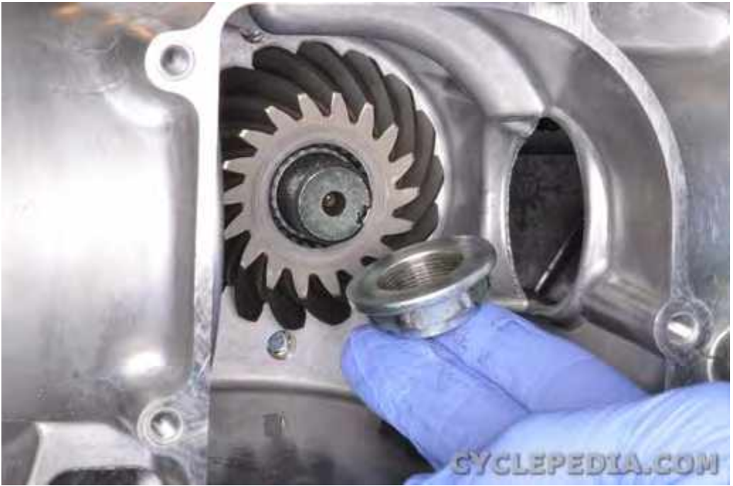
Remove the drive bevel gear nut.
