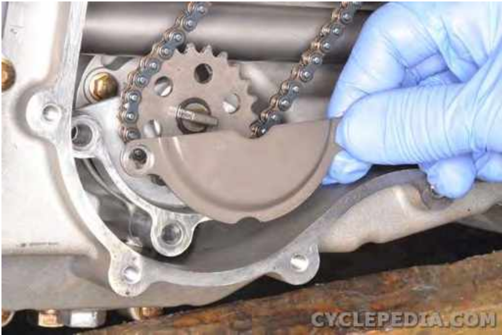
Remove the oil pump cover.
