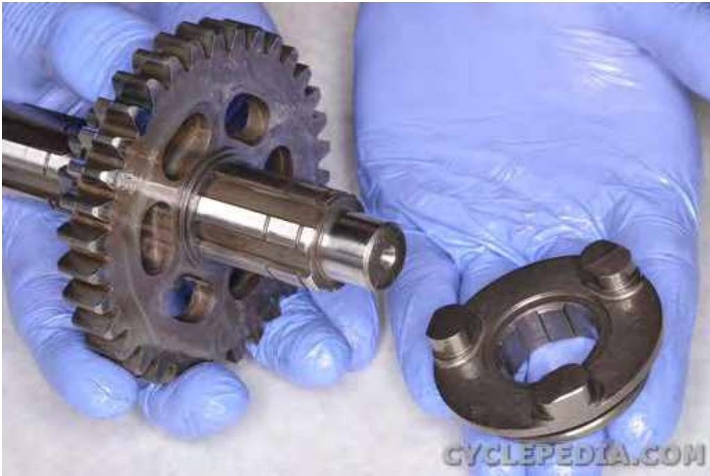
Remove the reverse gear shifter.
