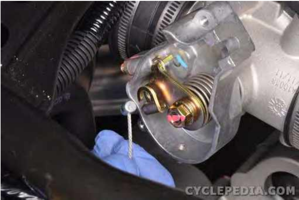
Free the throttle cable from the throttle drum.
