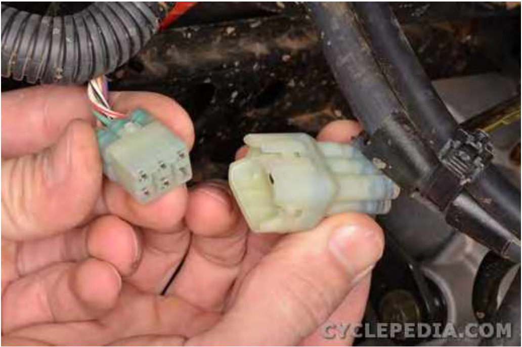
Plug in the gear position switch connector.
