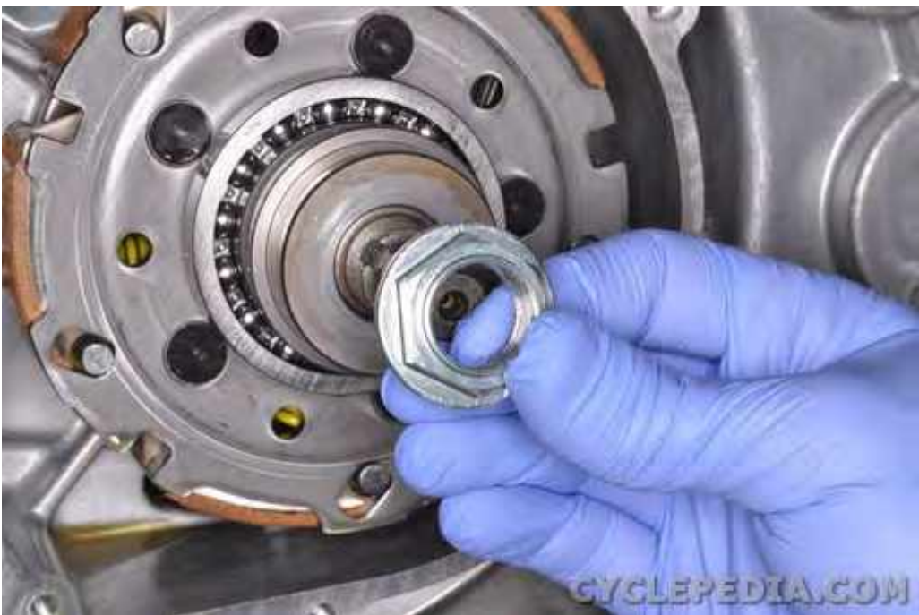
Thread on a new clutch lock nut.
