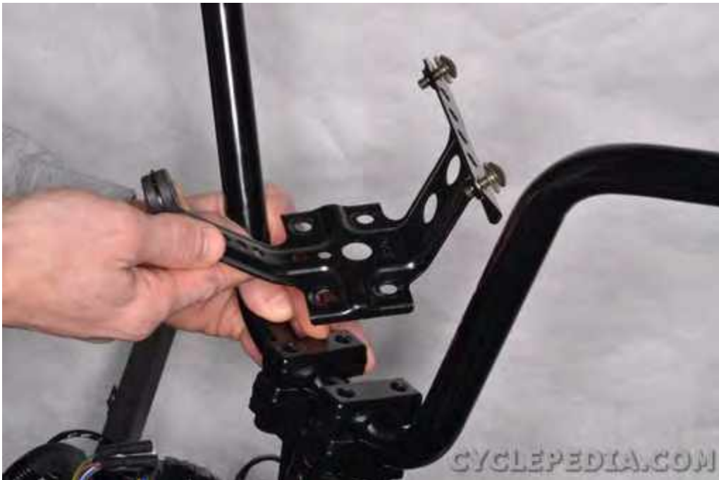
Lift off the instrument bracket.
