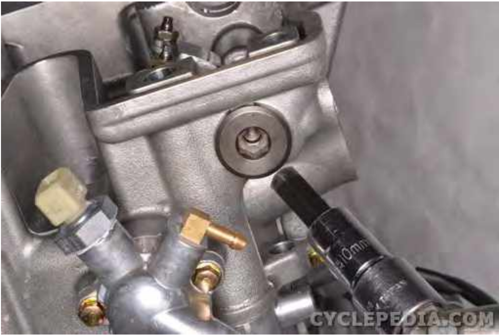
Loosen the rocker arm shafts with a 10 mm Allen.
