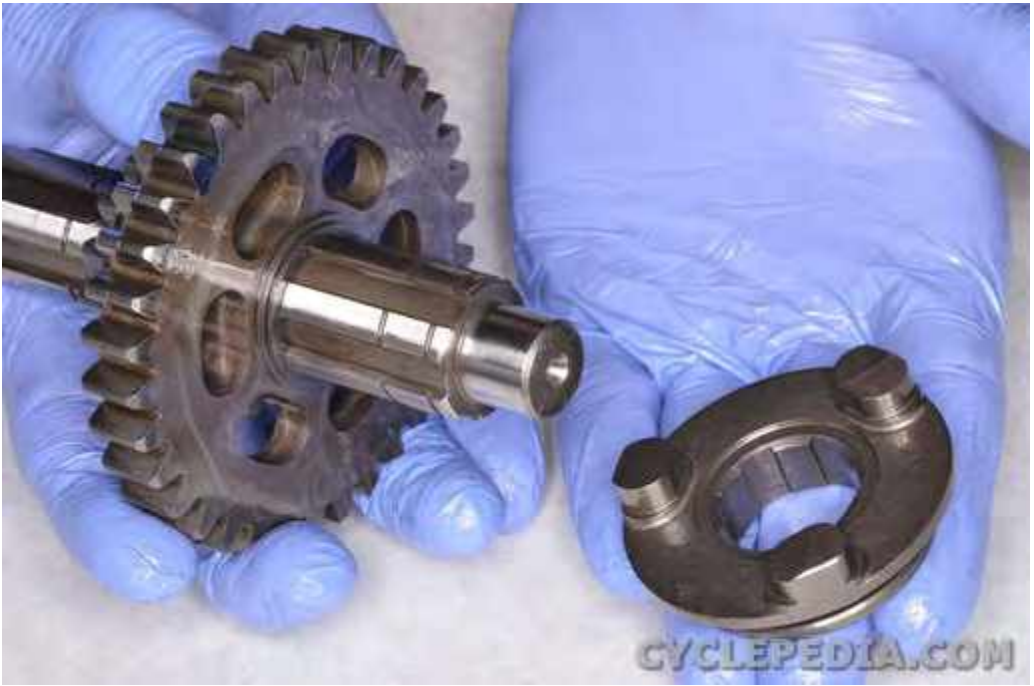
Remove the reverse gear shifter.
