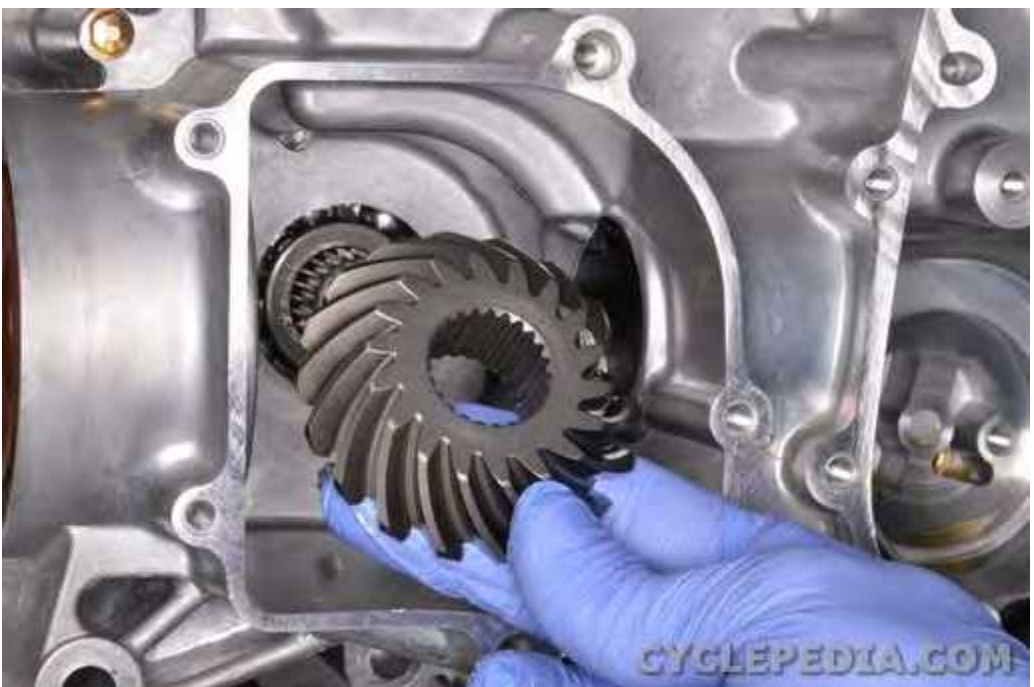
Slide off the drive bevel gear.
