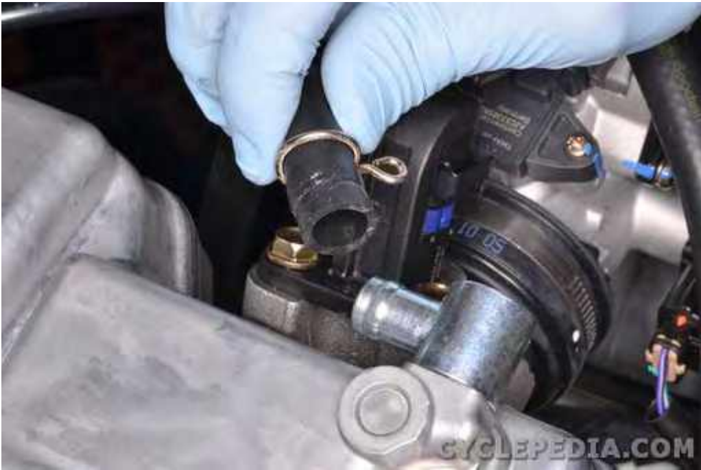
Disconnect the crankcase breather hose from the cylinder head cover on the MXU 500i models.
