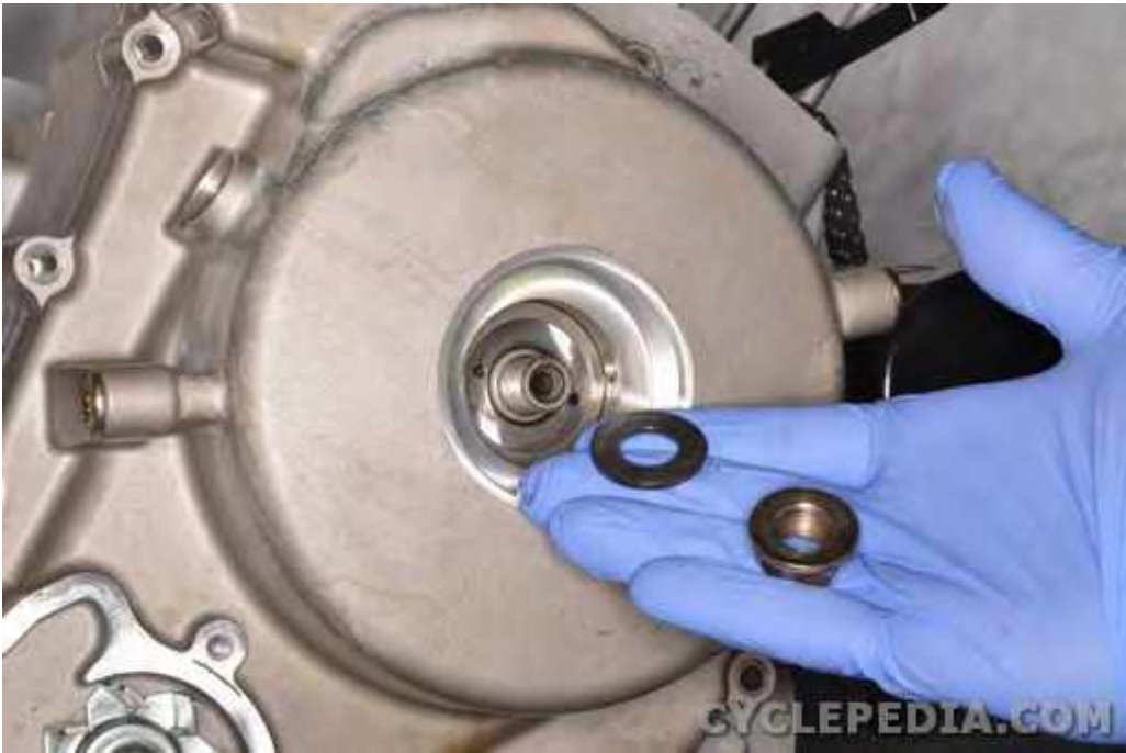
Place the washer on the crankshaft and thread on the nut.
