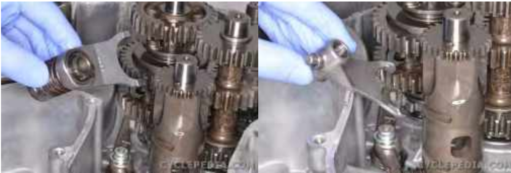
Remove the upper and lower shift forks.
