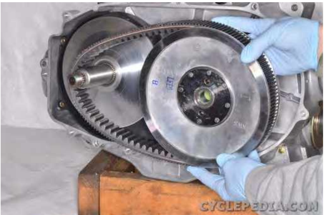
Remove the driven pulley and CVT belt.
