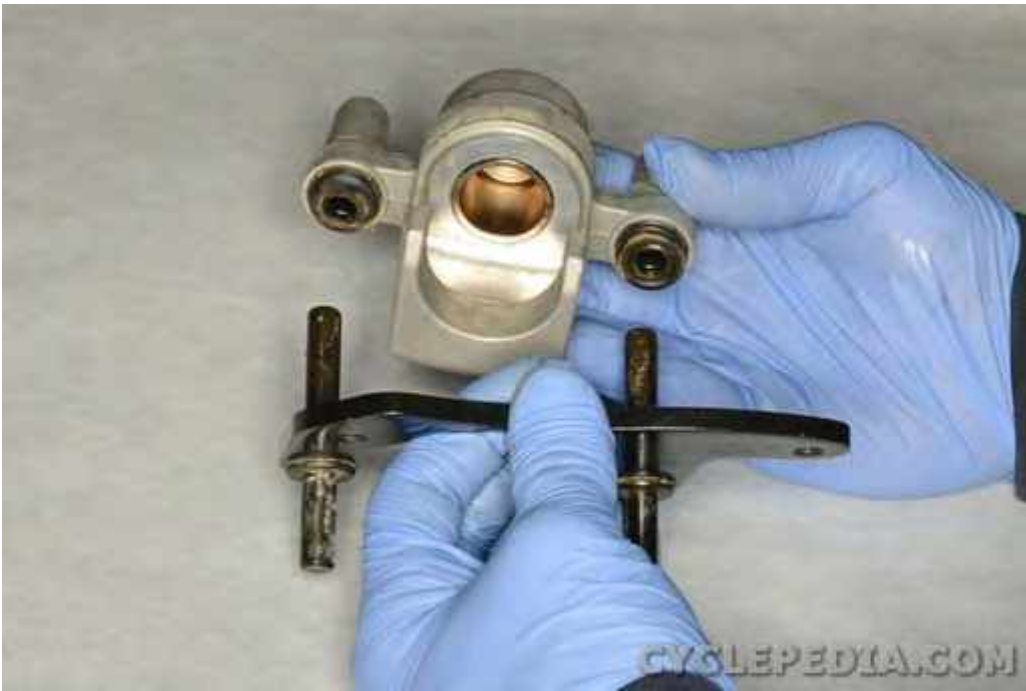
Apply silicone grease to the caliper bracket pins. Install the caliper bracket.
