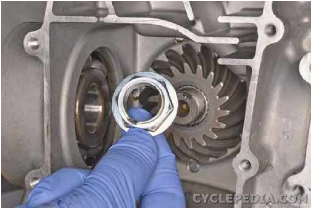
Remove the drive bevel gear nut.
