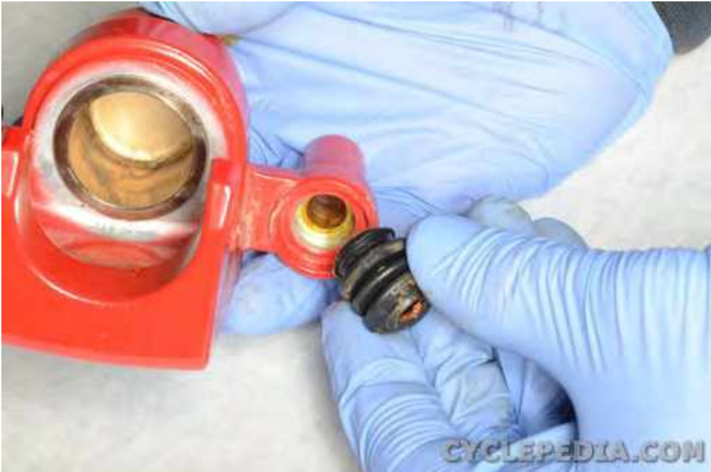
Install the pin boots into the caliper.
