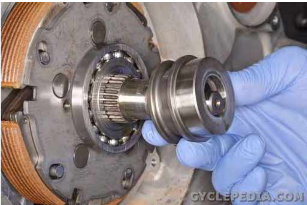
Slide off the outer clutch collar.
