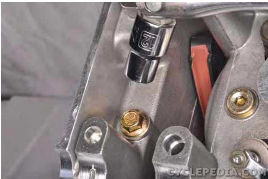
The cylinder head bolt is number 9.
