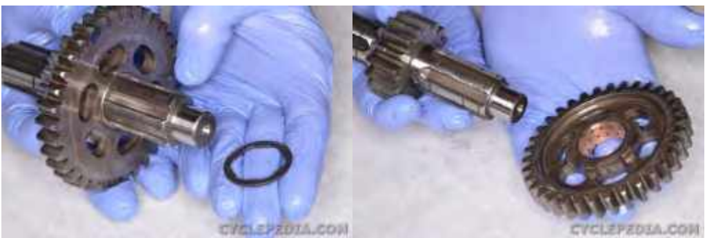
Remove the washer and reverse drive gear.
