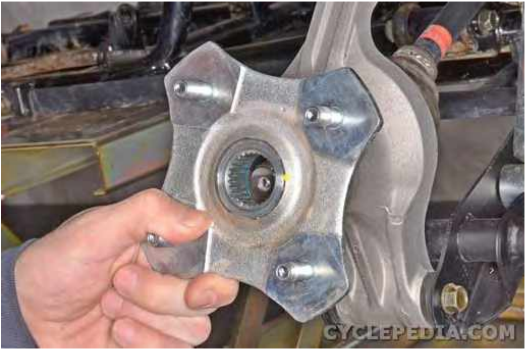
Slide on the wheel hub assembly.
