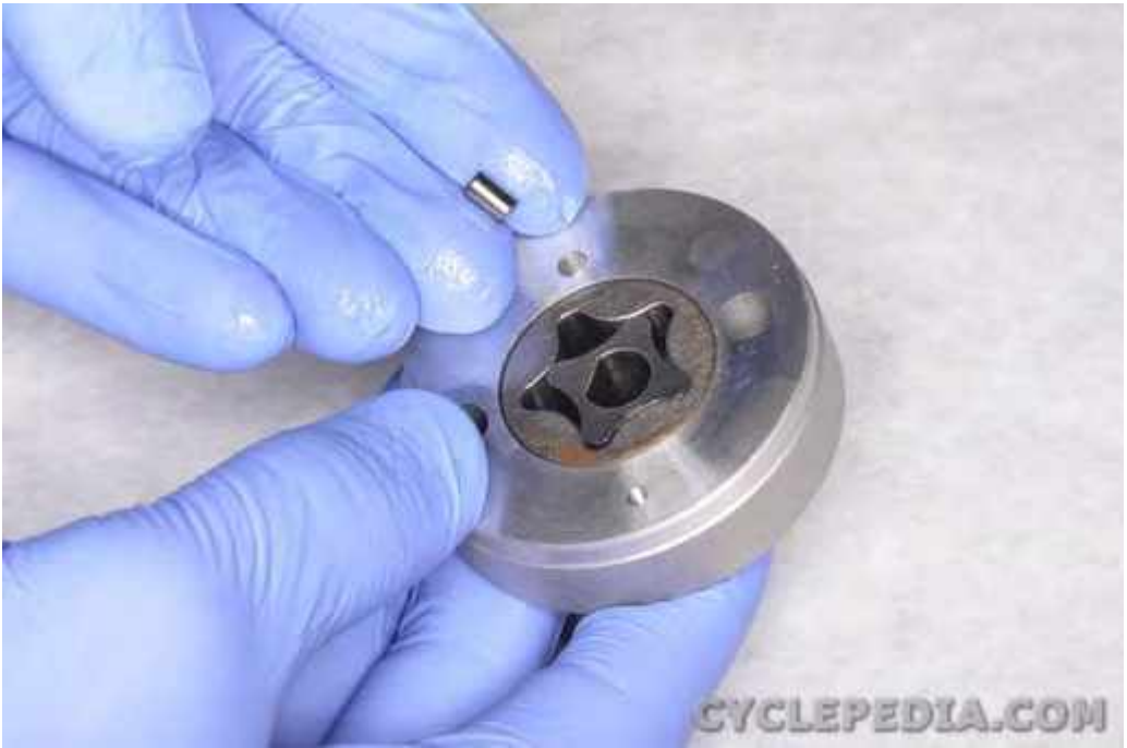
Remove the oil pump dowel pin.
