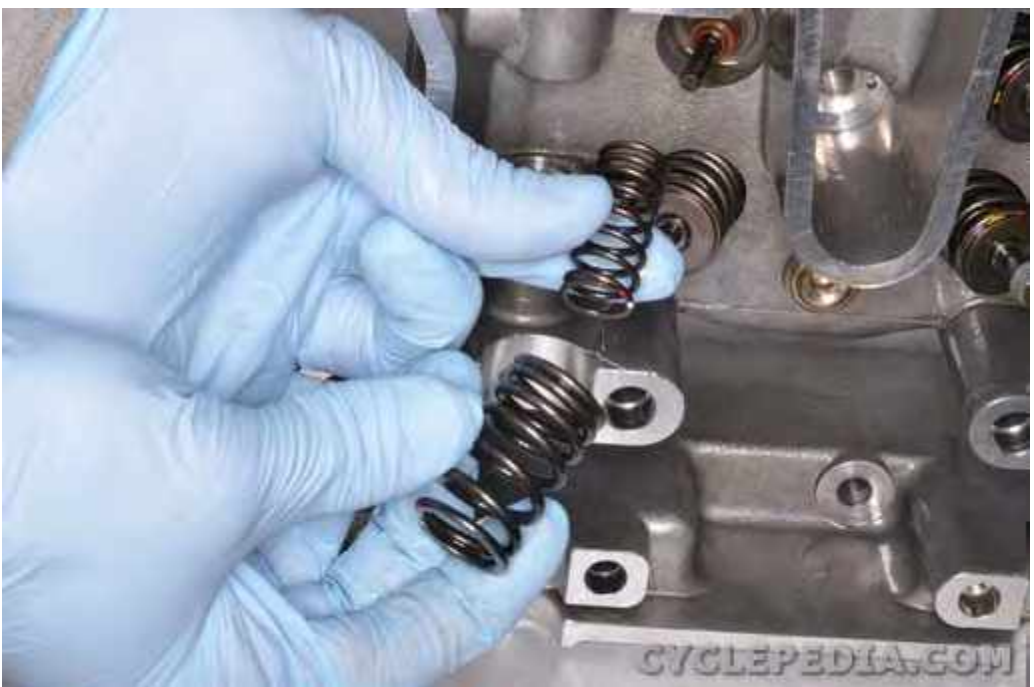
Lift out the valve springs.
