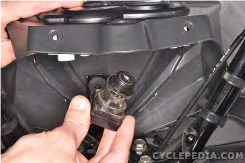
Fit the main switch into the instrument cover.
