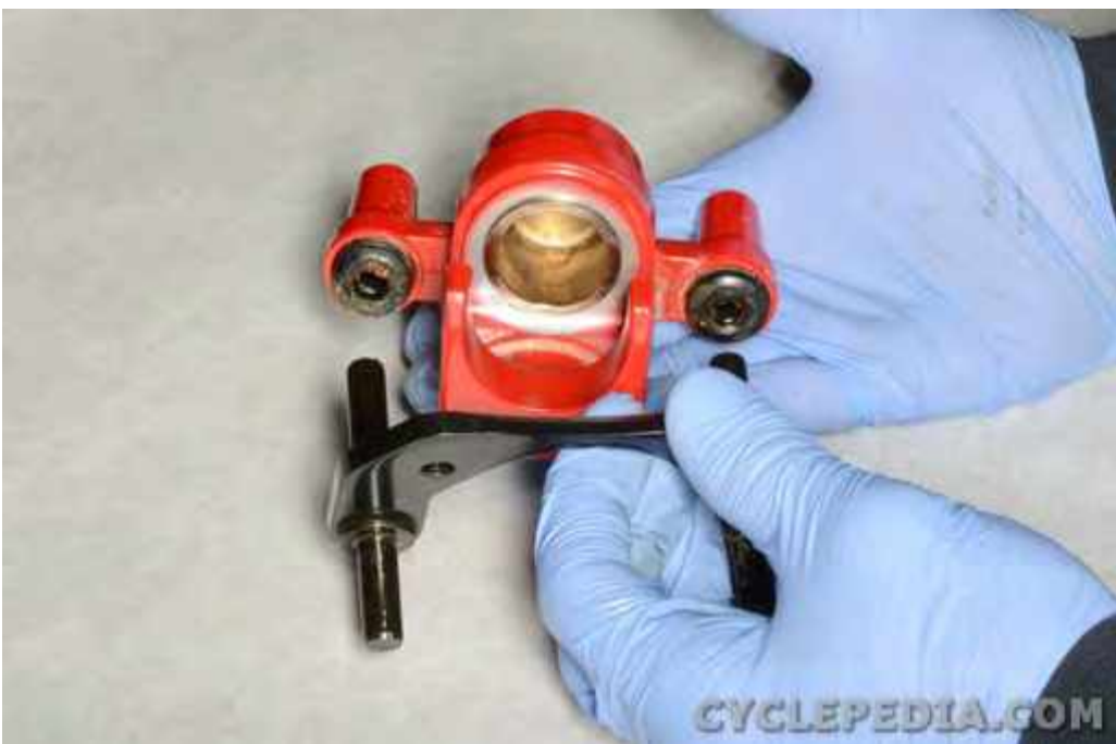
Apply silicone grease to the caliper bracket pins. Install the caliper bracket.
