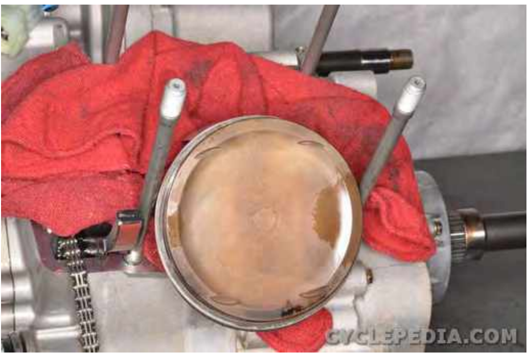
Remove the two dowel pins.
