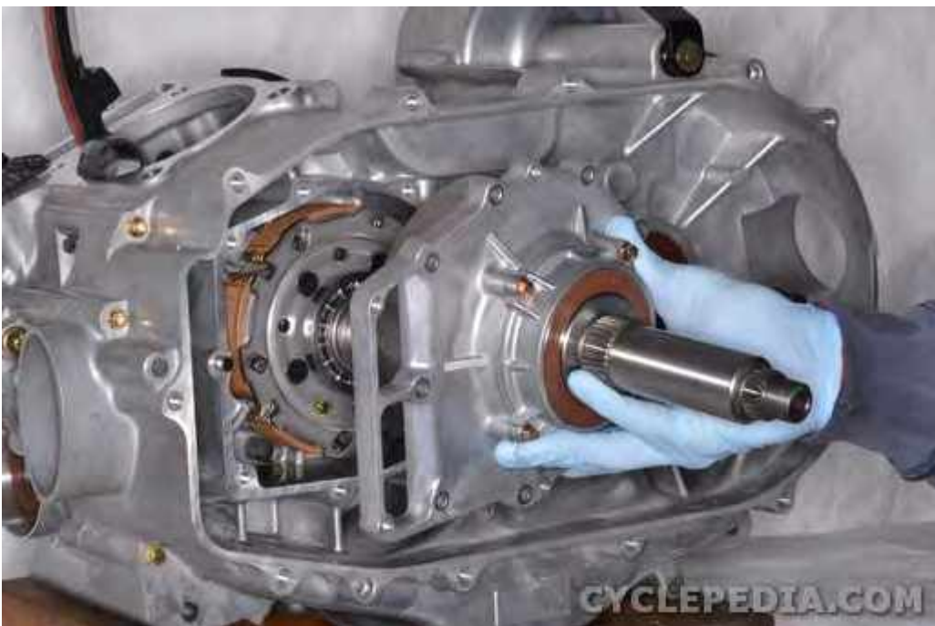
Remove the clutch cover assembly evenly.
