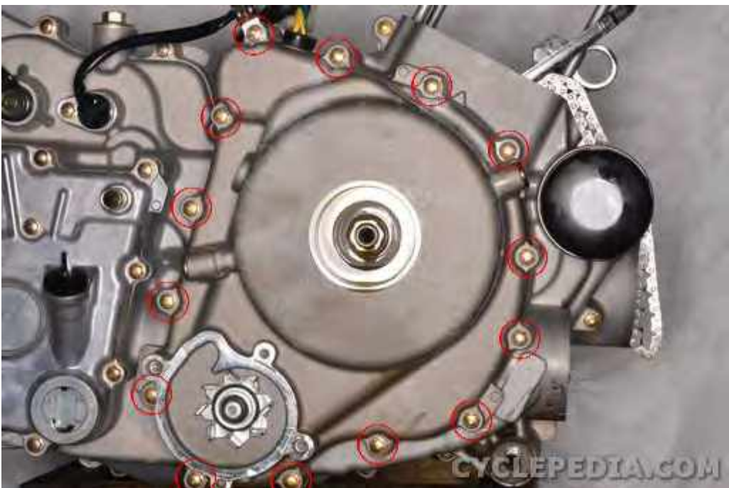
Thread in the generator cover bolts. Install the wire clamp with the top bolt.
