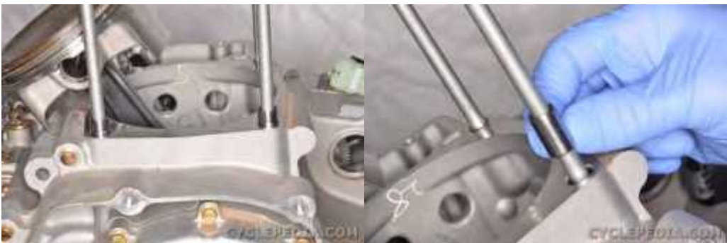
Remove the two dowel pins.
