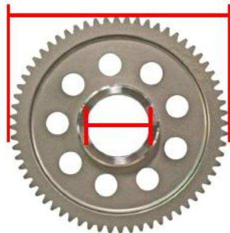
Inspect the starter driven gear for wear and damage. Measure the inside and outside diameter of the starter driven gear and replace if needed.
