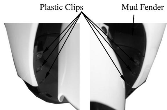
Remove 2 plastic fasteners beneath the handlebar cover.(turn the handlebar to the left end and right end,you will see them)
