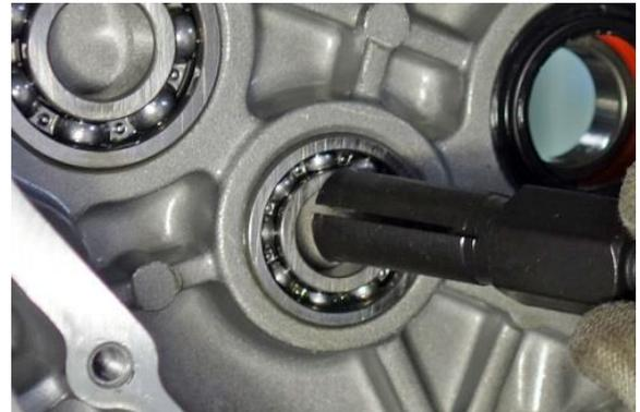
Use a bearing puller to remove the crankcase or transmission cover.
