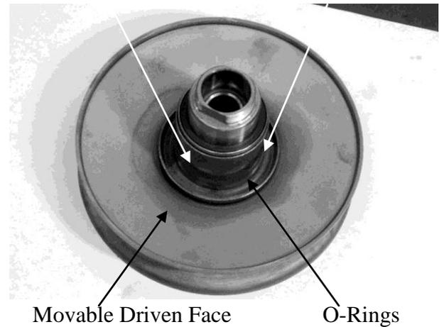
Remove the O-rings and oil seal from the movable driven face.
