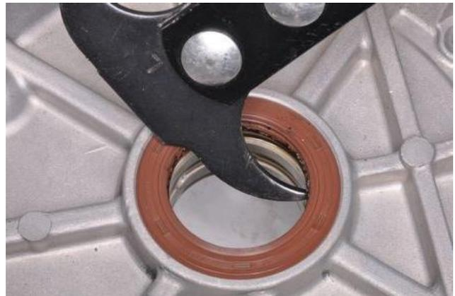
Drive a new seal into the left crankcase from outside with a suitable driver, which should have the same outside diameter with the seal.
