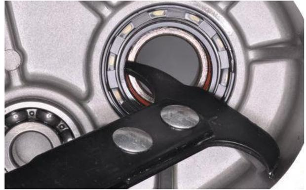
Use a bearing driver to install any new bearings into the crankcase and transmission Case cover. The driver should have the same Outside diameter as the bearings. The bearings should go in square and have their marking facing out. Drive in a new seal in the same way if needed.
