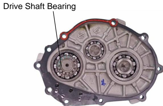
Check the transmission cover bearings for excessive play. Inspect the drive shaft, drive shaft bearing and oil seal for wear or damage.
