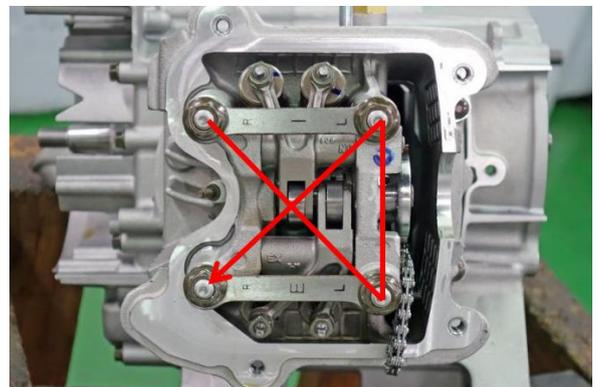
Remove the 2 camshaft holders.
