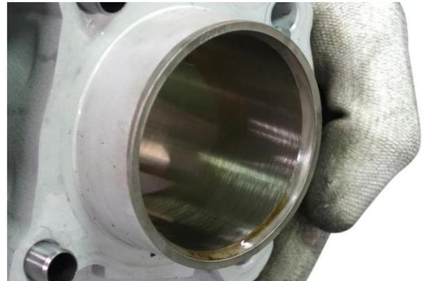
Measure the cylinder diameter as below with a telescoping gauge.
