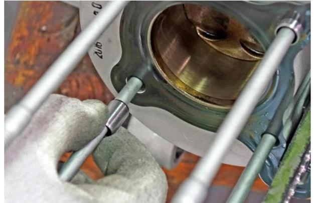
Remove the intake plate and gasket from the cylinder head.
