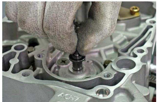
Remove the 2 oil pump screws with a #3 philips screwdriver.
