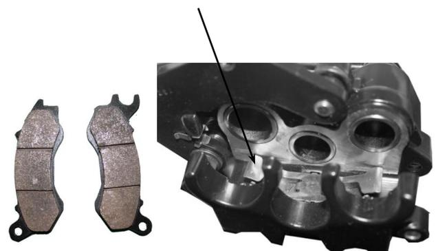
Install the brake pads in the reverse order of removal.
