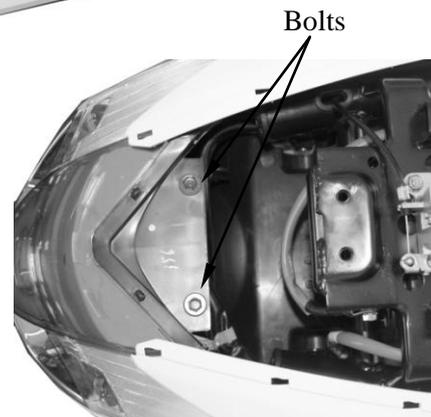
Remove 2 plastic fasteners attaching the frame body cover.
