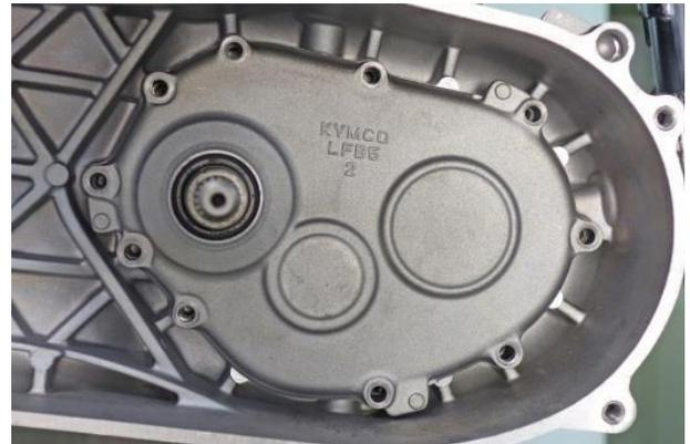
Insert the 10 transmission case cover bolts. Tighten the bolts to specification using a 8mm socket.
