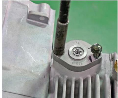
**Rotate the crankshaft 360° clockwise and check the engine timing one more time.**
