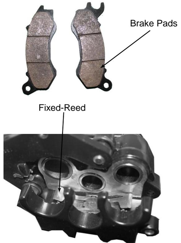
Wipe off excessive brake fluid with a clean shop towel. Apply silicon grease to the brake caliper seat pin and caliper inside. Install the brake caliper seat.
