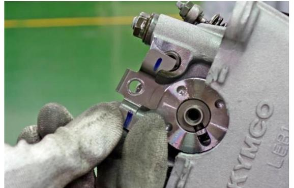
Remove the 4 camshaft holder nuts with
