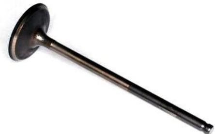
Inspect the valve for burning and damage.
