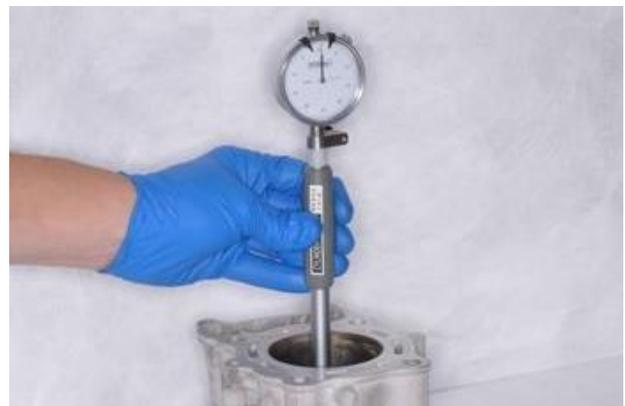
Inspect the cylinder front to back and side to side at three different height levels with a dial bore gauge. Replace the cylinder and piston as a set if the cylinder is out of specification.
