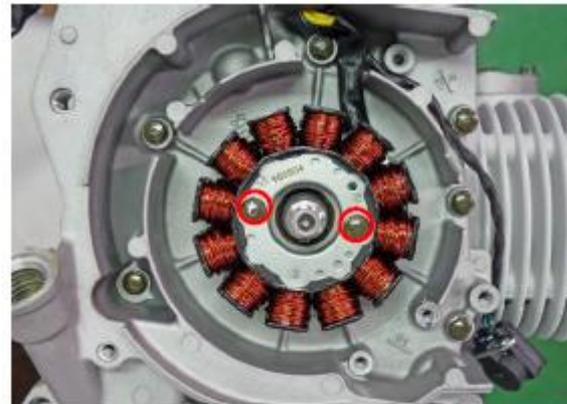
Remove the 3 stator mounting bolts and the 2 crank position sensor bolts with an 8mm socket. Remove the stator and the crank position sensor together.
