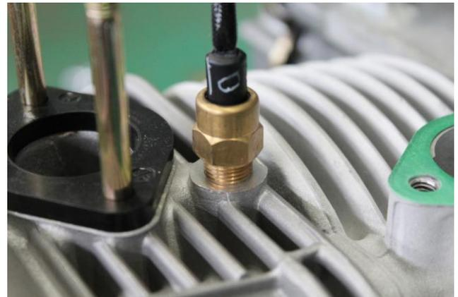
remove the engine temperature sensor if needed.
