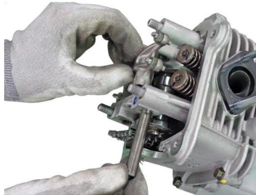
Remove the camshaft from the cylinder head.
