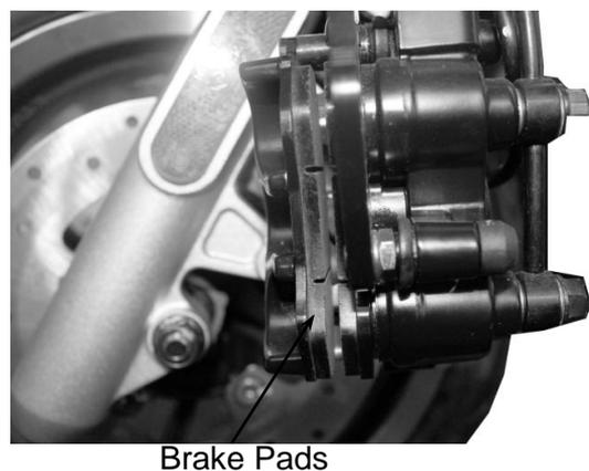
Remove the pistons from the brake caliper. If necessary, use compressed air to squeeze out the pistons through the brake fluid inlet opening and place a shop towel under the caliper to avoid contamination caused by the removed pistons. Check each piston cylinder for scratches or wear and replace if necessary.
