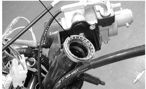
Apply grease to the ball races and install the front fork.
