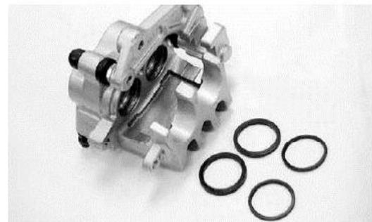
Check the piston for scratches or wear.
