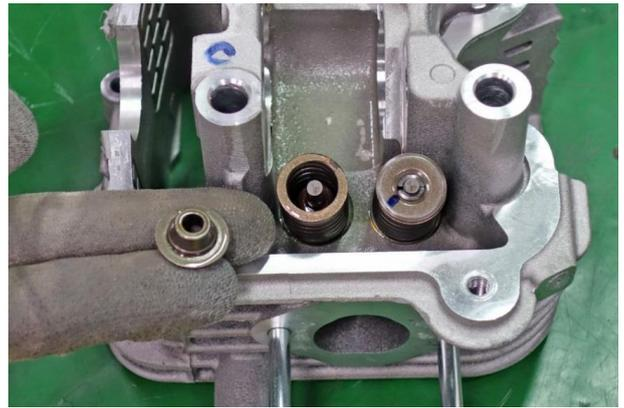
Remove the valve springs.
