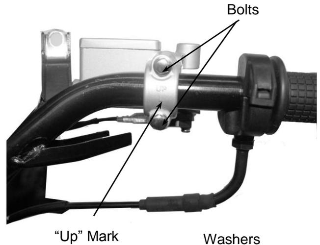
Install the brake fluid tube with the attaching bolt and two sealing washers.
