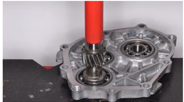
Insert the final shaft through the oil seal and bearing.
