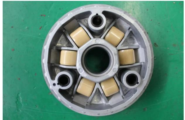
Check the drive pulley collar for wear or damage. Measure the O.D. of the drive pulley collar sliding surface.
