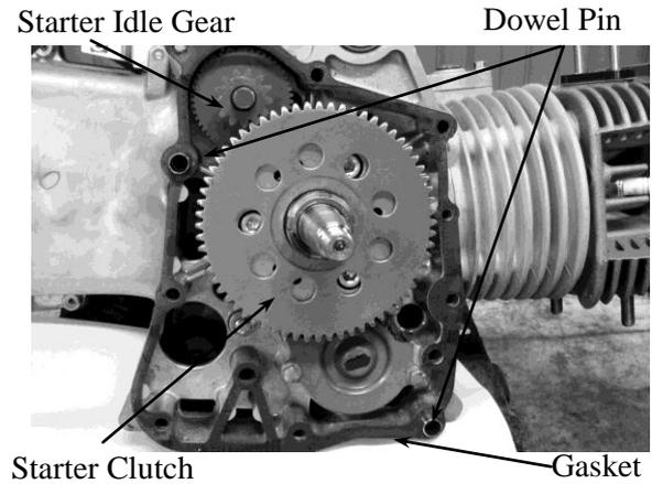
Install the right crankcase cover and tighten the nine bolts.
