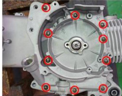
Use the special tool to remove the nut.
