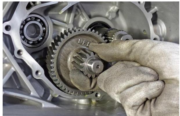
Install the final gear onto the final shaft as shown.
