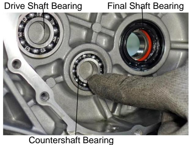
Check the transmission case cover bearings for excessive play and inspect the final shaft bearing oil seal for wear or damage.
