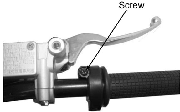
Remove the throttle seat from the handlebar and disconnect the throttle cable from the throttle pipe.
