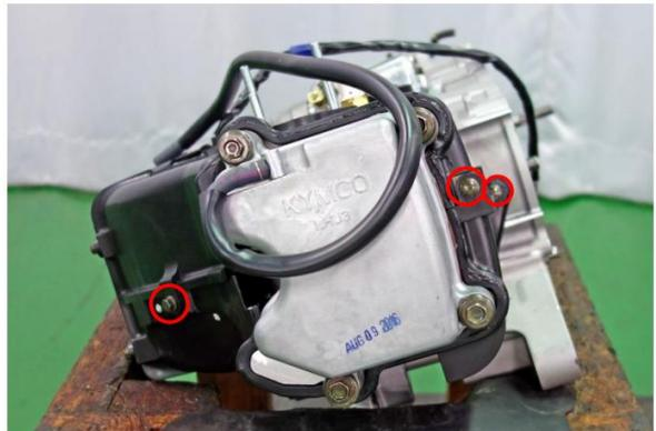
Remove 4 bolts and remove the cylinder head cover and gasket. Replace it with a new one when installation.
