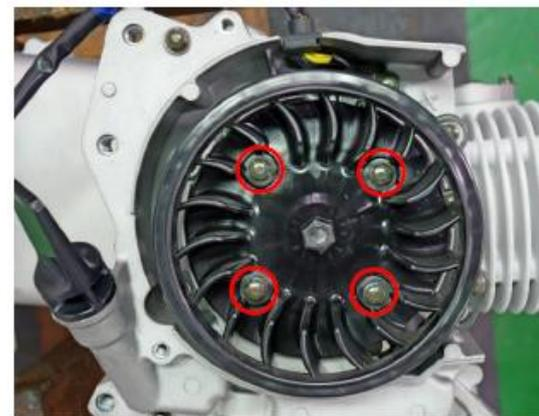
Install the lower cover first, then the upper cover, the fan cover is the last.
