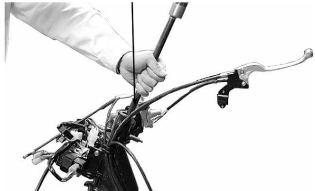
Drive new top and bottom ball races into the steering head using the outer driver.
