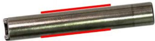
Inspect the rocker arm shaft inner diameter for the intake and exhaust valves.
