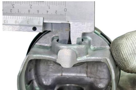
Measure the inner diameter of the small end of the connecting rod with vernier calipers.
