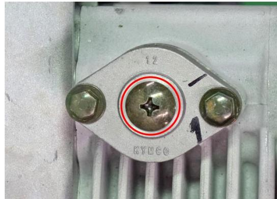
The cam chain tensioner is located on top of the cylinder.
