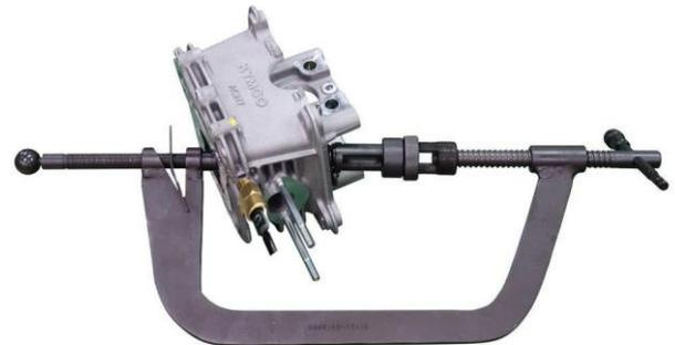
Push down the valve springs with a valve spring compressor.
