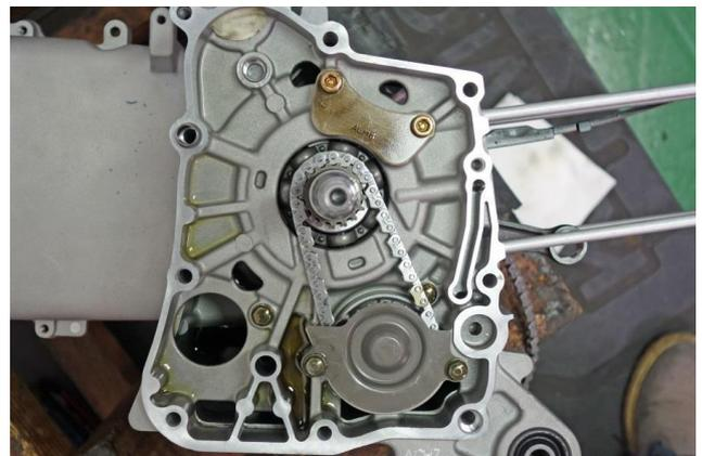
Loosen the two oil pump cover bolts with an 8mm socket.
