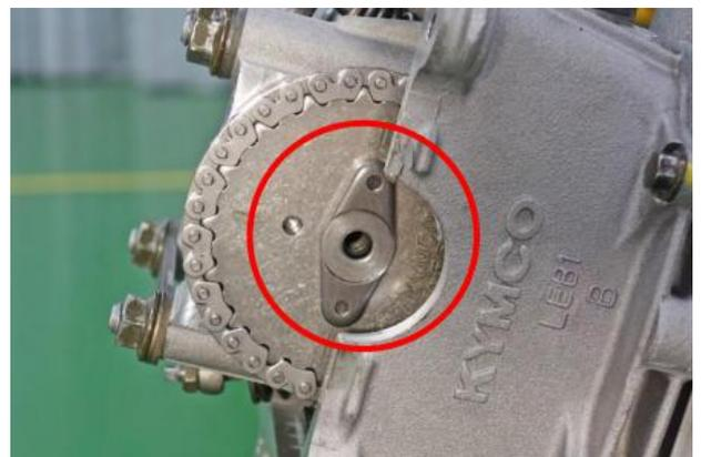
Remove the camshaft sprocket as shown,
