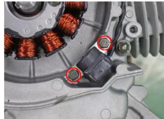
Install the 2 bolts and install the ACG cord clamer.
