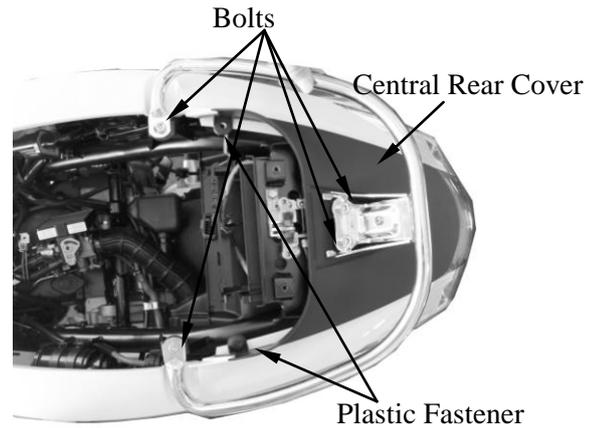
Remove 2 screws attaching the central cover
