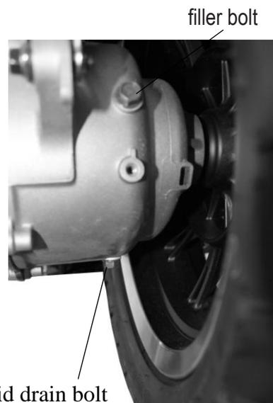
fluid drain bolt
