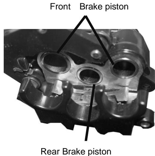
Check each piston for scratches or wear. Measure each piston O.D. with a micrometer gauge.
