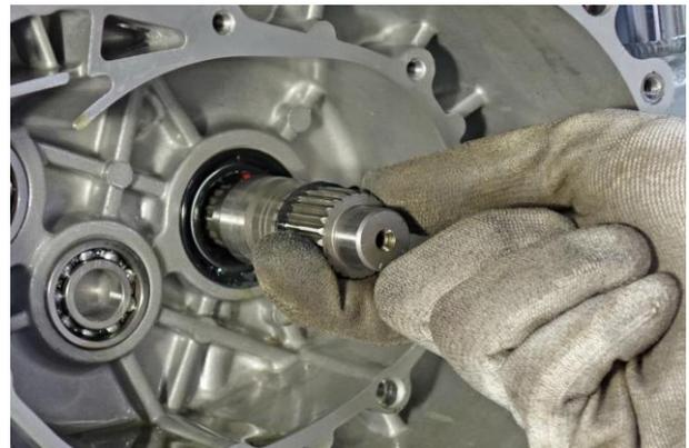
Insert the countershaft into its bearing as shown
