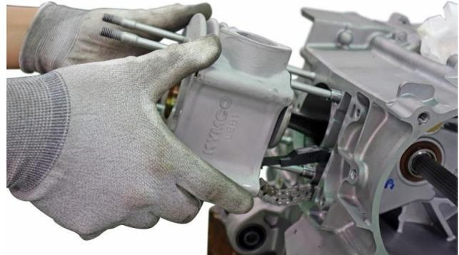
Insert the lower cam chain guide and make sure it is seated correctly.
