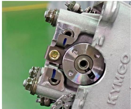
Install the camshaft sprocket onto the camshaft so the camshaft sprocket boss fits into the appropriate hole on the camshaft sprocket.
