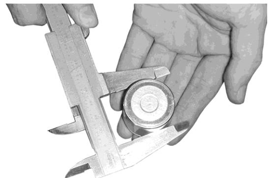
Check each caliper cylinder for scratches or wear and measure the cylinder bore.
