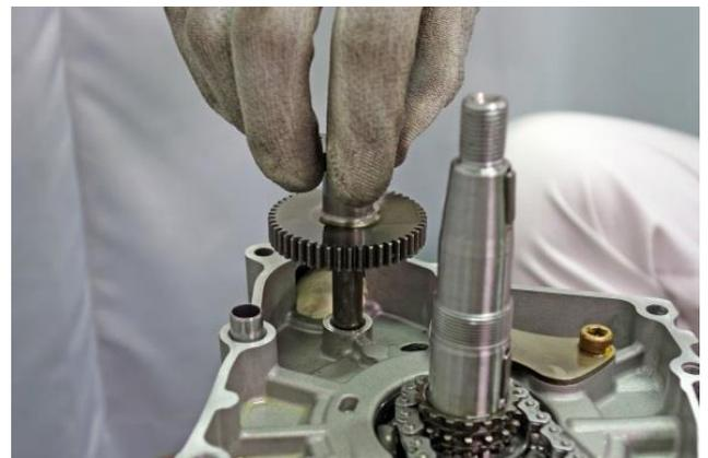
Put the bearing on the starter clutch.
