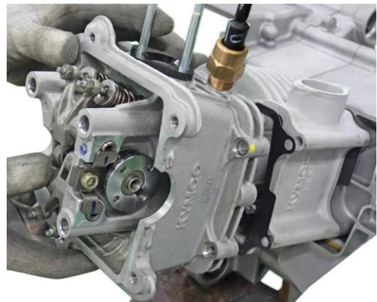
Lift the cylinder head off the stud,guide the cam chain through the opening in the cylinder head ,but don't allow the cam chain to fall into the crankcase.
