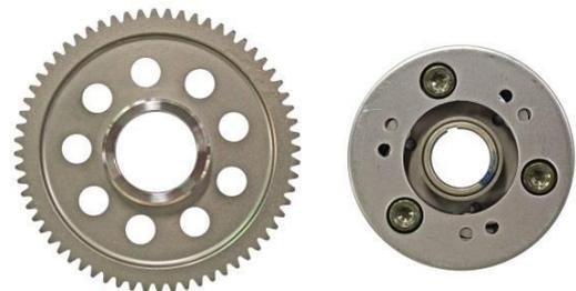
Fit the boss of the starter driven gear into the starter clutch. The Starter clutch should only allow the driven gear to turn in one direction. If the starter clutch allows turning both ways or will not let the driven gear rotate smoothly in one direction, the starter clutch must be replaced.
