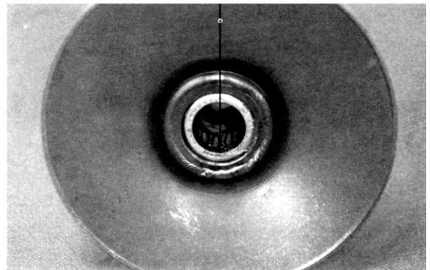
Remove the snap ring and drive the outer bearing out of the driven face.
