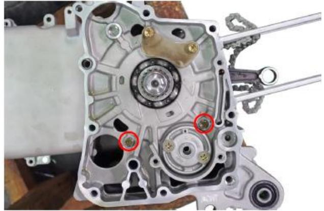
Lift the crankshaft out of the left crankcase half. Remove the cam chain from the crankshaft and crankcase. Inspect the cam chain for wear and damage. Replace the cam chain if needed.
