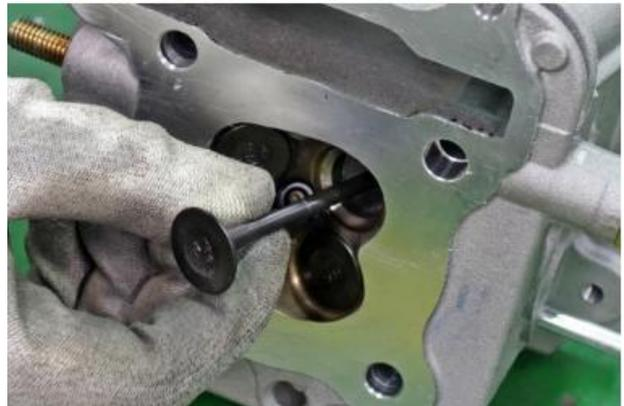
Remove the valve seal from the valve guide. The valve seal should be replaced if they are removed or you need to install new valves.
