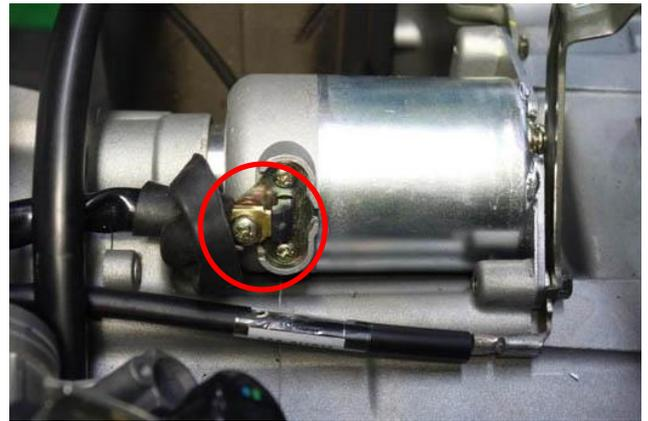
Remove the two starter motor mounting bolts with an 8mm socket.
