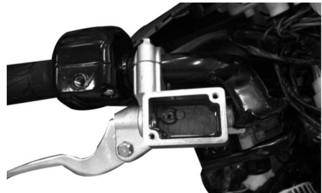
Fully apply the brake lever and then loosen the brake caliper bleed valve to drain the brake fluid until there is no air bubbles in the brake fluid. Then, tighten the bleed valve. Repeat these steps until the brake system is free of air.
