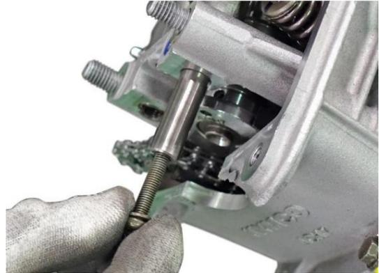
Lift the rocker arms as the shafts are removed.
