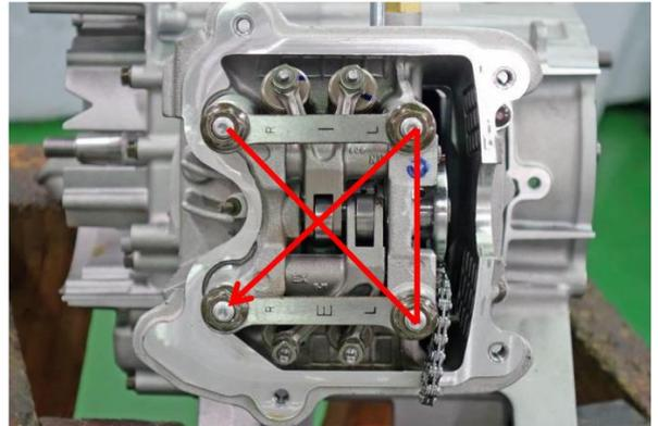
Install the set plate so it fits into the groove on the camshaft and between the projections on the rocker arm shafts.
