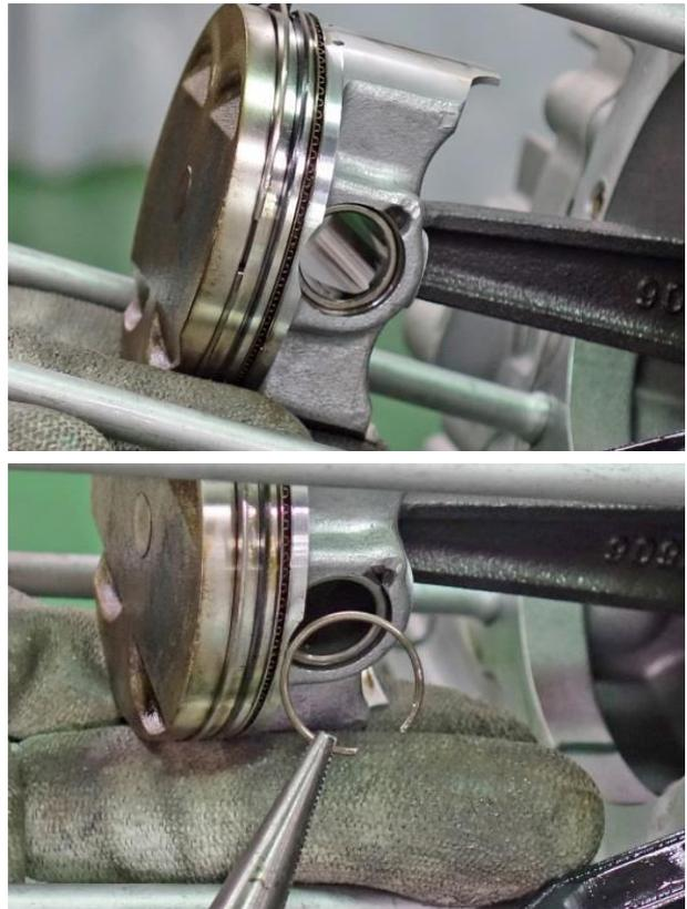
Remove the piston pin and the piston.
