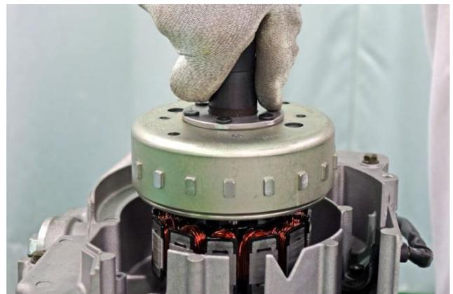
Remove the flywheel from the crankshaft.
