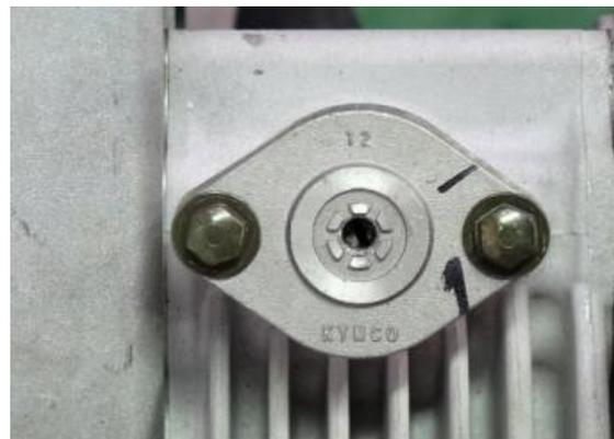
Remove the cam chain tensioner out of the cylinder.
