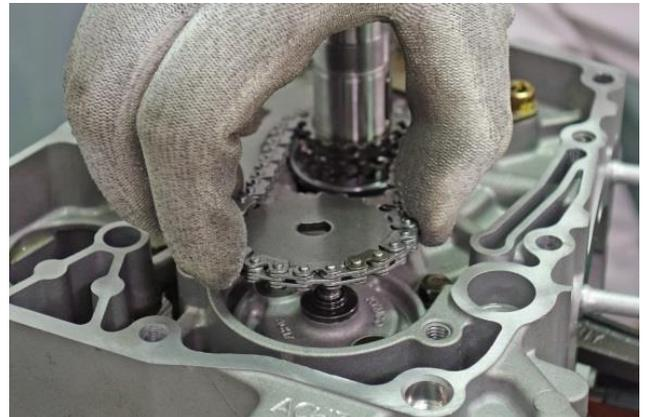
Remove the oil pump shaft.
