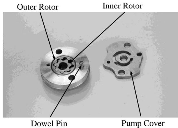
Tighten the screw to secure the pump cover. Make sure that the pump shaft rotates freely without binding.
