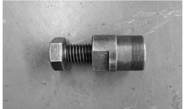
Apply grease to the threads of the flywheel puller tool before using it. Thread the puller onto the flywheel. Hold the tool with a large wrench and turn in the bolt until the pressure separates the flywheel from the crankshaft.
