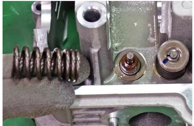
Push the valve stem down and remove the valve from the combustion chamber side of the cylinder head. Rotate the valve as it is removed
