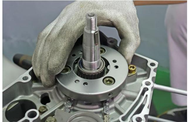
Take the bearing out of the starter clutch.
