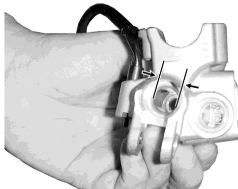
Measure the brake master cylinder piston O.D.
