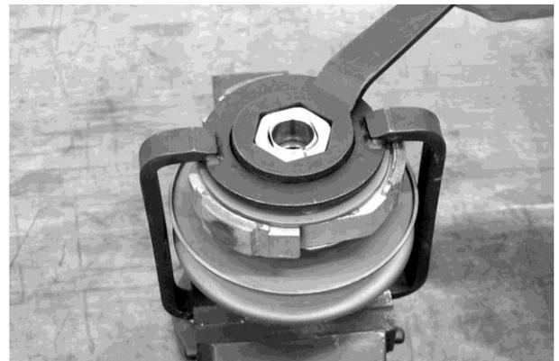
Loosen the clutch spring compressor and disassemble the clutch/driven pulley assembly.
