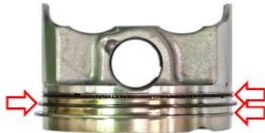
Install the top and second rings with their markings facing up. Install the rings to the piston as shown above so that no ring end gaps line up with the piston pin or perpendicular to the piston pin. The rings should turn easily on the piston without sticking or roughness.
