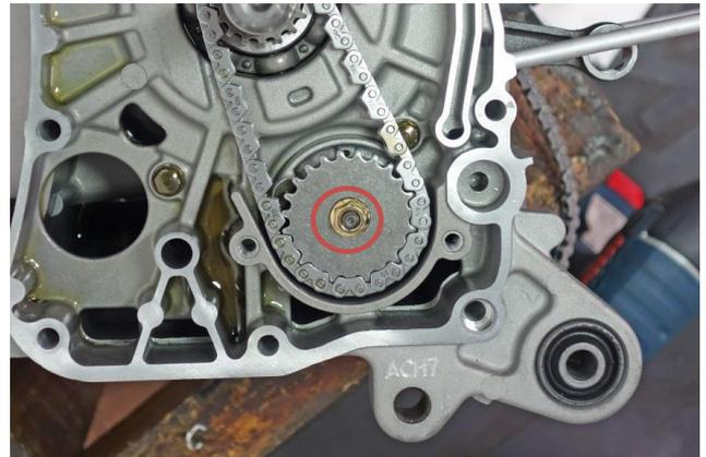
Remove the oil pump drive chain and driven sprocket.
