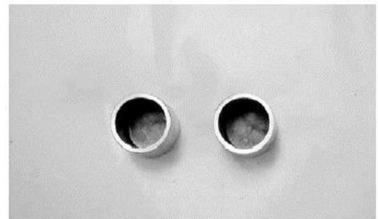
Check the caliper cylinder for scratches or wear and measure the cylinder bore.
