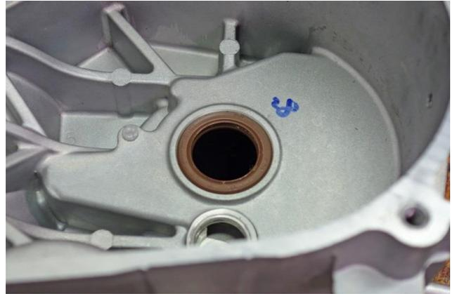
Remove the seal with a seal pick.
