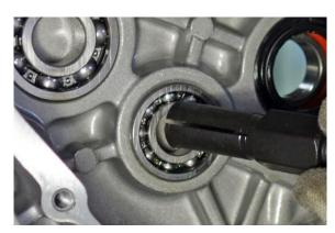
Use a bearing puller to remove the crankcase or transmission cover.
