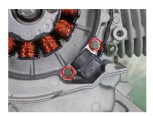
Install the 2 bolts and install the ACG cord clamper.
