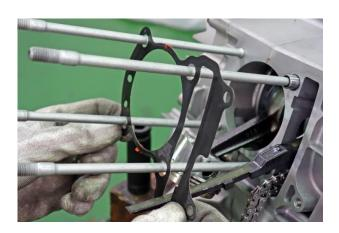
Remove the 2 cylinder dowel pins from the left side of the studs
