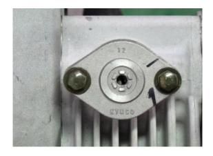
Remove the cam chain tensioner out of the cylinder.
