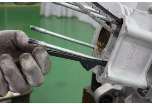
To remove the upper chain guide,remove the CVT ,see the CVT chapter.
