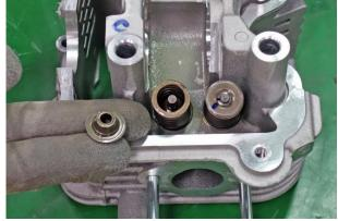
Remove the valve springs.
