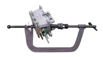
Special Tool: valve spring compressor, E040
