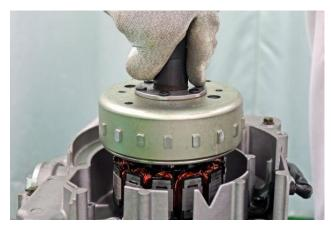
Remove the flywheel from the crankshaft.
