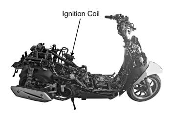
Measure the ignition coil resistances  $0.55 \sim 0.75 \,\Omega/20\,^{\circ}\text{C}$
