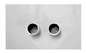
Check the caliper cylinder for scratches or wear and measure the cylinder bore.
