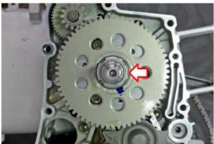
Remove the nut and washer, and then remove the starter clutch gear.
