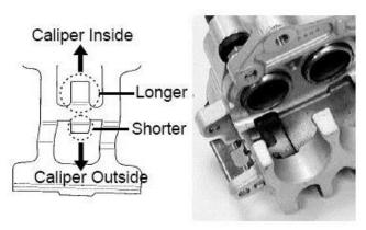
Install two brake pads and brake pad dowe pin.l
