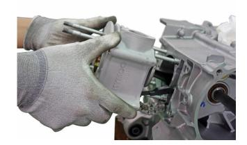
Insert the lower cam chain guide and make sure it is seated correctly.
