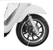
Remove the front axle nut and pull out the
