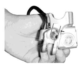
Measure the brake master cylinder piston O.D.
