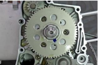
Install the right crank case cover, and then tighten the 10 bolts.
