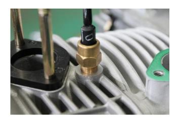
remove the engine temperature sensor if needed.
