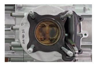
Remove the cylinder head gasket.
