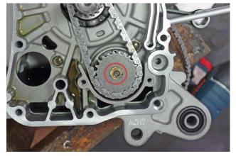
Remove the oil pump drive chain and driven sprocket.
