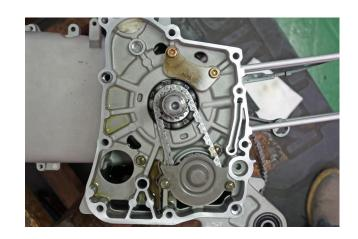
Loosen the two oil pump cover bolts with an 8mm socket.
