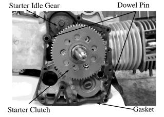
Install the right crankcase cover and tighten the nine bolts.
