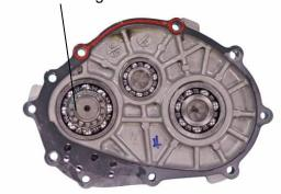
Check the transmission cover bearings for excessive play. Inspect the drive shaft, drive shaft bearing and oil seal for wear or damage.
