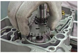
Remove the oil pump shaft.
