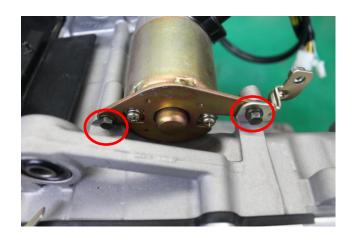
Inspect the starter motor O-ring and replace it as needed.
