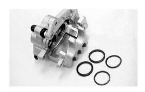
Check the piston for scratches or wear.
