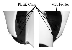
Remove 2 plastic fasteners beneath the handlebar cover.(turn the handlerbar to the left end and right end,you will see them)
