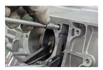
Install a new base gasket onto the crankcase.
