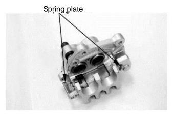
Make sure the spring plate next to the brake pad dowel pin orientation.
