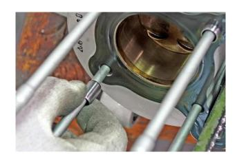
Remove the intake plate and gasket from the cylinder head.
