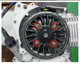
Remove the 17mm nut and washer.
