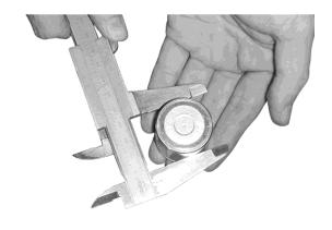
Check each caliper cylinder for scratches or wear and measure the cylinder bore.
