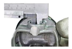
Measure the inner diamter of the small end of the connecting rod with vernier calipers.
