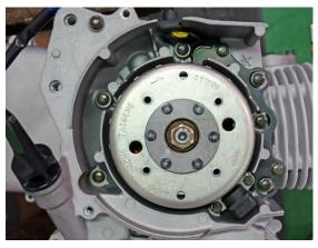
Install the fan, and tighten the 4 bolts.
