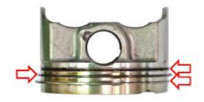
Install the top and second rings with their makings facing up.Install the rings to the piston as shown above so that no ring end gaps line up with the piston pin or perpendicular to the piston pin.The rings should turn easily on the piston without sticking or roughness.
