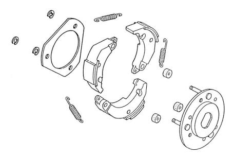
Install the damper rubbers on the drive plate pins.
