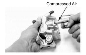
Push the piston oil seal outward to remove it. Clean the oil seal groove with brake fluid.
