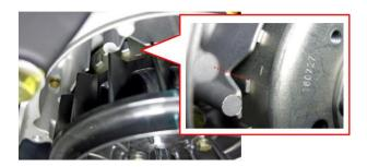
Apply a small amount of Loctite to threads of the camshaft sprocker bolts. Thread in the bolts and tighten to specification.
