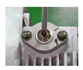
Install the fan cover and install the 4 bolts.
