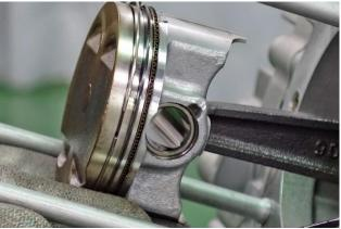
Make sure the cylinder head mating surface is clean. Install the two dowel pins as shown.
