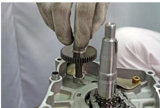
Put the bearing on the starter clutch. Install the starter clutch
