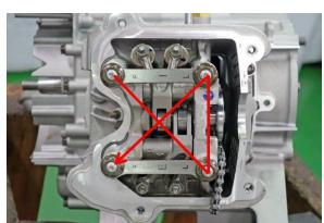
Remove the 2 camshaft holders.
