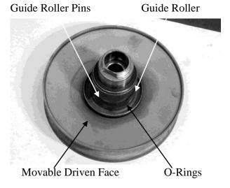
Remove the O-rings and oil seal from the movable driven face.
