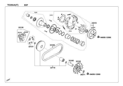
Install the weight rollers into the movable drive face.
