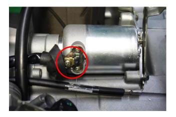
Remove the two starter motor mounting bolts with an 8mm socket.
