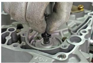
Remove the 2 oil pump screws with a #3 philips screwdriver.
