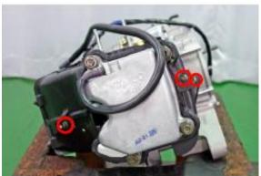
Remove the 4 bolts, and remove the fan.
