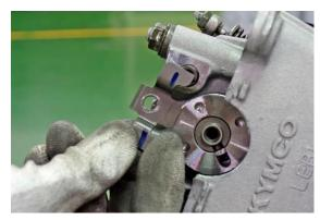
Remove the 4 camshaft holder nuts with a 14mm socket.
