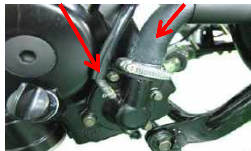
Air bleed hose
