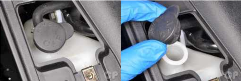
Open the coolant reserve tank lid.
