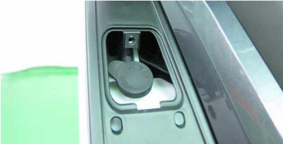
Install the coolant reserve tank lid.
