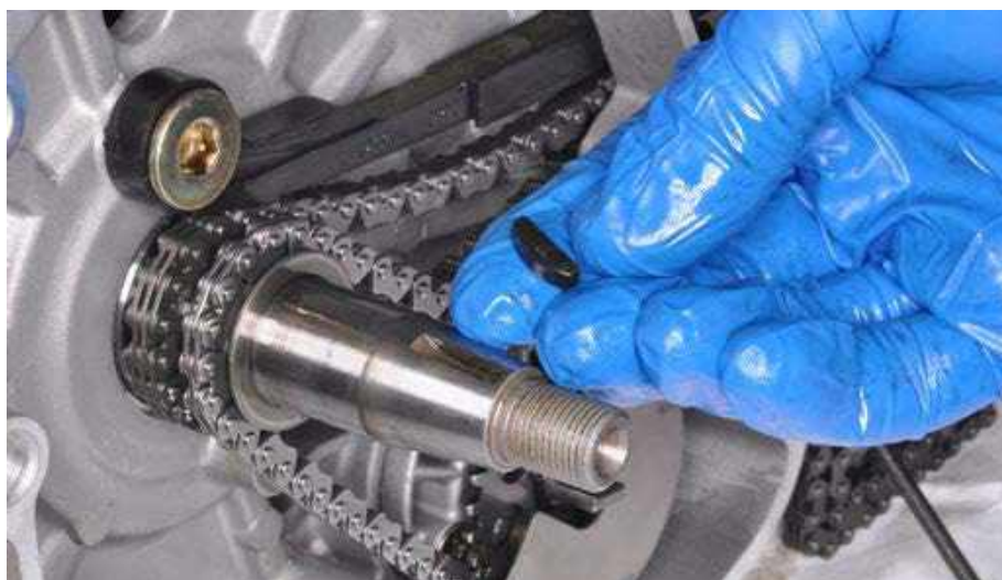
Remove the woodruff key from the crankshaft.
