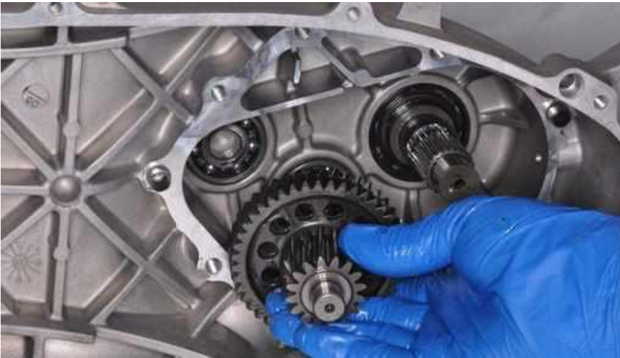
Remove the countershaft.
