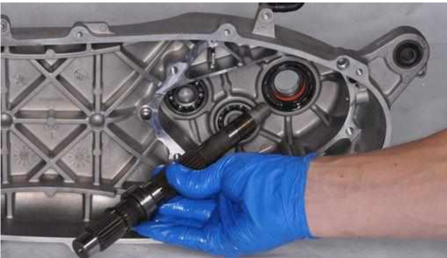
Remove the final shaft.
