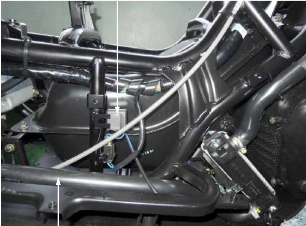
Coolant is from Radiator to Engine
