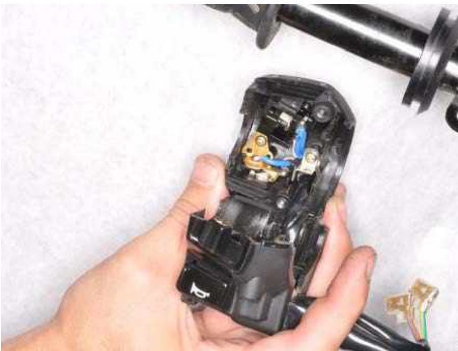
Disconnect the switch. Separate the left switch housing from the handlebar.
