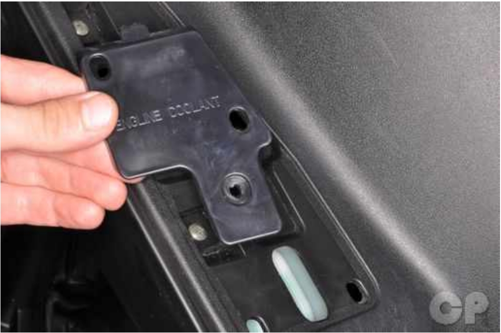
Remove the engine coolant reserve tank cover.
