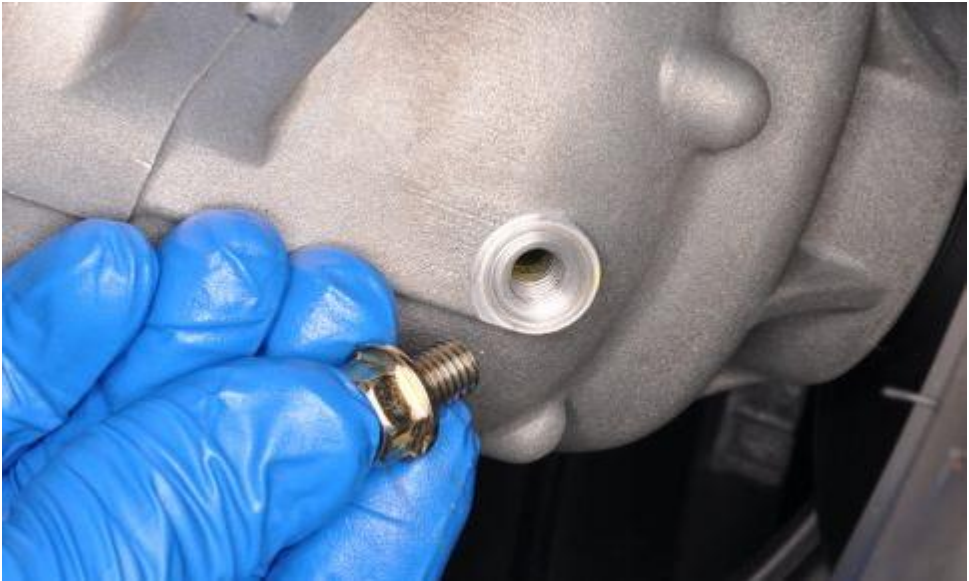
Thread in the final drive oil level filler bolt.
