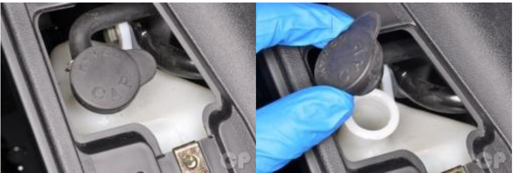
Open the coolant reserve tank lid.
