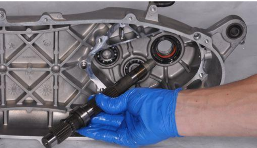
Remove the final shaft.
