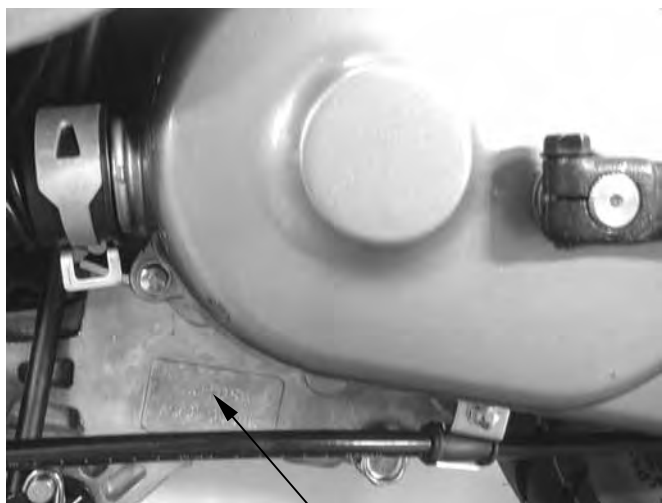
Location of Engine Serial Number
