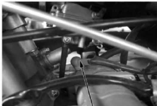
Positive Wire, Starting Motor
