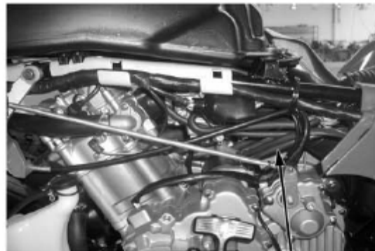
Negative Wire, Starting Motor
