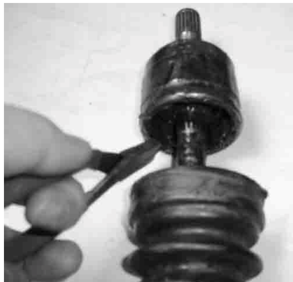
Remove the stopper ring
