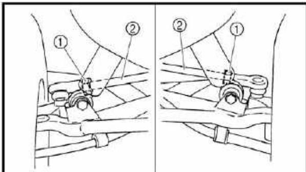
*make , sure if the Steering bar is pormal , if not , adjust the tension rod left or right within the specification .*
