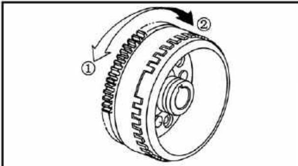
b. Turn the starter wheel gear counterclockwise ① to check that the starter clutch and wheel gear engage.
