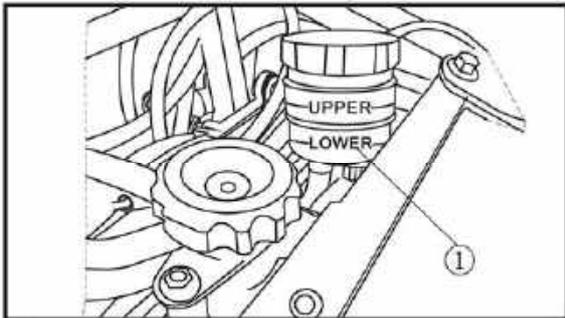
①. To check the amount of liquid in the oil cup. If it is lower than the minimum mark, refill the box with the same type of fluid as was recommended by the manufacturer, to ensure to fluid level is higher than the minimum mark.
