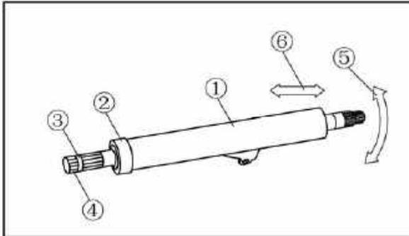
The central axis of the steering shaft whether flexible and moves. If does, dismantle and check the axis, bearing and retaining ring whether ware or damaged, according to the inspection situation to instead the parts.
