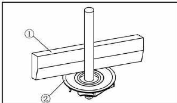
**Max. impeller shaft tilt
