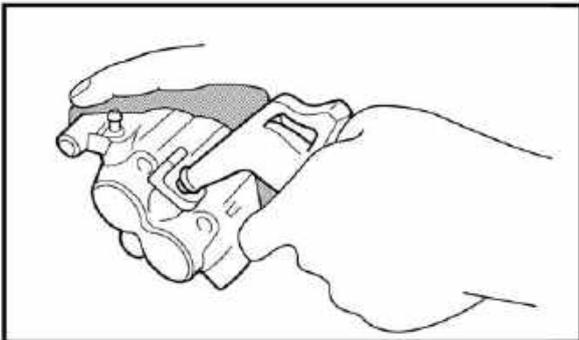
b. Remove the dust seals and caliper piston seals.
