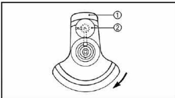
The crankshaft ① and the crank pin ② oil passages must be properly interconnected with a tolerance of less than 1 mm (0.04 in).
