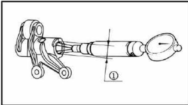
**Rocker arm inside diameter repairing limit value**
