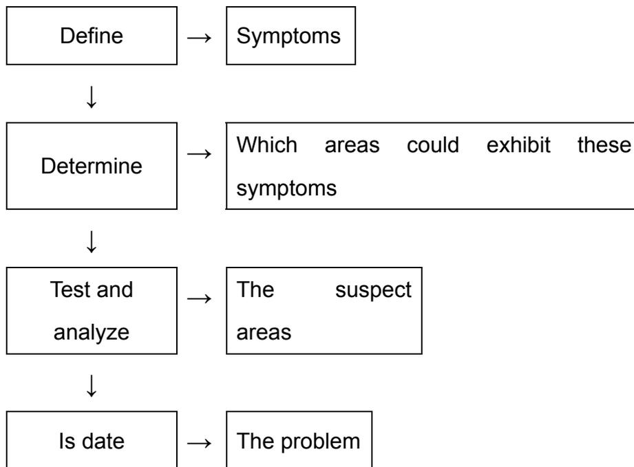
By following a systematic approach, the possibility of unnecessary parts replacement can be avoided, always start with the simple and most obvious checks when troubleshooting, This would include the engine stop switch, fuel quantity and condition, fuel vale position and spark plug cap tightness
