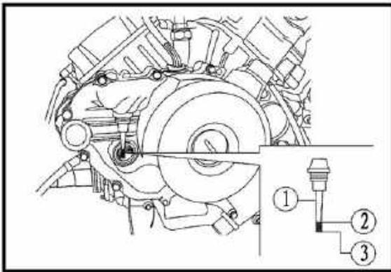
**CHECKING THE ENGINE OIL LEVEL**
