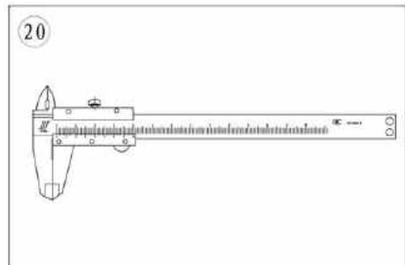
Calipers are available in dial, vernier or digital versions. Dial calipers have a dial readout that provides convenient reading. Vernier calipers have marked scales that must be compared to determine the measurement. The digital caliper uses a liquid-crystal display (LCD) to show the measurement.
