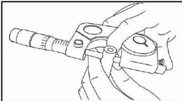
**Rocker arm shaft outside diameter repairing limit value**
