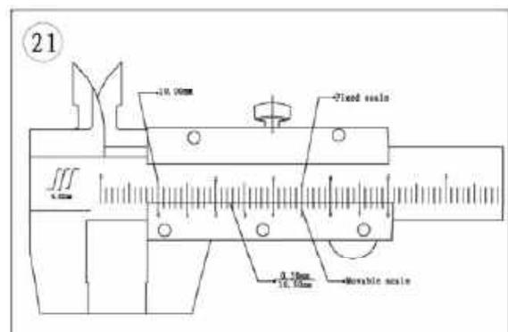
A number of lines will seem close, but only one will align exactly. In this case, 0.50 mm is the reading to add to the first number. Adding 10 mm and 0.50 mm equals a measurement of 10.50 mm.
